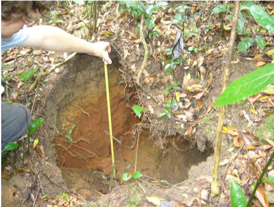
Plate 27 - Collapse Feature Upslope of Main Scarp of the Distressed Hillside (Photograph taken on 22 March 2006)
