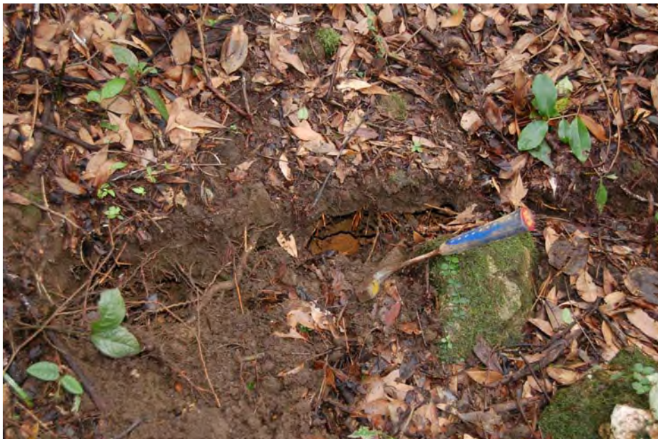
Plate 26 - Discontinuous Tension Crack above Drillhole No. BH4 near the Western Flank of the Distressed Hillside (Photograph taken on 10 July 2006)
