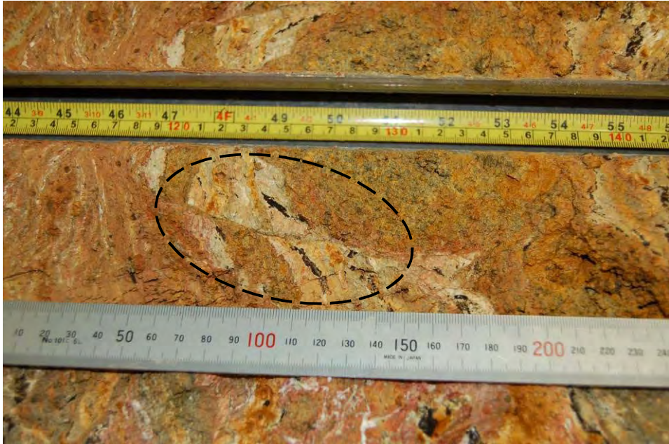
(a) Offset observed at about 9 m Depth in drillhole No. BH4
