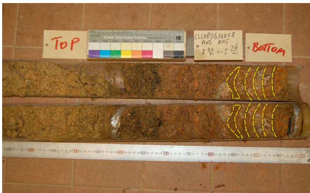
Plate 42 - Clay Bands at 5.7 m Depth in Drillhole No. BH5
