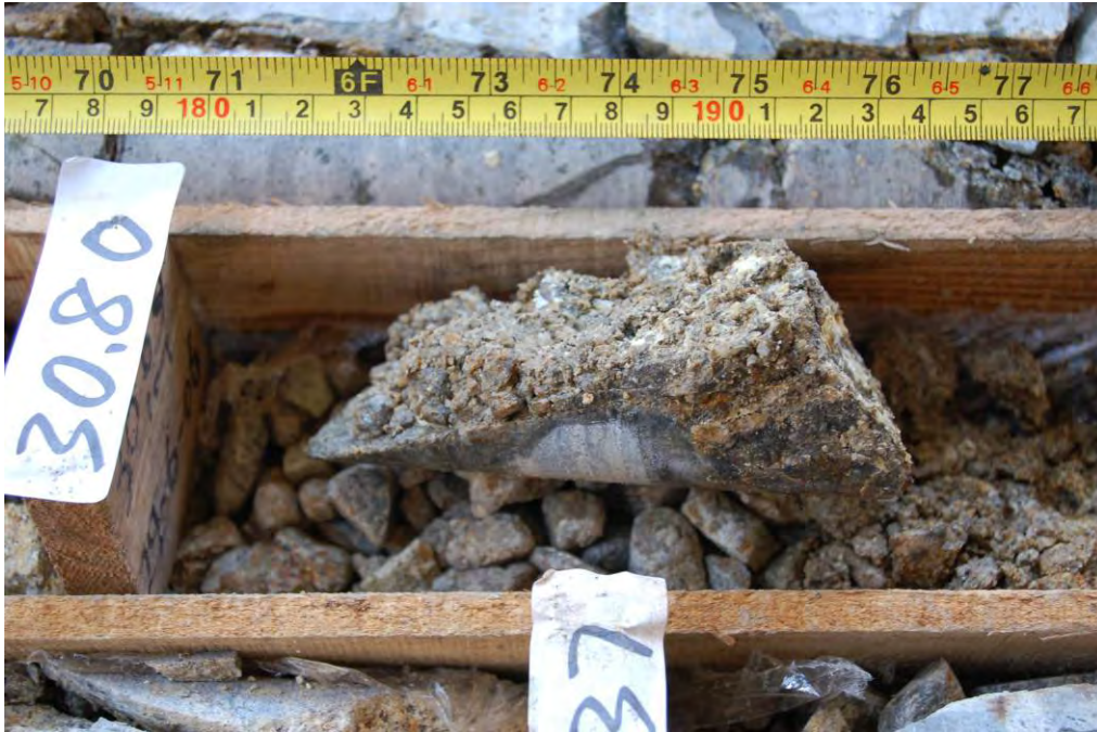
Plate 37 - Fault Gouge along Joint at 30.8 m Depth in Drillhole No. BH2
