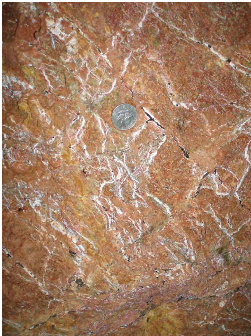
Plate 35 - Boxwork Kaolin Veins in CDT in Trial Pit No. TP8
