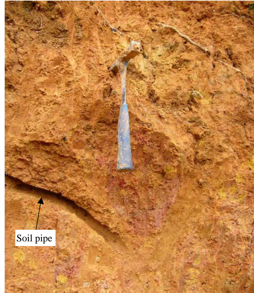
Plate 8 - Old Colluvium Exposed in the Western Flank of the August 2005 Landslide (Photograph taken on 14 March 2006)
