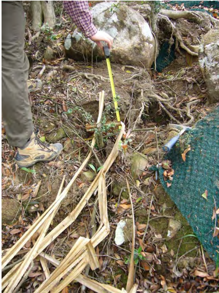
Plate 9 - Lateral Tension Crack Immediately West of the August 2005 Landslide (Photograph taken on 10 March 2006)
