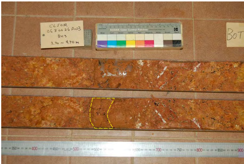
Plate 39 - Clay Bands at 4.2 m Depth in Drillhole No. BH3
