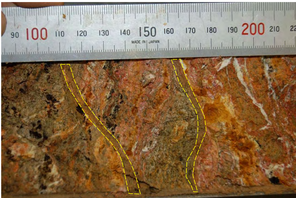
Plate 40 - Clay Bands at 4.2 m Depth in Drillhole No. BH4
