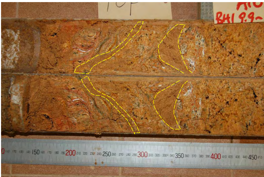
Plate 38 - Clay Bands at 10 m Depth in Drillhole No. BH1
