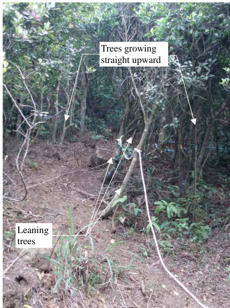
Plate 29 - Leaning Trees near the Eastern Flank of the Distressed Hillside (Photograph taken on 28 April 2006)
