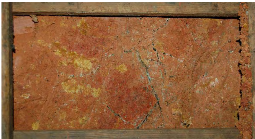
Plate 34 - Old Colluvium Observed in Split Mazier Samples and Trial Pit
