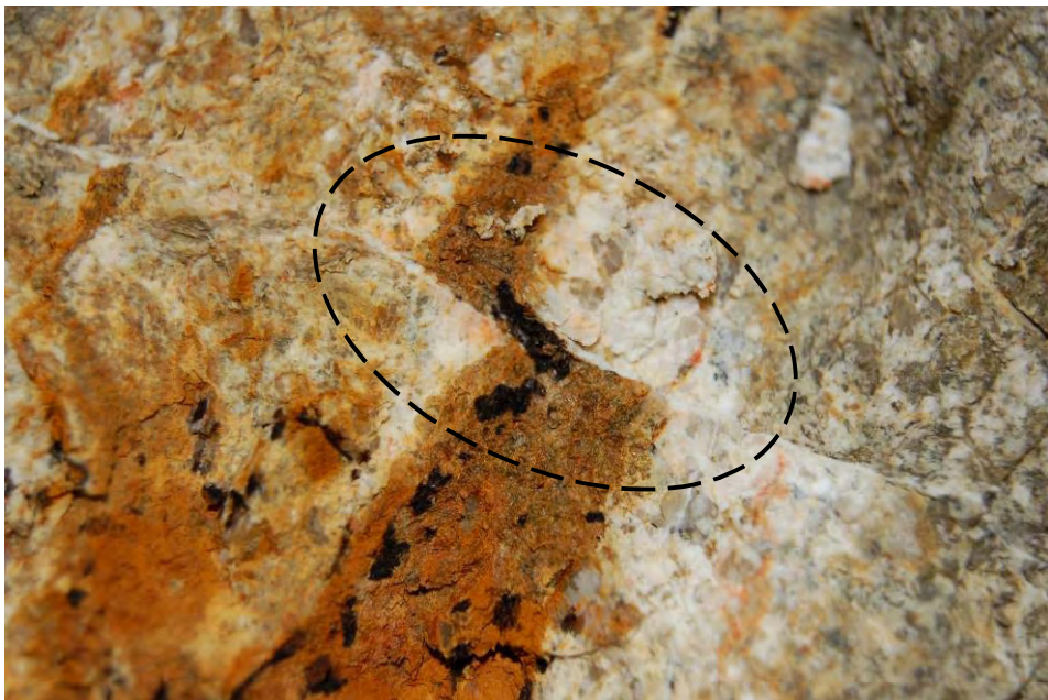
(b) Offset observed at about 25 m Depth in drillhole No. BH5
