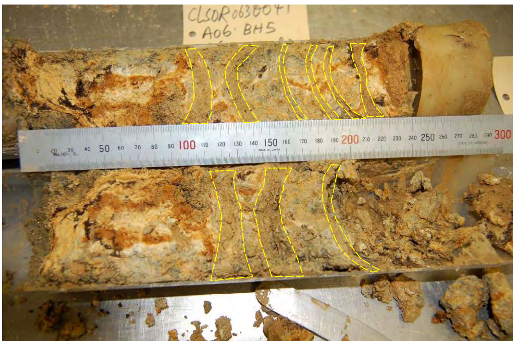
Plate 44 - Clay Bands at 18.7 m Depth in Drillhole No. BH5
