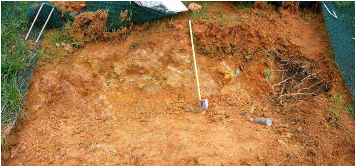
Plate 11 - Completely Decomposed Tuff with Kaolin Veins Exposed in the Base of the August 2005 Landslide (Photograph taken on 14 March 2006)
