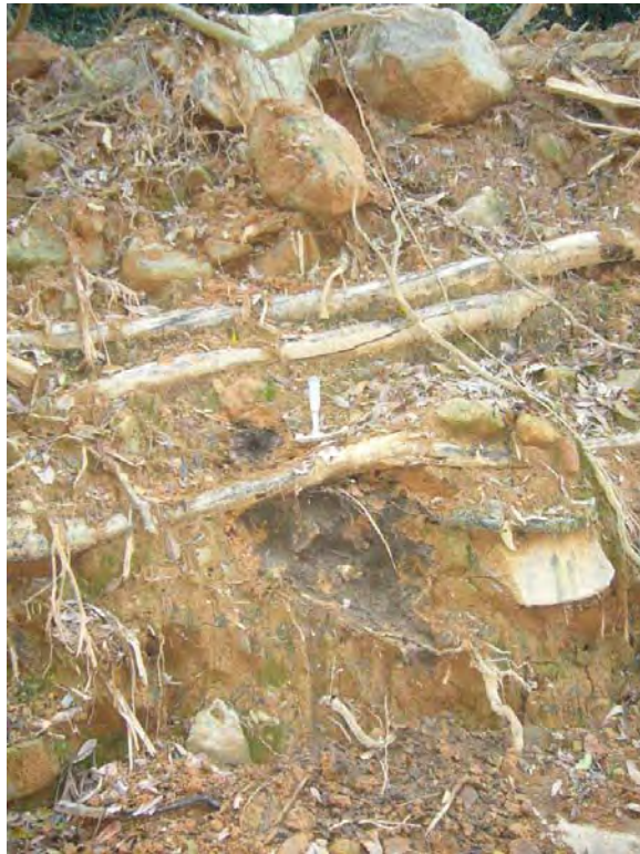
Plate 19 - Trees and Soil Adjacent to the Debris Trail Buried by Previous Landsliding (Photograph taken on 10 March 2006)
