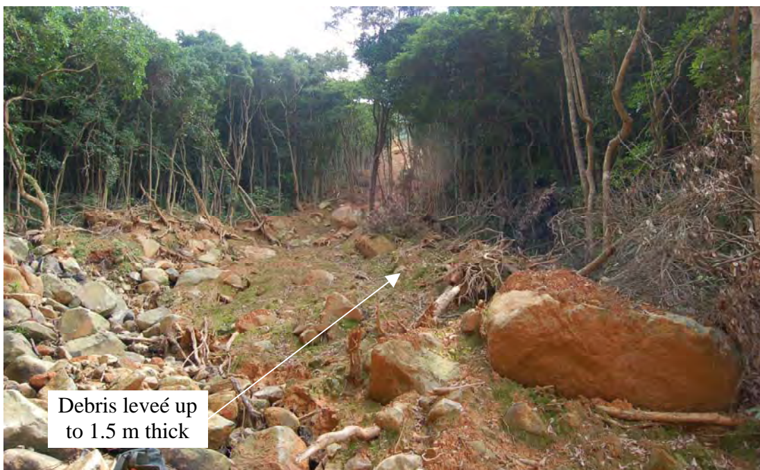
Plate 18 - Debris Trail at Chainage CH220 Showing Deposition of Debris on the Inside Bend (Photograph taken on 25 May 2006)
