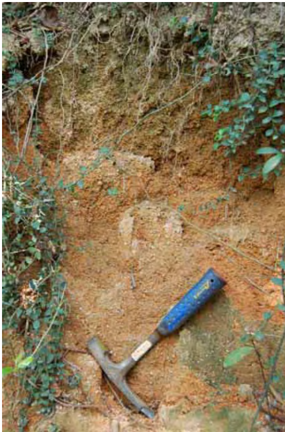
Plate 14 - Colluvium Overlying Residual Soil (Photograph taken on 27 April 2007)
