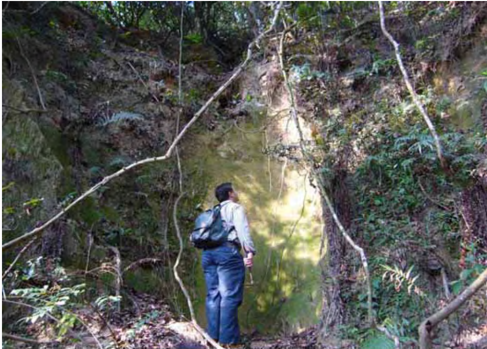
Plate 11 - Sub-vertical Steeply Dipping, Southwest-facing Joint Surfaces at Backscarp of Older Landslide Scar (Photograph taken on 13 April 2007)
