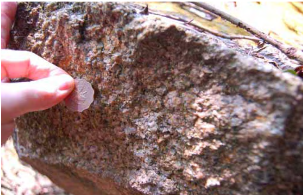
Plate 12 - Exposure of Pale Pink Kowloon Granite at Cut Slopes Nos. 11NW-B/C519 and 11NW-B/C250 (Photograph taken on 27 April 2007)
