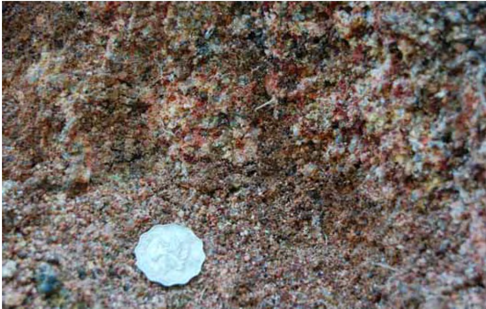
Plate 13 - Exposure of Completely Decomposed Coarse-grained Shatin Granite at Slope No. 11NW-B/C521 (Photograph taken on 27 April 2007)
