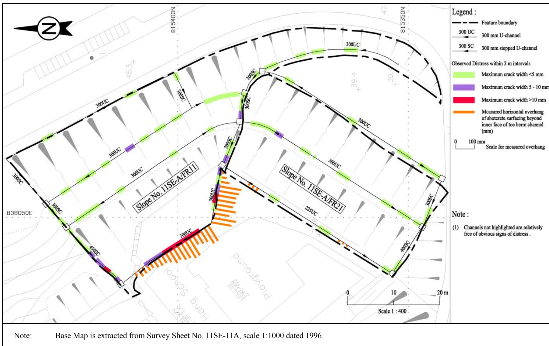
Figure 4b - Distress of Slope No. 11SE-A/FR11 at Lai Tak Tsuen Road
