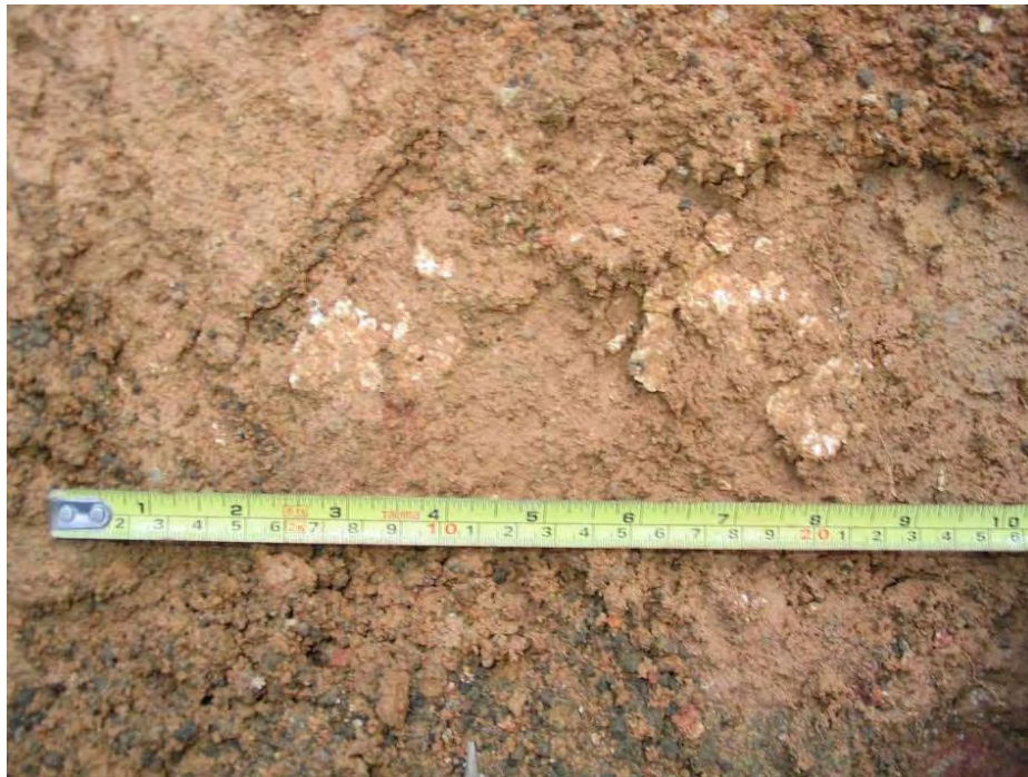
Plate 11 - Localised Kaolin Deposits on the Failure Surface (Photograph taken on 23 August 2005)
