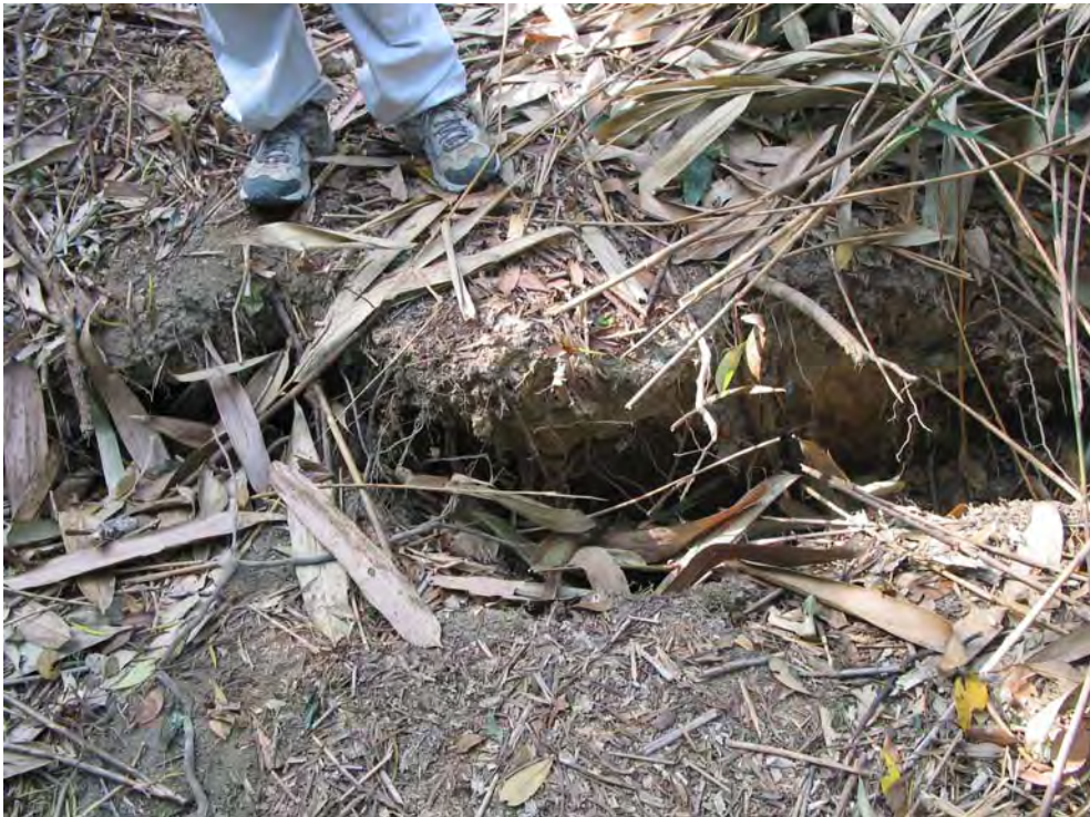
Plate 21 - Tension Crack within the Distressed Hillside (Photograph taken on 2 December 2005)
