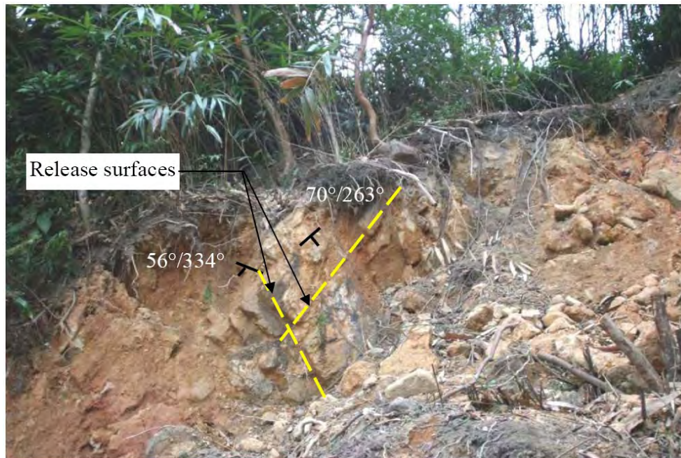
Plate 13 - Release and Unfavourable Joints on Eastern Flank of the Landslide (Photograph taken on 2 December 2005)
