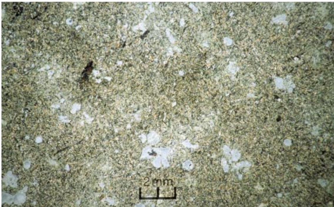
Plate 7 - Thin Section of a Mafic Dyke from Hau Hok Wan (HK9237, 1156 1727)
