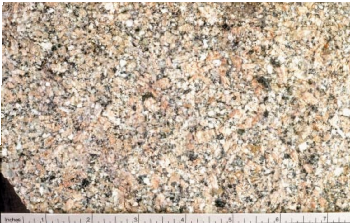
Plate 6 - Fine-grained, Porphyritic Tong Fuk Quartz Monzonite from Sha Lo Wan (HK10067, 0812 1633)
