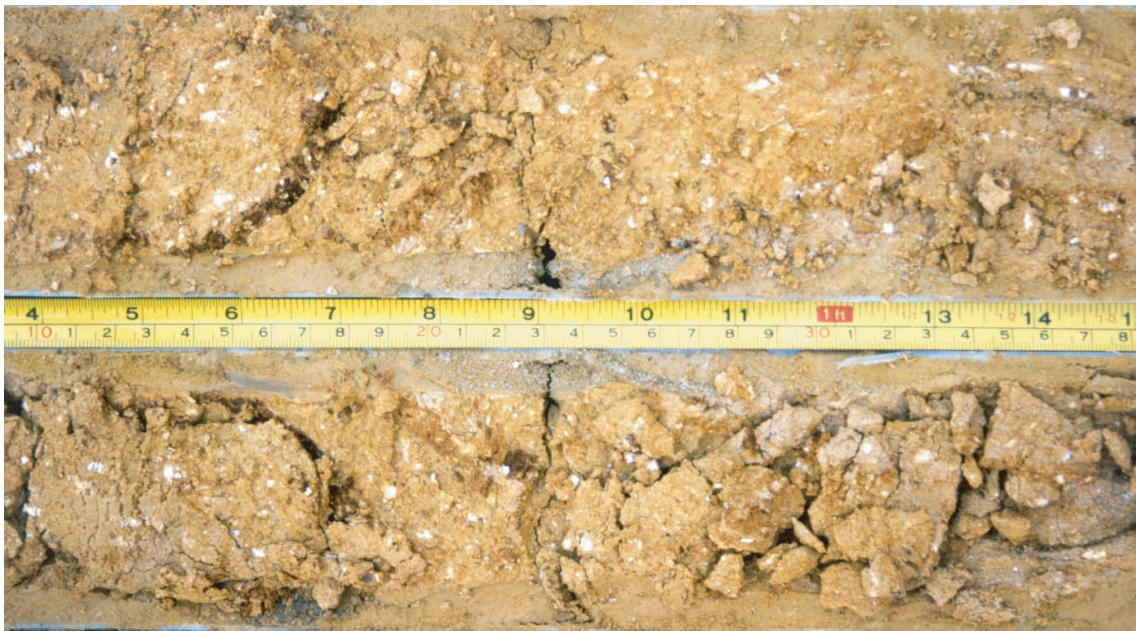
Plate A22b - Residual soil derived from (?) coarsely feldsparphyric rhyolite. Relict feldspar (white areas) and fresh quartz phenocrysts can be discerned in the orange-brown clayey matrix. Way-up to the right. Tung Chung, Site 4; Drillcore A-8B, Mazier sample, 76 - 77 m
