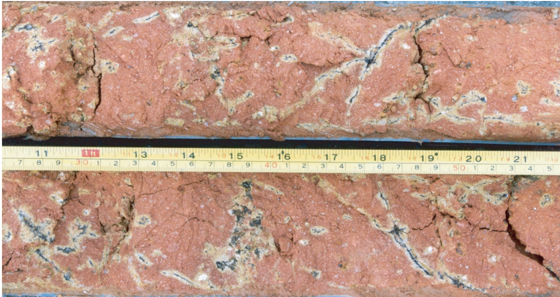
Plate A22a - Residual soil derived from finely feldsparphyric rhyolite. Relict feldspar and fresh quartz phenocrysts can be discerned in the reddish clayey matrix. The black and orange colouration is secondary Mn and Fe oxide minerals which developed originally in and around hairline fractures. Way-up is to the right. Tung Chung, Site 4; Drillcore A-48, Mazier sample, 64 - 65 m
