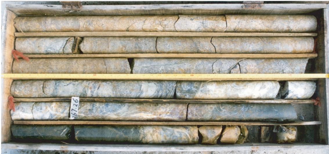
Plate A13b - Contact facies granite and skarn. This is typical of granite-metasedimentary rock contacts in Site 3 drillcores : the granite, whose textural and mineralogical characteristics are clearly modified with respect to 'normal' granite encountered in Tung Chung drillcores, has a sharp, unfaulted contact (at the left side of the fourth drillcore stick in this view) with skarn. Tung Chung, Site 3; Drillcore CC-20; Box 7, 163.22 - 168.71 m
