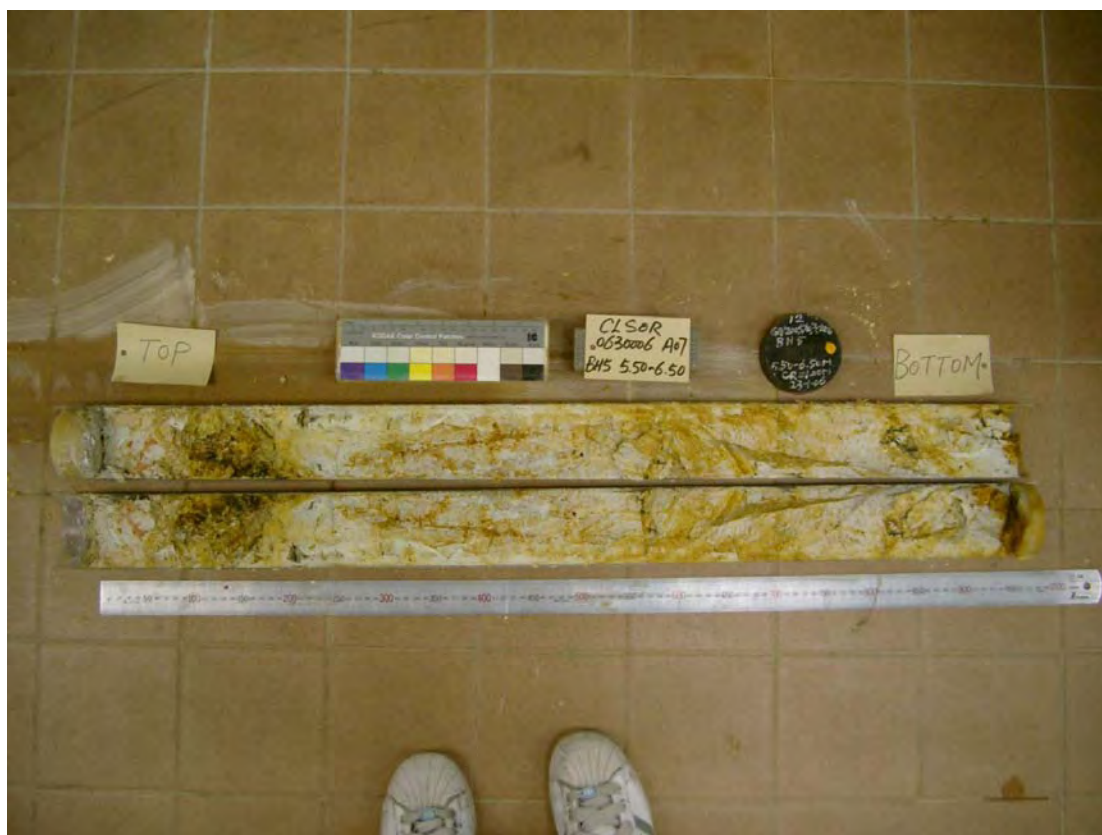
Plate 33 - Kaolinised Tuff in Mazier Sample Recovered from Drillhole BH5 (Photograph taken on 26 April 2006)
