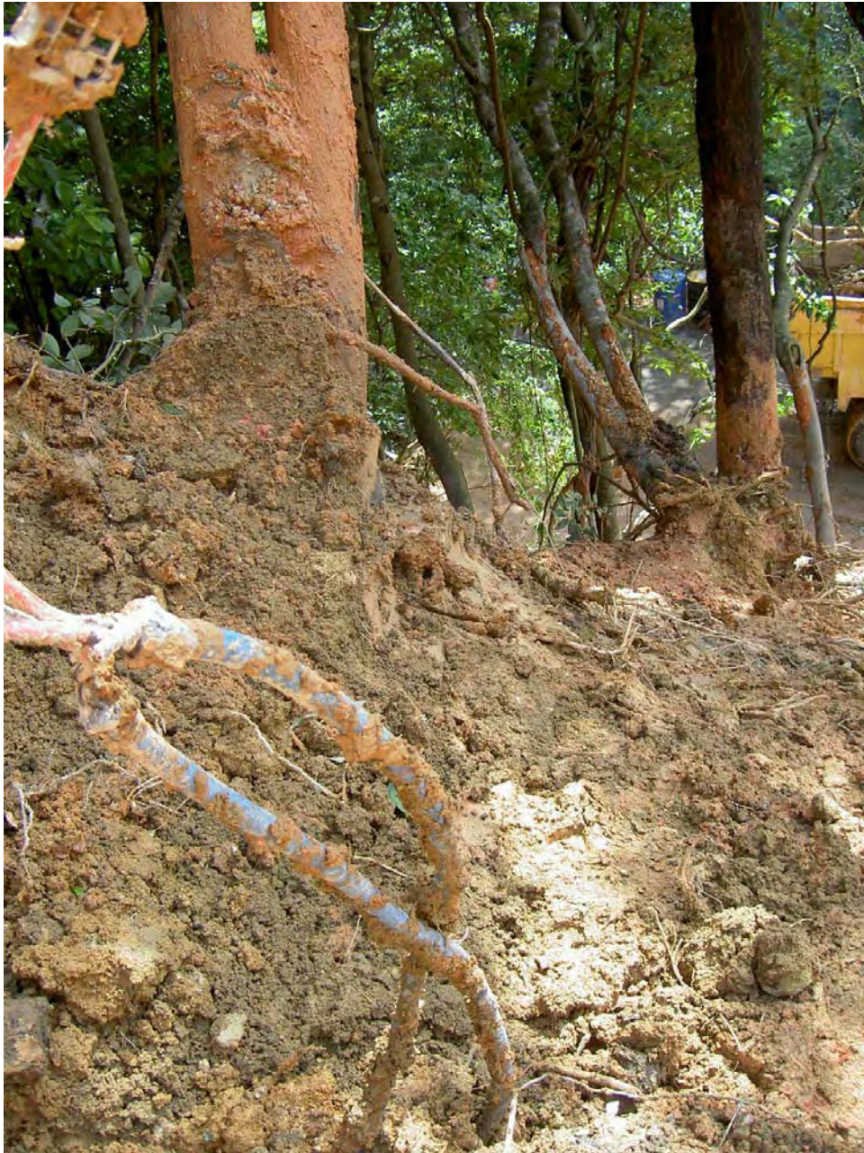
Plate 24 - View East from Mount Cameron Road Showing Scarring on Trees Providing Indication of Thickness of Debris Mass During the Landslide
