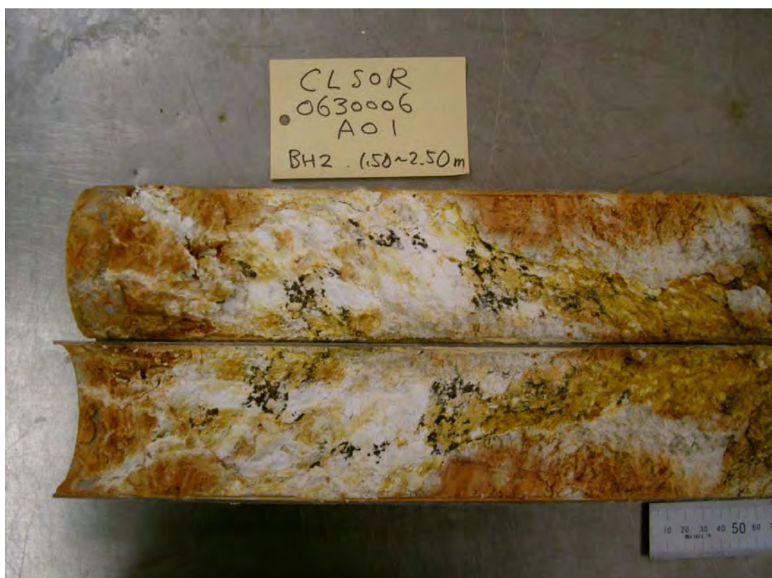
Plate 34 - Deposition of White and Buff Kaolin and Black Manganiferous Infills in Relict Joints (Photograph taken on 26 April 2006)
