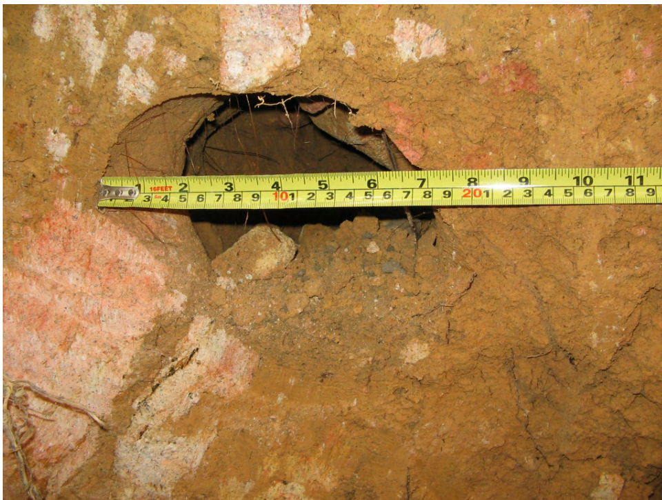
Plate 28 - Soil Pipes within Colluvium in Trial Pit TP1 (Photograph taken on 9 February 2006)
