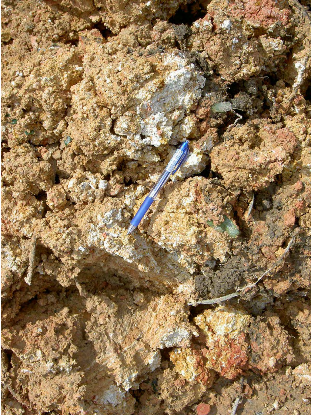
Plate 23 - Example of Kaolin-like Material Identified in Landslide Debris
