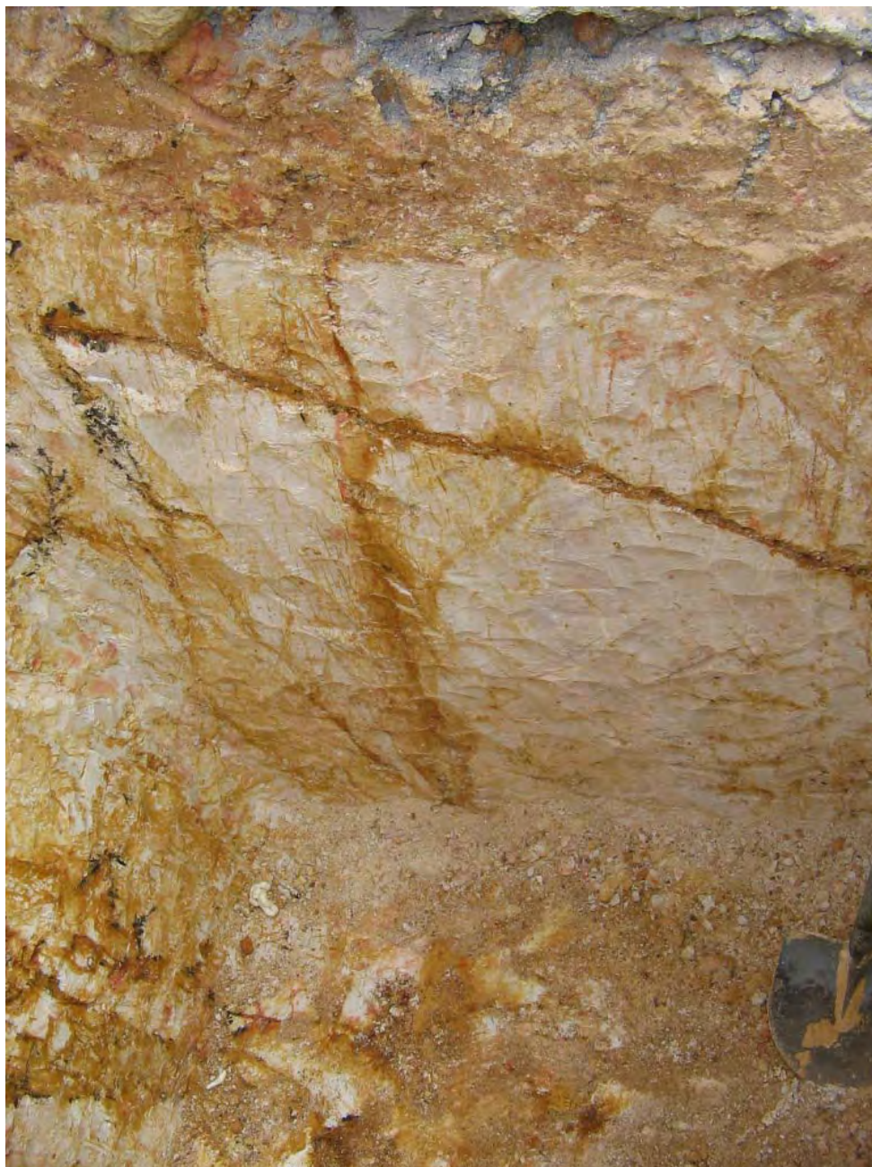
Plate 31 - Extensive Kaolinisation of Decomposed Tuff in Trial Pit TP5 (Photograph taken on 13 February 2006)
