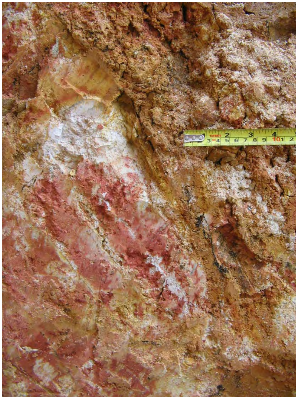
Plate 32 - Kaolin in Relict Joint in Trial Pit TP4 (Photograph taken on 11 February 2006)
