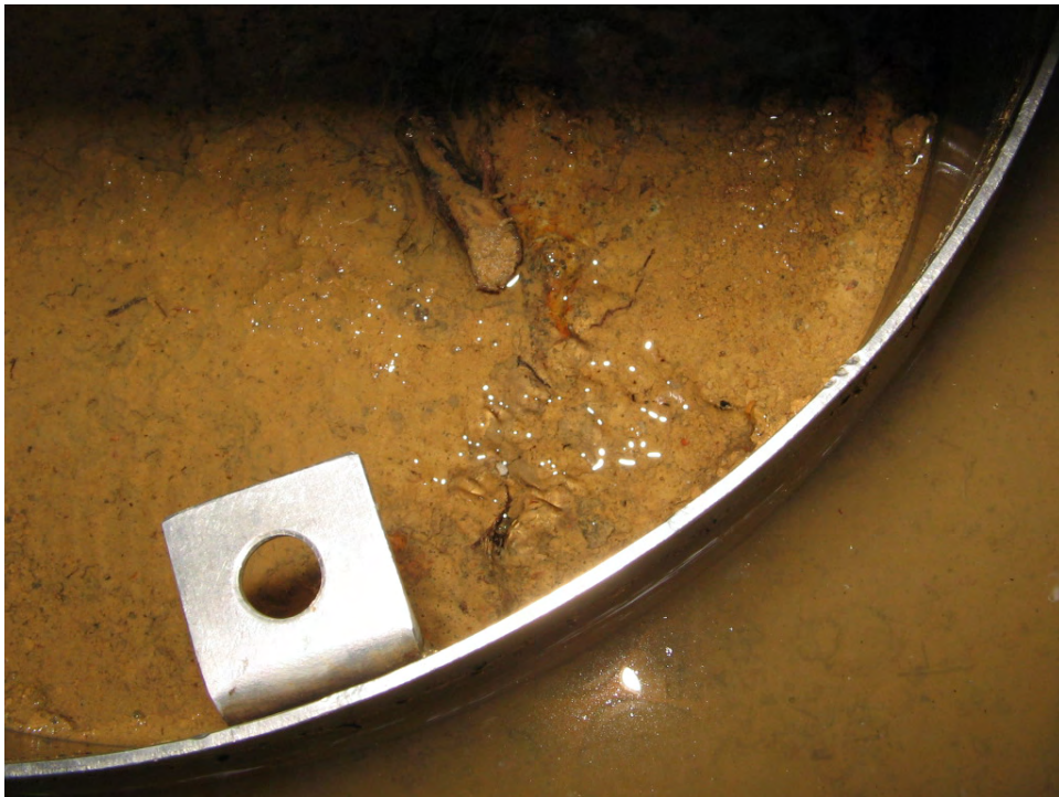
Plate 29 - Presence of Soil Pipe Caused Sudden Loss of Water Placed within Inner Ring During Double Ring Infiltrometer Testing in Trial Pit TP1 (Photograph taken on 7 February 2006)
