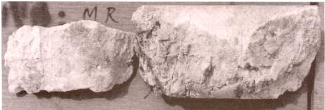
Plate 16 - Karst Features in Borehole Cores: Solution Widened Joint Showing Fretted Surface
