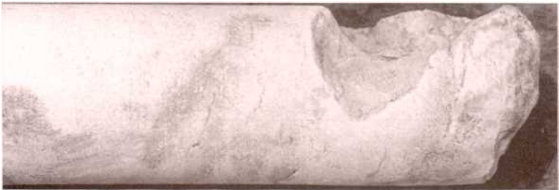
Plate 15 - Karst Features in Borehole Cores: Solution Feature Showing Ferruginous Staining
