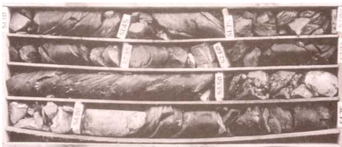
Plate 10 - Graphite Schist of the Mai Po Member, Lok Ma Chau Formation, with Prominent White Quartz Veins; BGS27, 51.10-54.75 m
