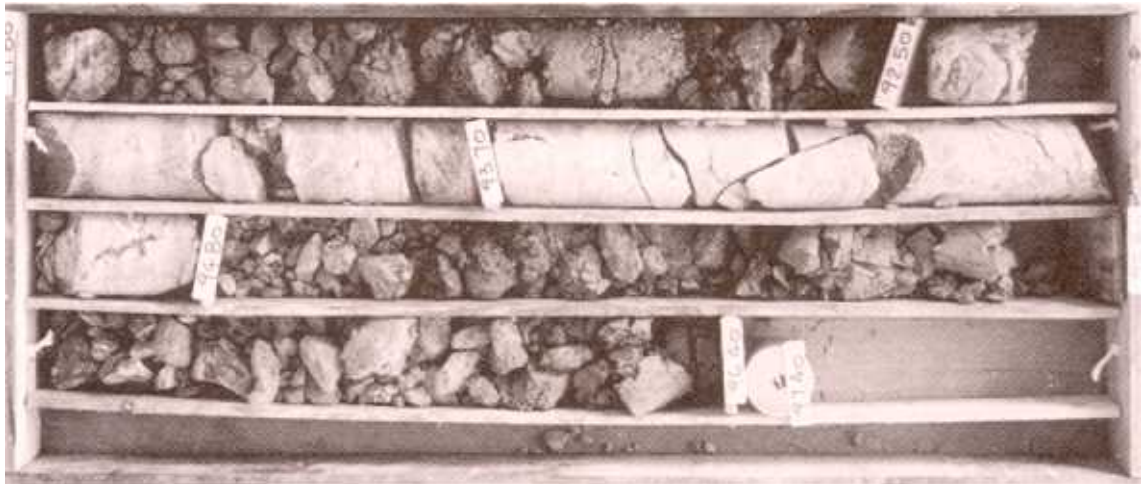
Plate 11 - Highly to Completely Weathered Tuffaceous Siltstone with Clasts of Marble, Tin Shui Wai Member, Tuen Mun Formation; BGS8, 91.80-97.40 m
