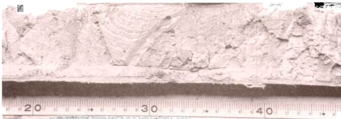
Plate 5 - Highly to Completely Weathered Metasilstone of the Mai Po Member Showing Liesgang Rings in Ferruginous Concretions; BGS17, 52.90-53.90 m
