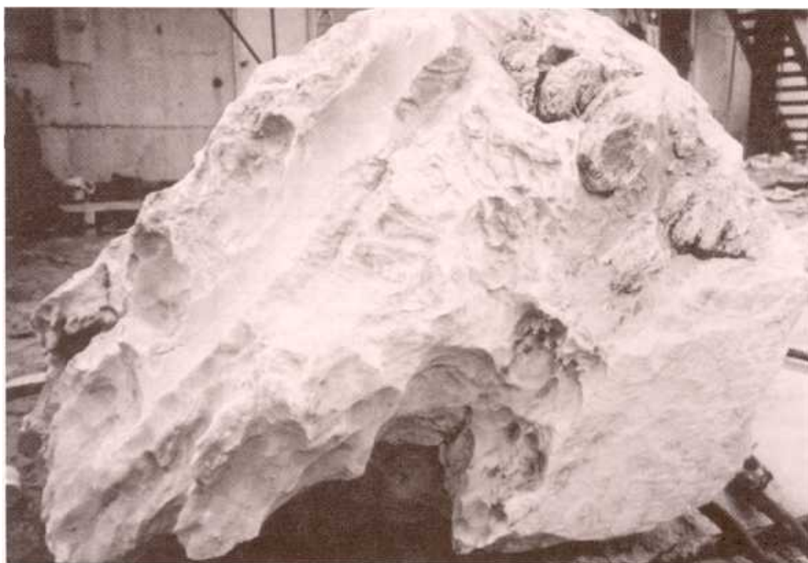
Plate 3 - Large Block of Karst Marble (inverted Ma Tin Member) Excavated from the Rockhead at the LRT Site, Yuen Long
