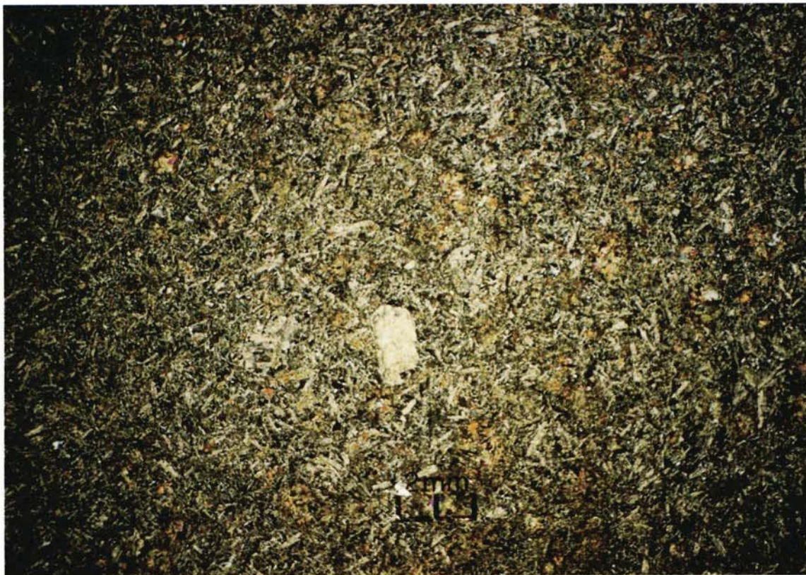
Plate 36 - Thin Section of Very Fine-grained Basalt (HK10684) (1152 1810), from Chek Lap Kok; XPL
