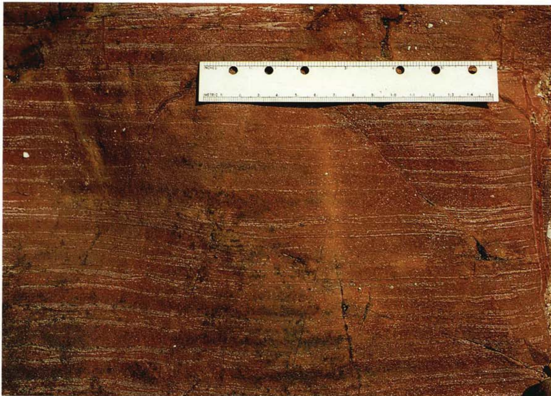
Plate 6 - Finely Laminated Siltstone and Fine-grained Sandstone, of the Carboniferous Mai Po Member on the Western Foreshore (1606 2194) of East Brother Island (Siu Mo To)
