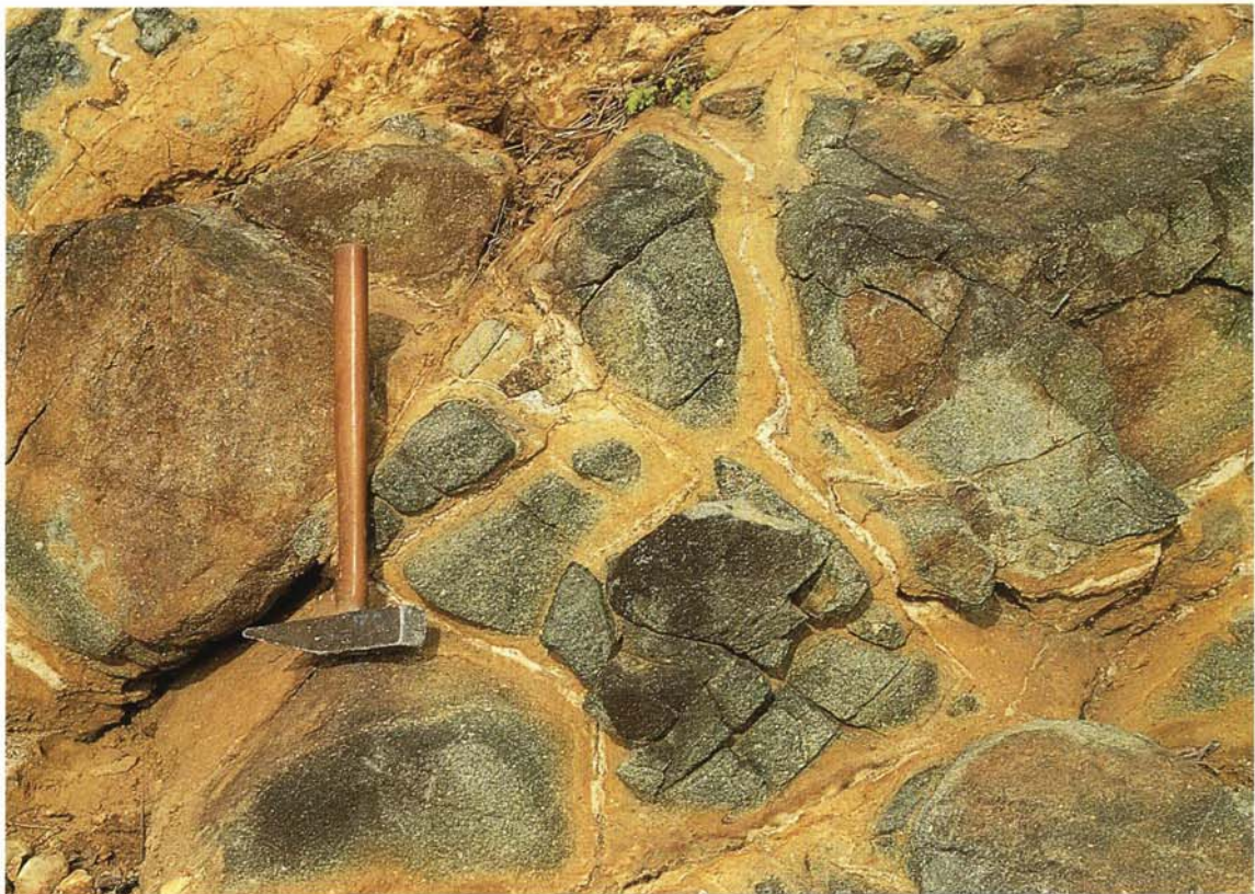
Plate 50 - Corestone Development (Spheroidal Weathering) in Fine-grained Gabbro (1999 1089), East Chi Ma Wan Peninsula
