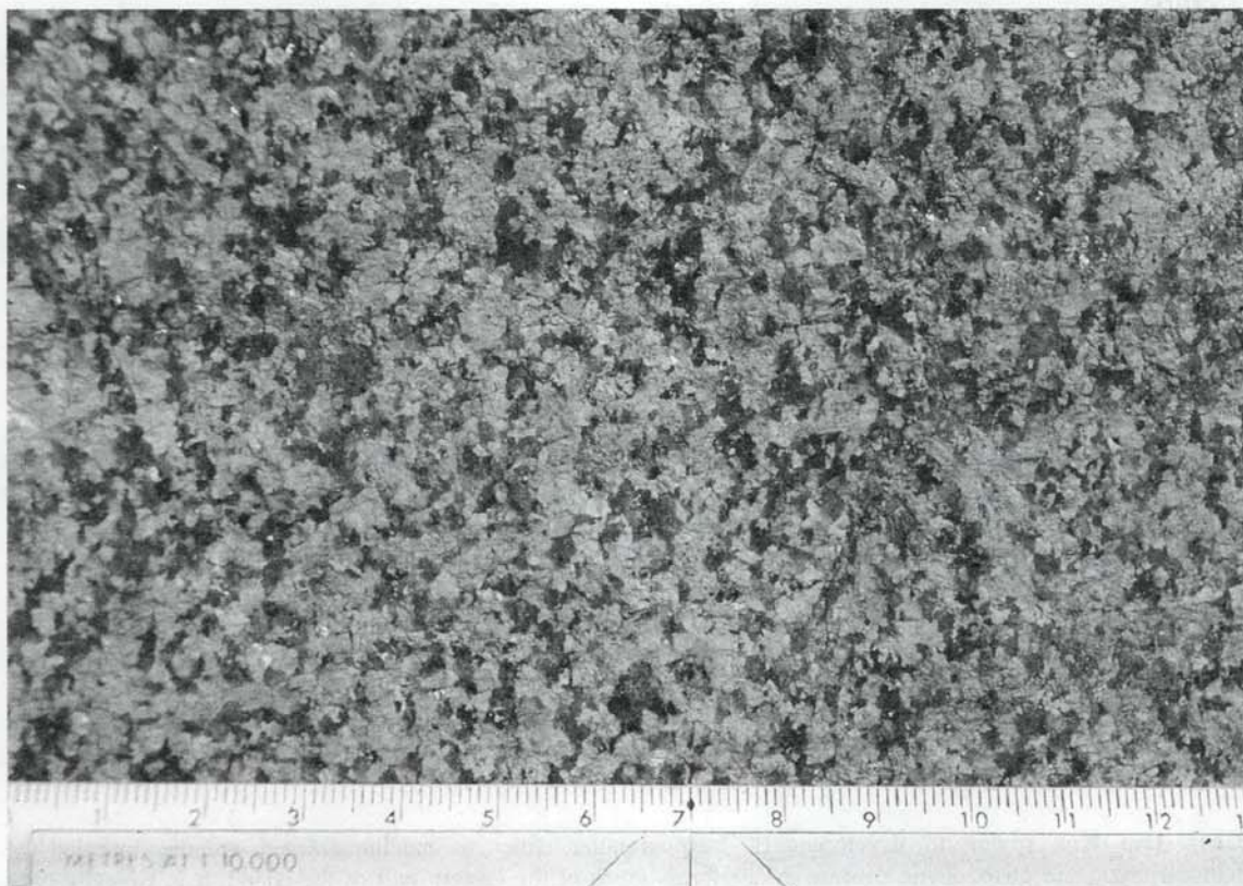
Plate 24 - Fine to Medium-grained Granite (11309 17165), from a Borehole South of Ha Law Wan
