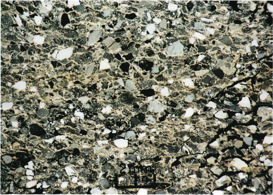
Plate 17 - Thin Section of Lithic Greywacke (HK7406, 4405 3928) within the Lower Cretaceous Pat Sin Leng Formation, Chek Ma Tau; XPL
