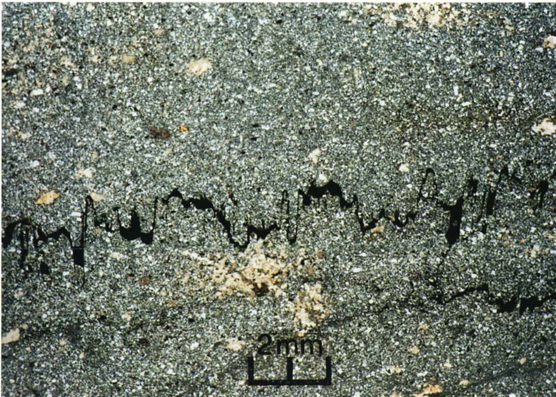
Plate 34 - Thin Section of Chert with Stylolitic Horizon (HK9115, 6276 4422), within the Ping Chau Formation, Chau Tau, Ping Chau; XPL
