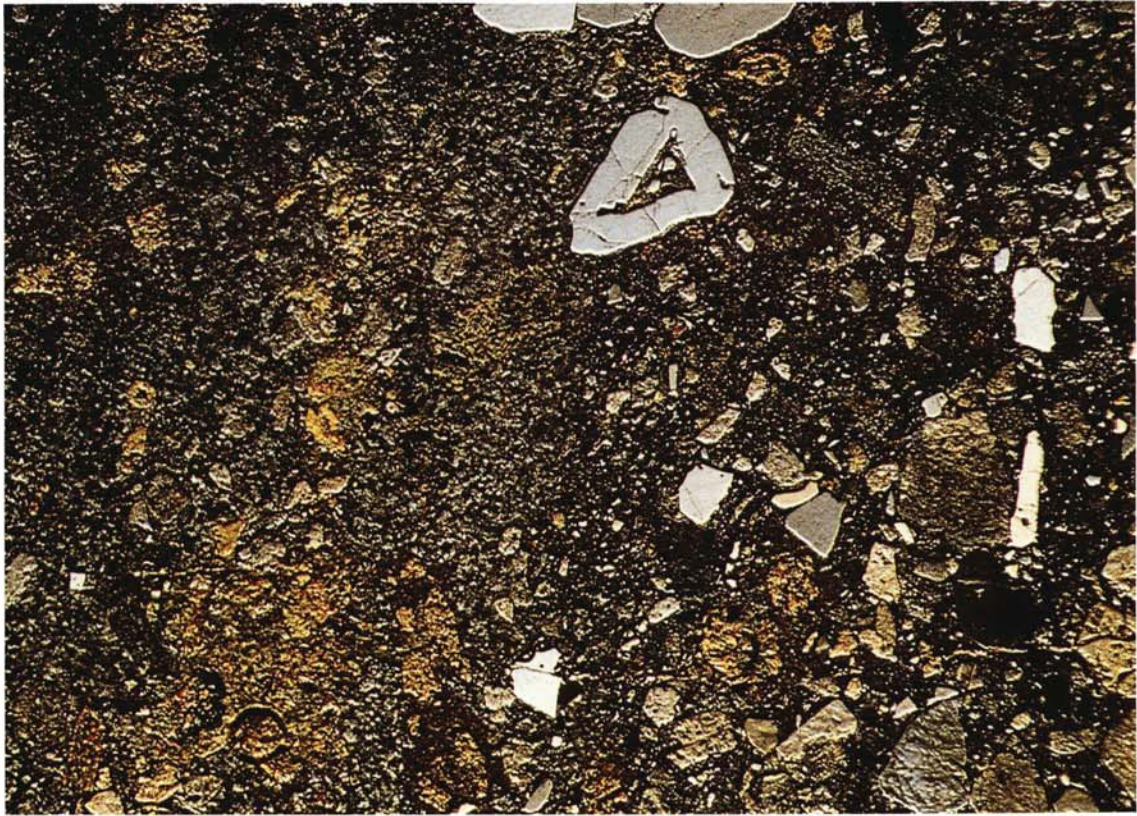
Plate 7 – Thin Section of Diffuse-edged Lapilli in Yim Tin Tsai Formation (HK2263) from Tsing Yi (2678 2427); XPL \times 10
