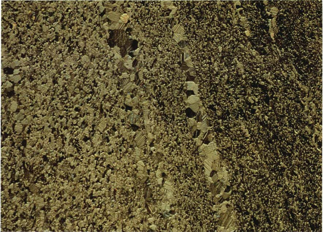
Plate 3 – Thin Section of Marble in Yuen Long Formation (HK3025) from Yuen Long (2056 3573); XPL \times 10
