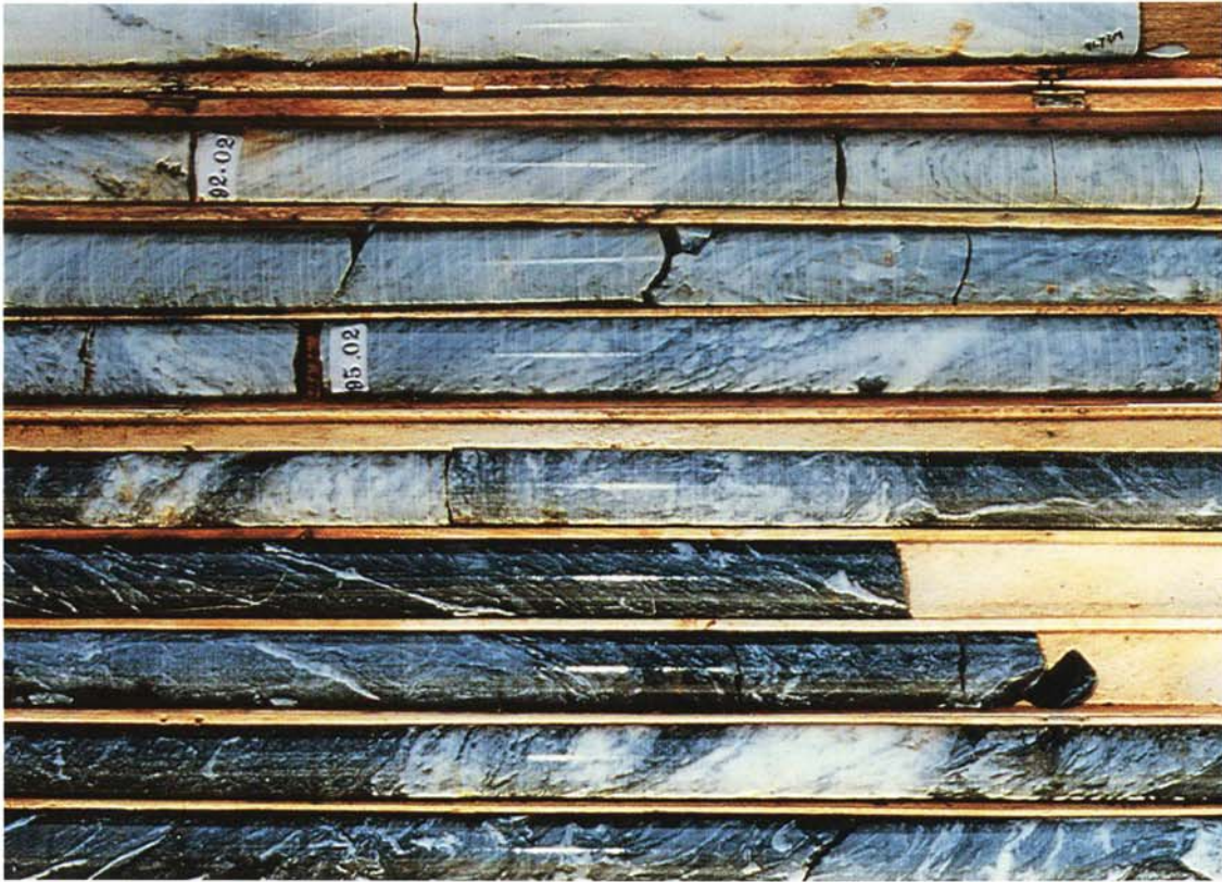
Plate 1 – Gradation from Black Marble to White Marble in Borehole AH98, LRT Interchange, Yuen Long (2171 3401) (Photograph Courtesy of KCRC-SHK JV Development)
