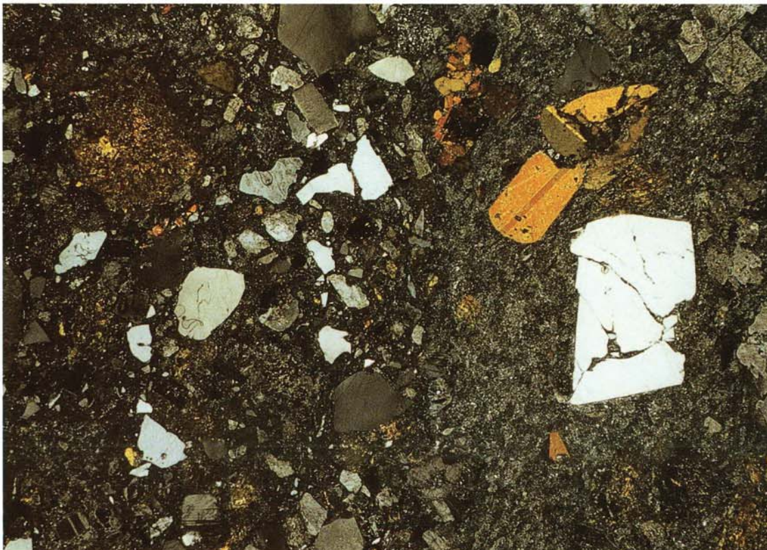
Plate 11 – Thin Section of Lapilli-Ash Crystal Tuff in Shek Lung Kung Member (HK5045) from Shek Lung Kung (2077 2681); XPL × 10
