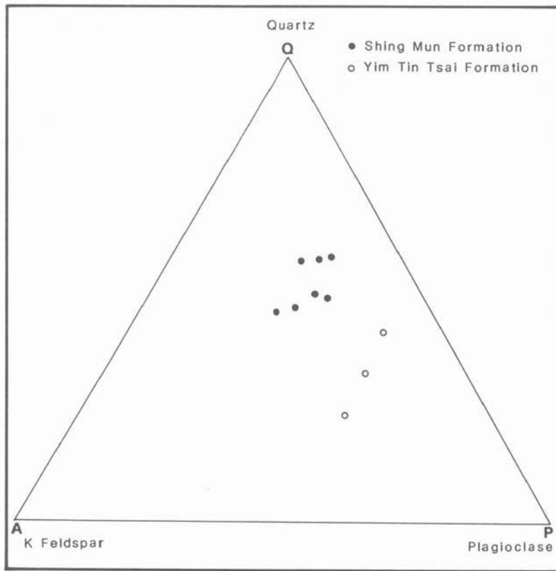
Figure 4 – QAP Diagram Showing Relative Proportions of Minerals in Tuff Samples from the Yim Tin Tsai and Shing Mun Formations (based on point counts of thin sections)
