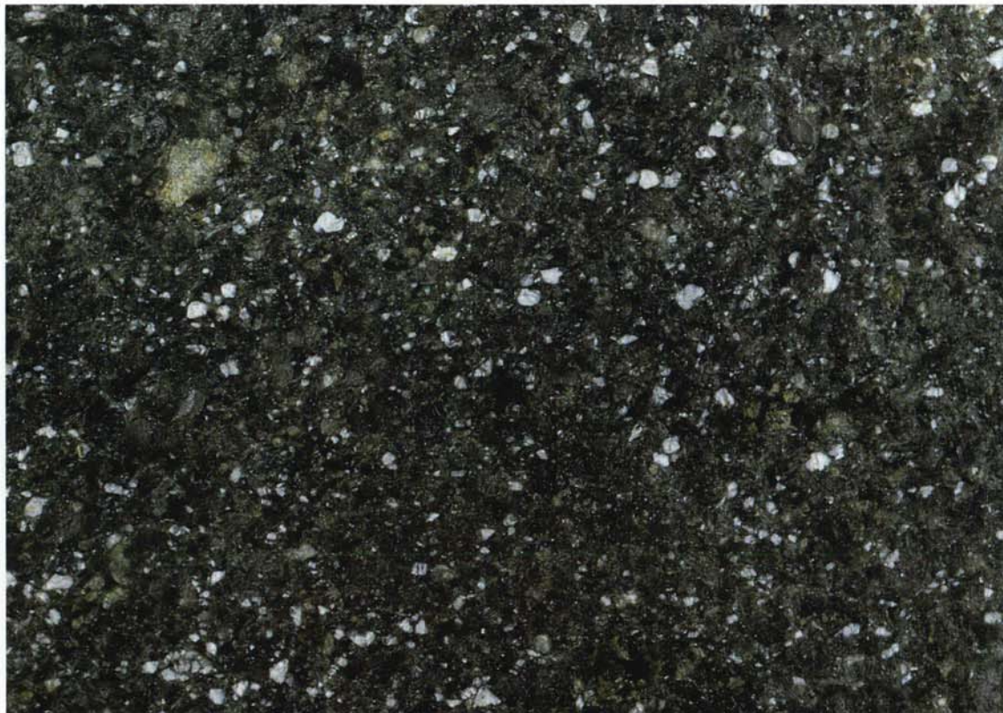
Plate 10 – Lapilli-Ash Crystal Tuff (HK 4951); Tai Mo Shan Formation on Tai Mo Shan (3006 3018); Natural Scale
