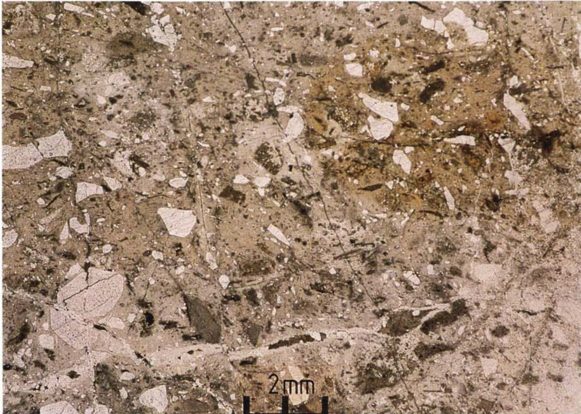
Plate 9 – Thin Section of Vitric Tuff (HK 822); Ap Lei Chau Formation on Ma On Shan (4416 2940); PPL \times 10
