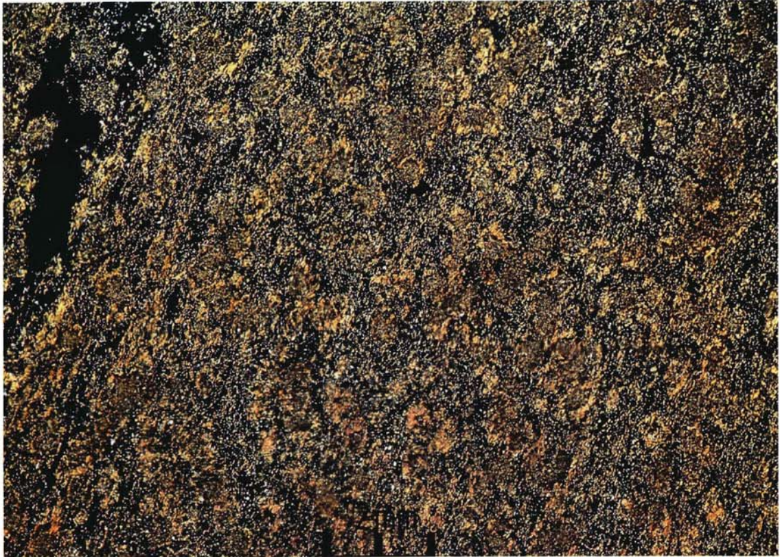
Plate 30 – Crystals of Cordierite in Thermally Altered Siltstone (HK 89) in Tolo Harbour Formation near the Chinese University (3945 3179); XPL \times 10
