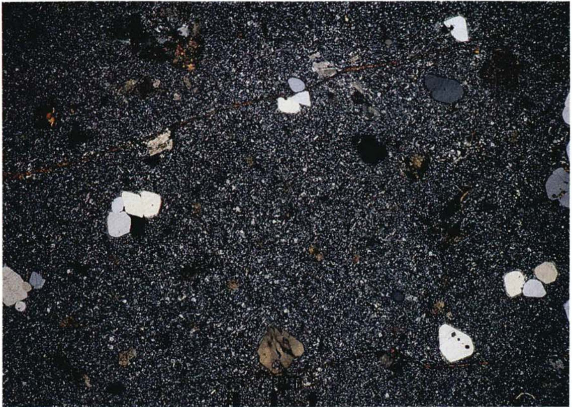
Plate 26 – Thin Section of Quartzphyric Rhyolite (HK 272) in Dyke on Grassy Hill (3584 2930); XPL \times 10
