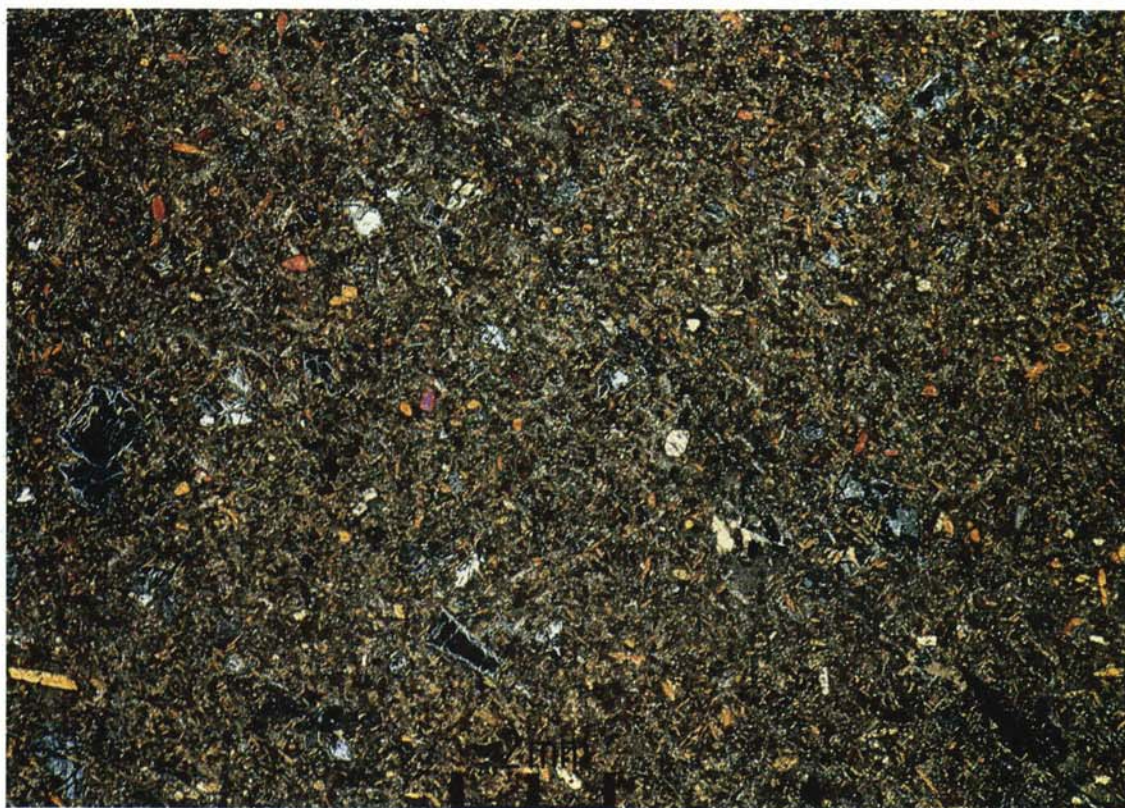
Plate 29 – Thin Section of Basalt (HK 412) in a Dyke at Wai Tau Tsuen (3322 3580); XPL × 10
