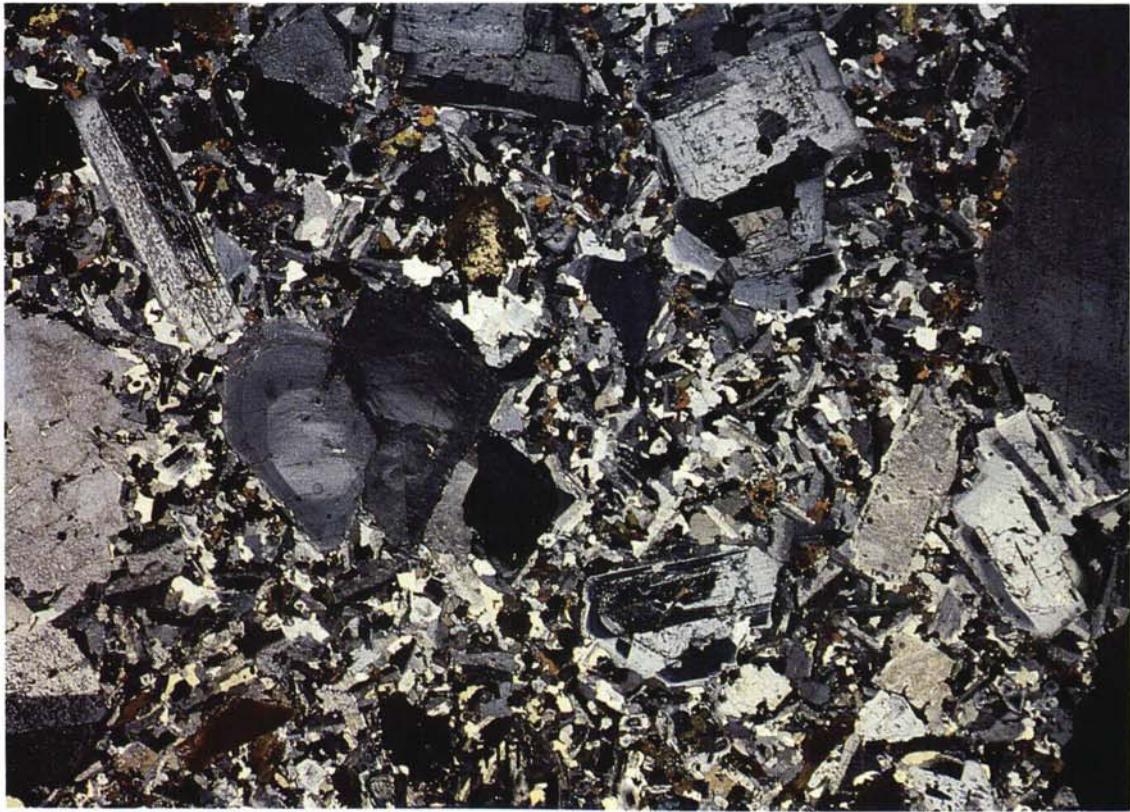
Plate 25 – Thin Section of Quartz Monzonite (HK 537) at Man Tau Tun (3912 2445); XPL \times 10
