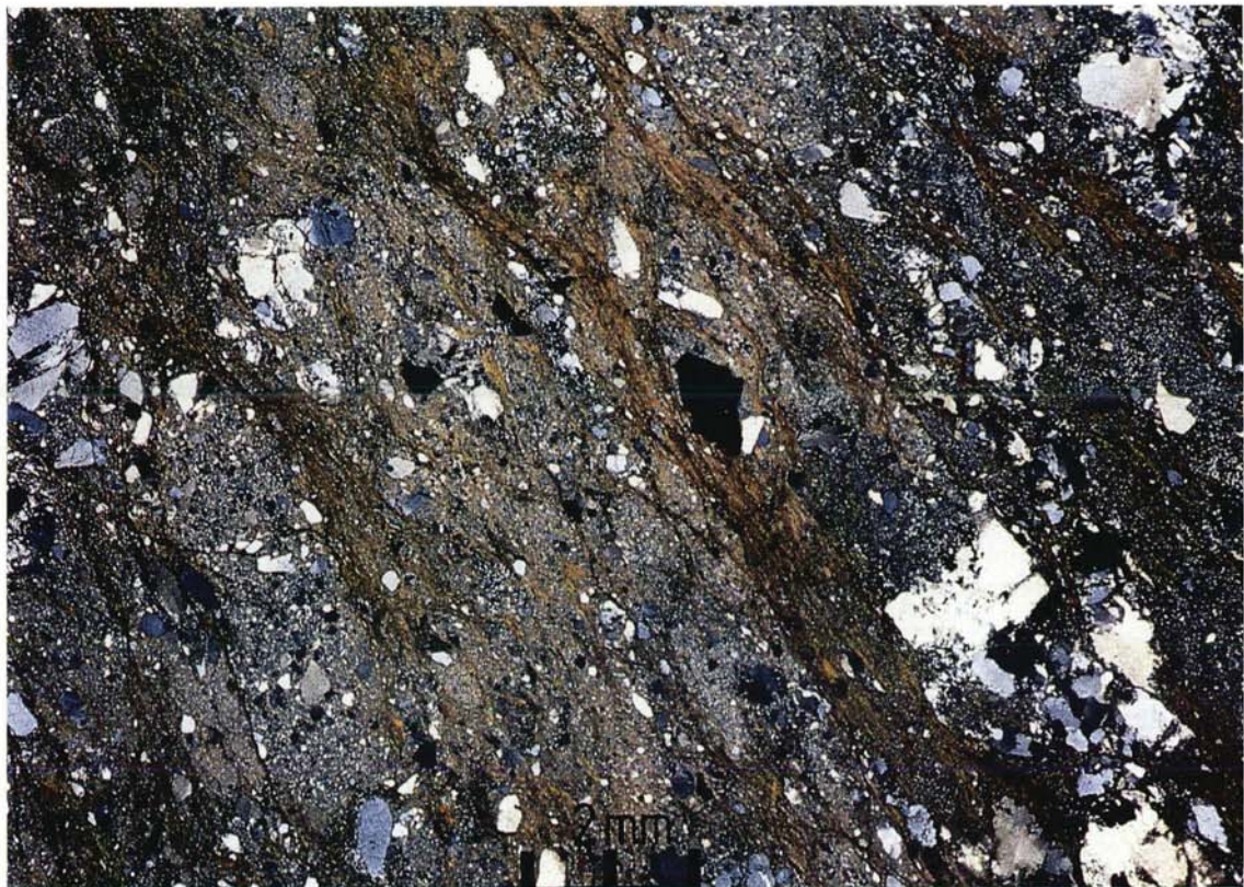
Plate 31 – Biotite in Cleaved Zones of Dynamically Metamorphosed Tuff (HK 341) near Kadoorie Farm (3067 3183); XPL \times 10
