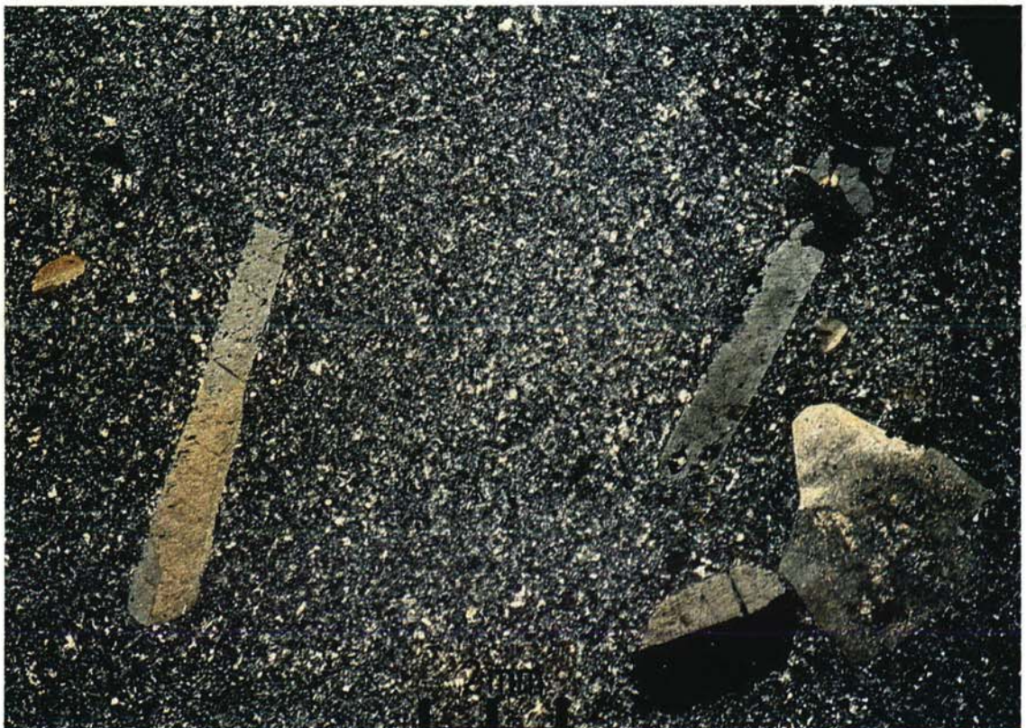
Plate 27 – Thin Section of Feldsparphyric Rhyolite (HK 1245) on Shek Nga Shan (4243 2707); XPL \times 10
