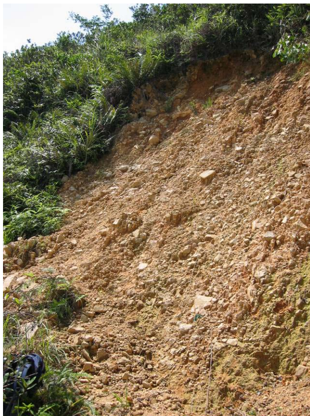
Plate 8 – Planar Surface of Rupture at Landslide 01K (Photograph Taken on 14 August 2002)
