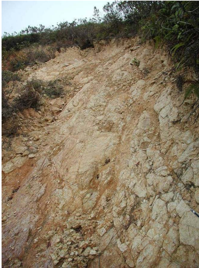
Plate 13 – Planar Persistent Joint along Western Flank of Landslide 01EE (Photograph Taken on 28 November 2001)
