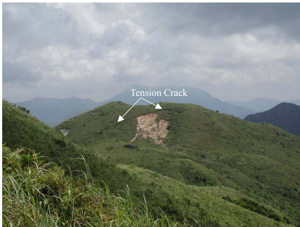
Plate 16 – View of Tension Crack at Landslide 01N (Photograph Taken on 9 August 2001)
