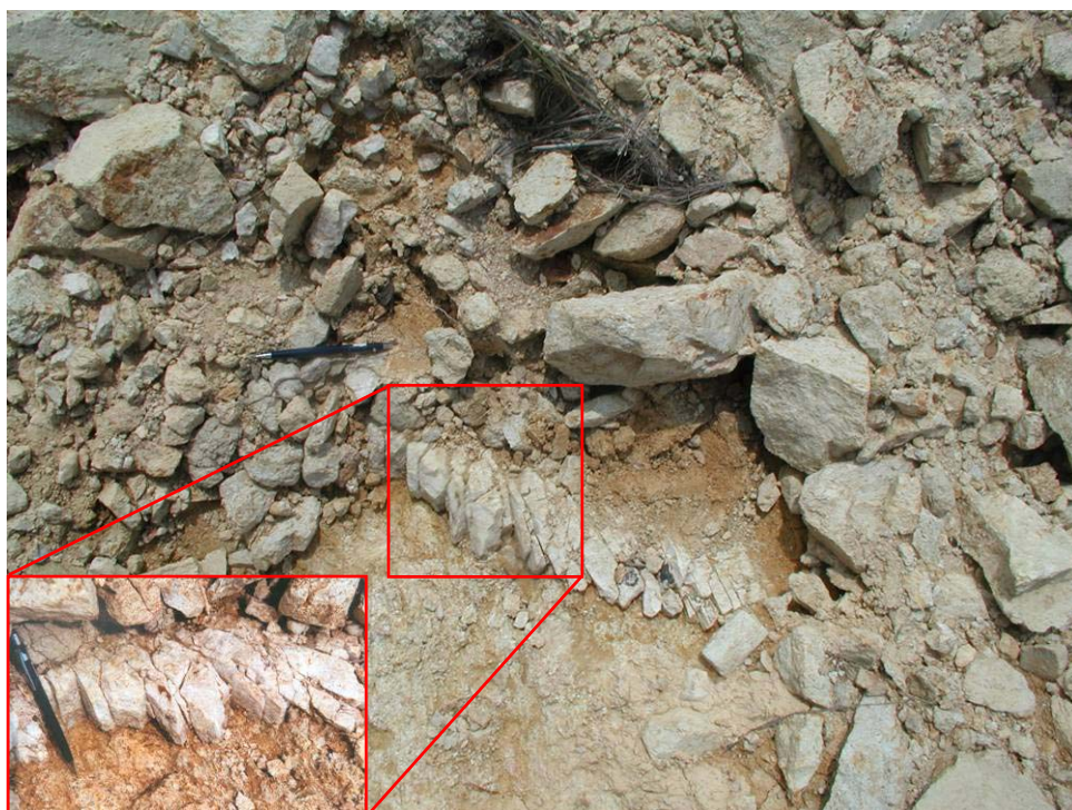
Plate 12 – Quartz Vein Parallel to Surface of Rupture of Landslide 01N (Photograph Taken on 18 October 2001)
