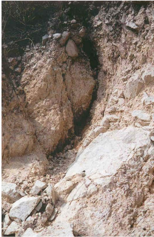
Plate 17 – Partially Displaced Mass Below Tension Crack at Landslide 01N (Photograph Taken on 18 October 2001)
