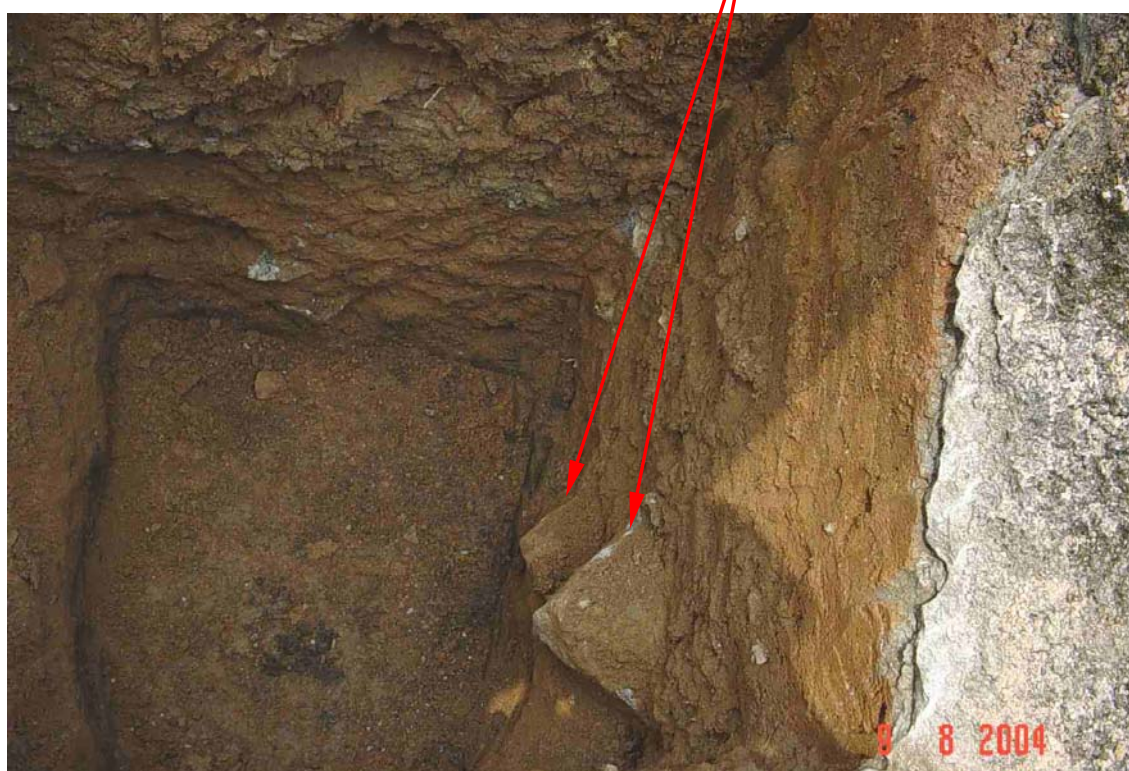
Plate 28 - Example of Rock Blocks Exposed within Compacted Fill Layer in Trial Pit TP4 (Photograph taken on 9 August 2004)
