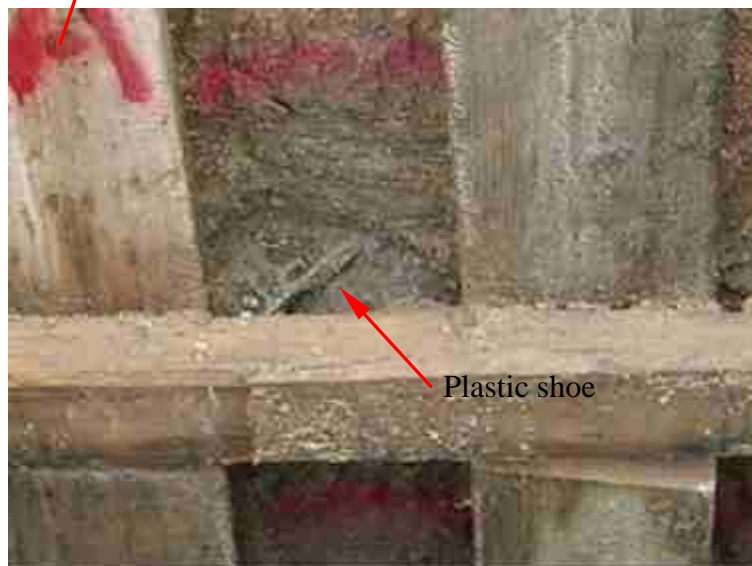
Plate 29 - Remains of Plastic Shoe Exposed within Compacted Fill Layer in Trial Pit TP6 (Photograph taken on 25 August 2004)
