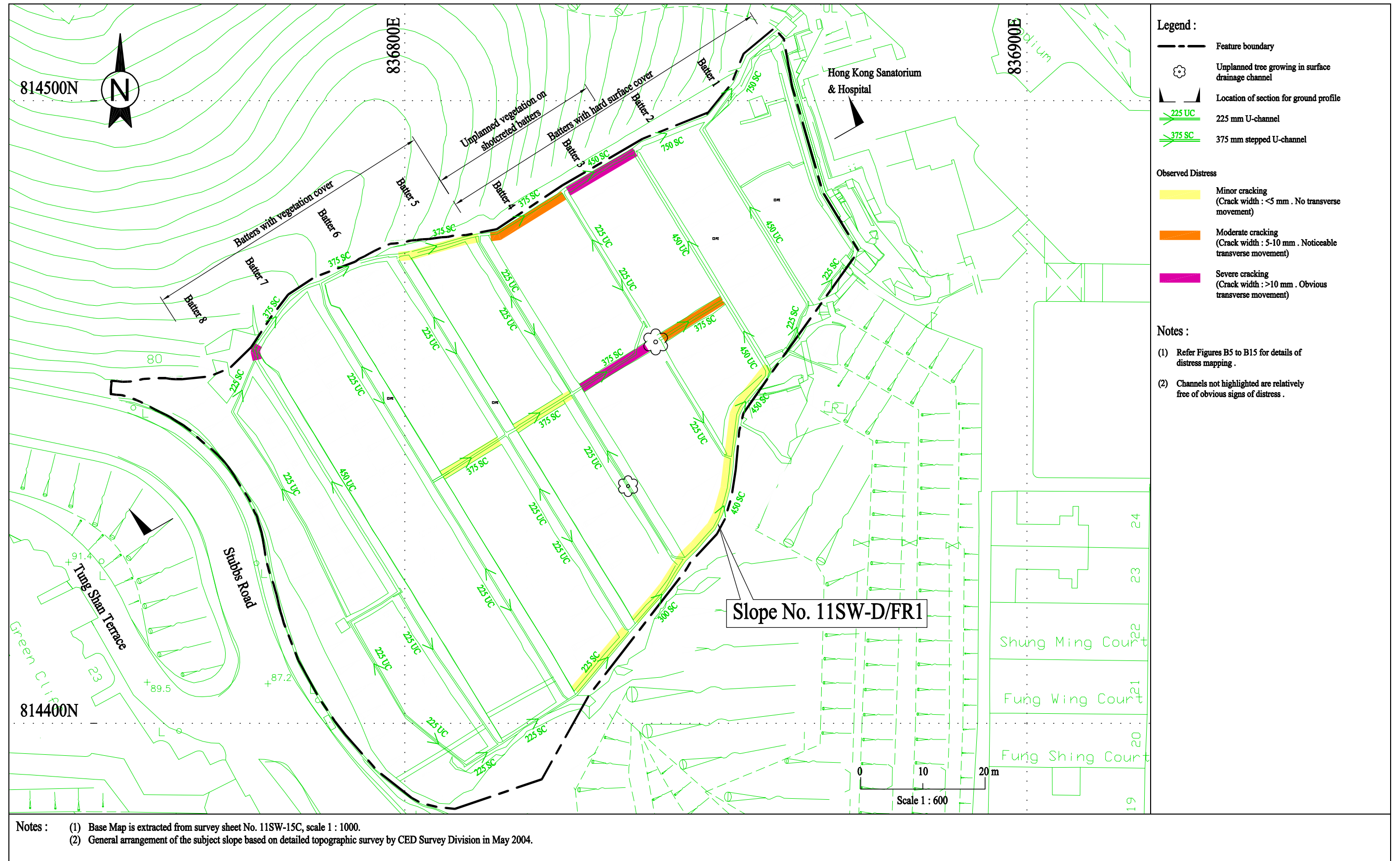
Figure B4 - Distress Mapping of Slope No. 11SW-D/FR1 - Relative Distress in Stepped Channels
