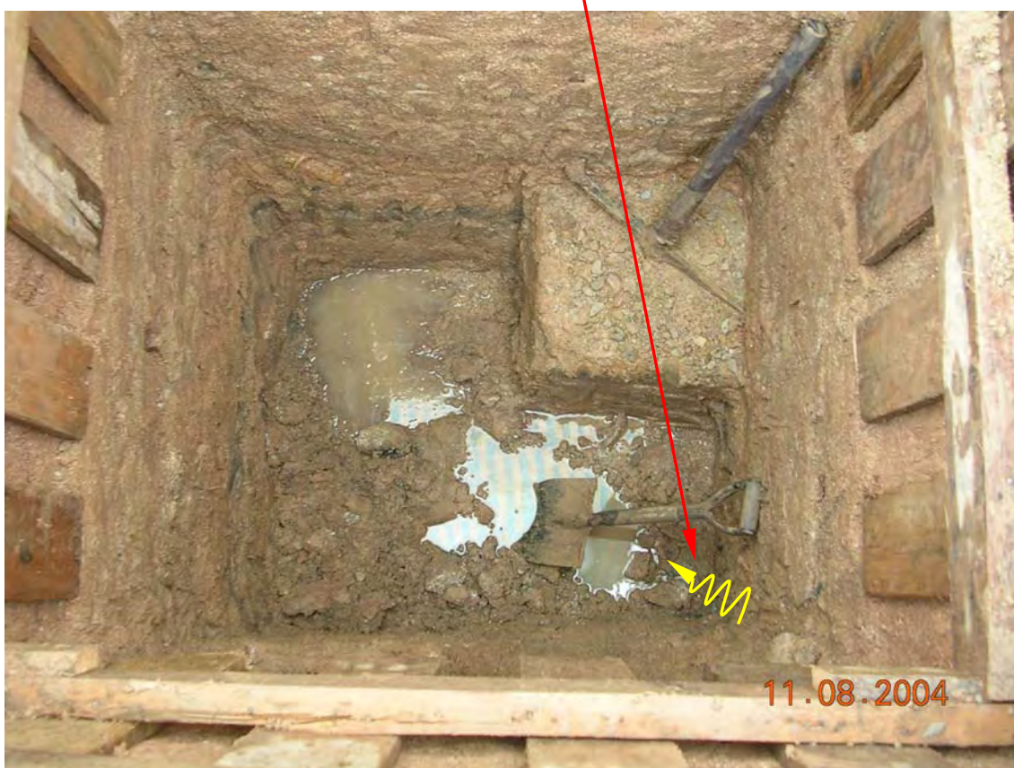
Plate 32 - Seepage Observed in Trial Pit TP5 during Excavation (Photograph taken on 11 August 2004)
