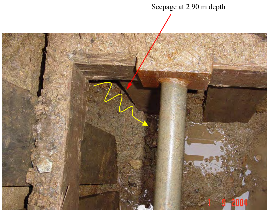
Plate 33 - Seepage Observed in Trial Pit TP6 during Excavation (Photograph taken on 1 September 2004)
