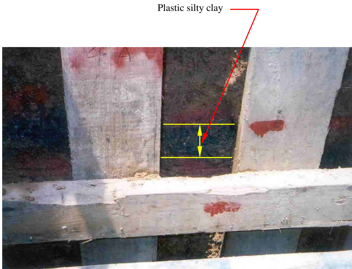
Plate 30 - Layer of Plastic Silty Clay Exposed within Compacted Fill Layer in Trial Pit TP4 (Photograph taken on 25 August 2004)
