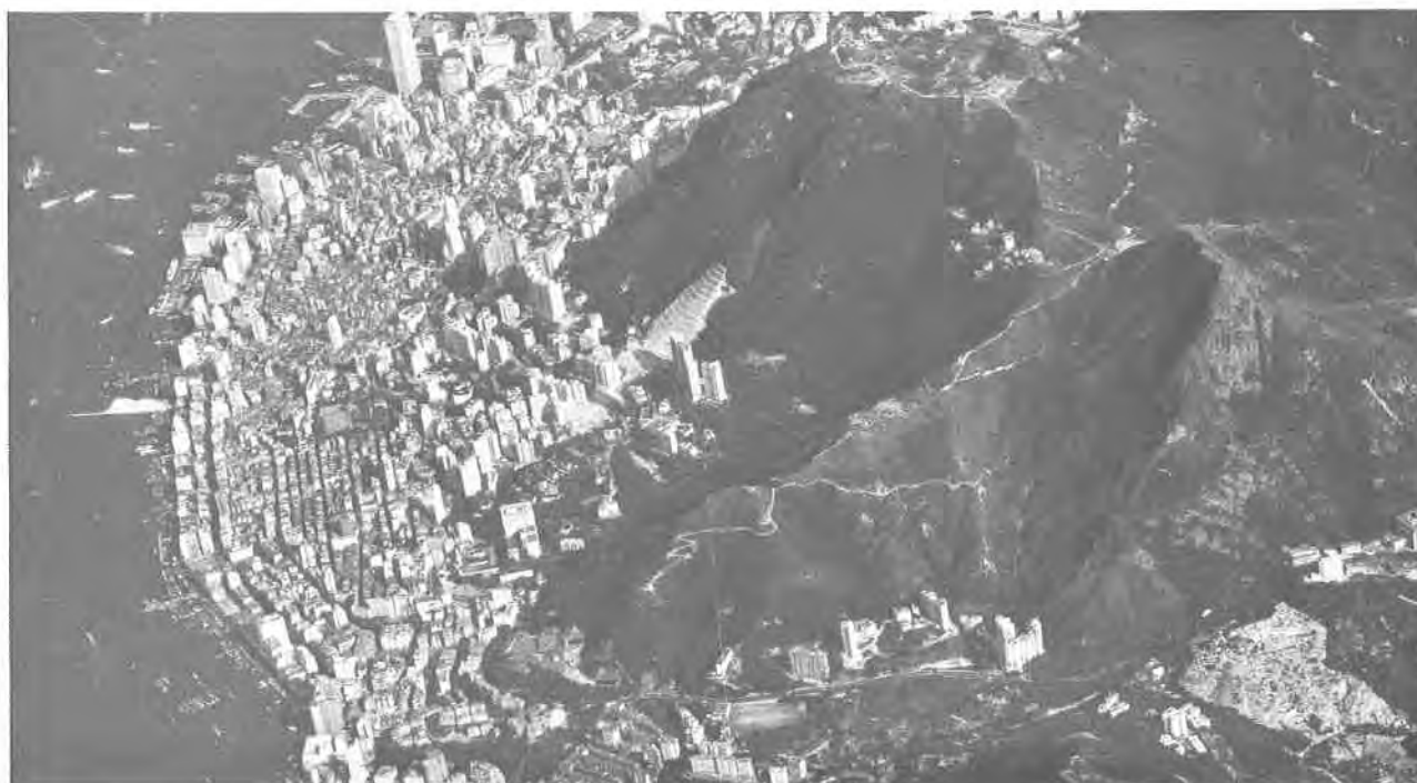
Plate 105. Oblique Aerial Photograph of Remedial Works to the Po Shan Road Landslip Site in October 1973. Reinstatement of the middle to upper portions of the landslide scar above Po Shan Road is clearly visible. Much of the slope is grassed, and surface drainage has been installed. Po Shan Road has been reinstated. (24.10.1973/5466).
