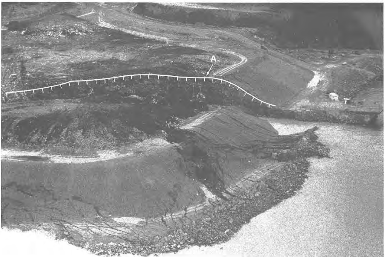
Plate 160. Oblique Aerial Photograph of Failure of Landfill at Junk Bay in 1984. This photograph views the site in an easterly direction. The multiple sets of tension cracks are clearly evident. The major line of failure is indicated at A. (GCO/MW/1984/64/84/15).
