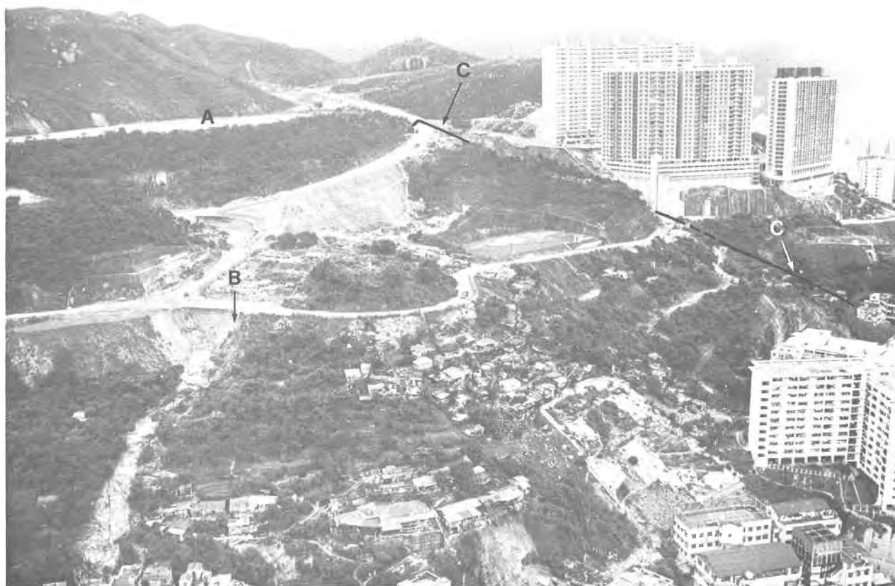
Plate 60. Oblique Aerial Photograph of Braemar Reservoir in 1966. Overflow from the Reservoir (A) caused serious flooding and damage evident in Plates 62–63 and 65–67. A large washout is evident on Tin Hau Temple Road (B). The severe damage in the Ming Yuen Street–King's Road area was caused by stormwater runoff which flowed along the natural stream course indicated in the western portion of the area (C). (Reproduced from Chen (1969), ISD/3982/275).
