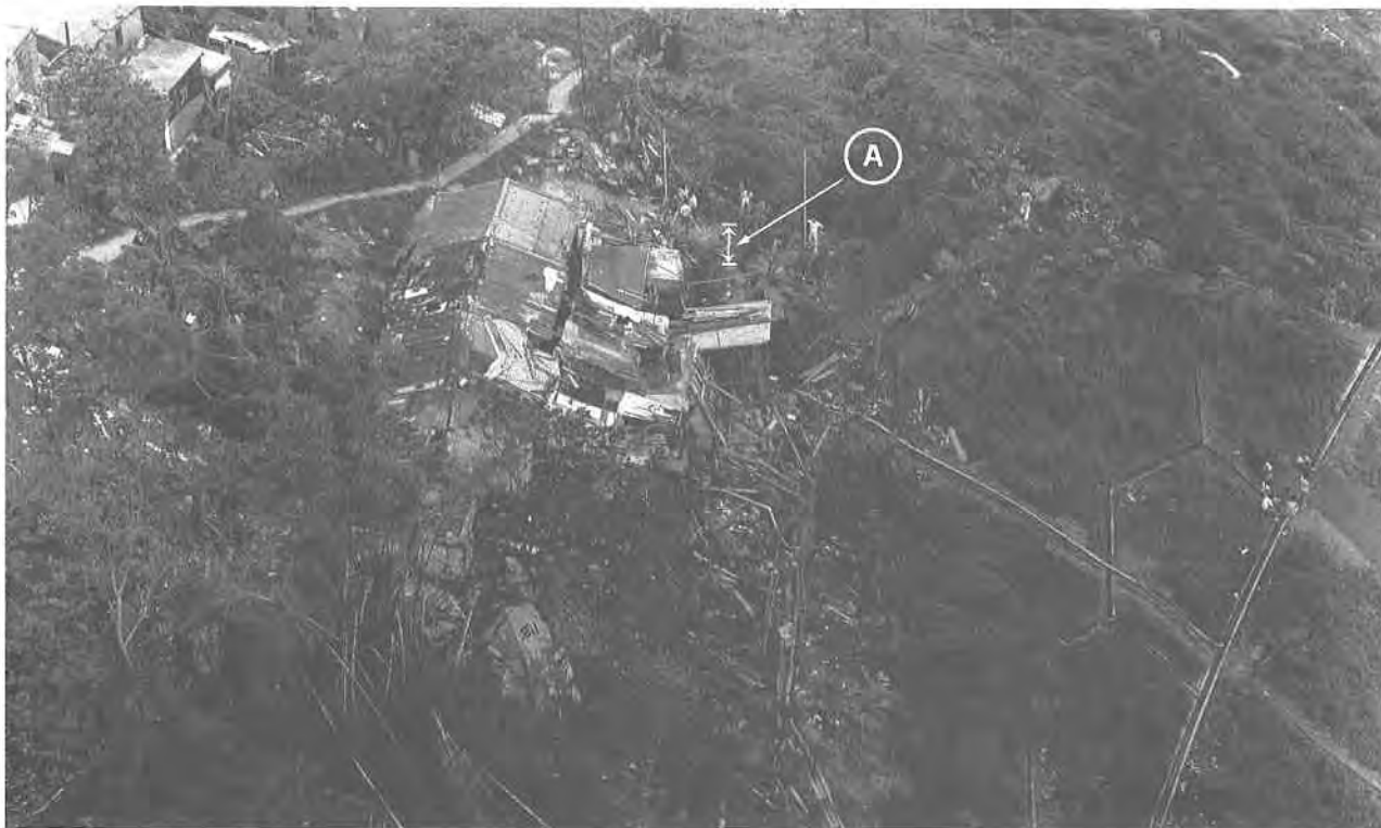
Plate 172. Oblique Aerial Photograph of Slope Failure at Pun Shan Tsuen in October 1983. The backscar of the landslide caused major distress to a number of huts at the the crest of the slope. A vertical displacement of approximately 1m is evident at (A). A general view of the slope is given in Plate 171. (GCO/OAP/1983/PS400-7).
