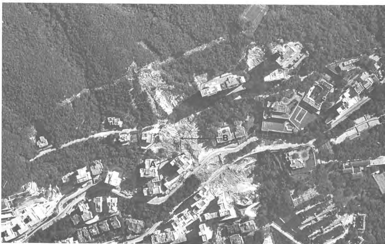
Plate 102. Site of the Po Shan Road Landslip in October 1972. This plate shows the state of remedial works to the site some 3.5 months after the landslip. Access has been cleared across Conduit and Kotewall Roads. Clearing operations are still being carried out, and preliminary slope works appear to be underway. Debris has been removed from around Skyline Mansions (A), and the large boulder evident at A in Plate 96 has been removed (B). (3.10.1972/2303).
