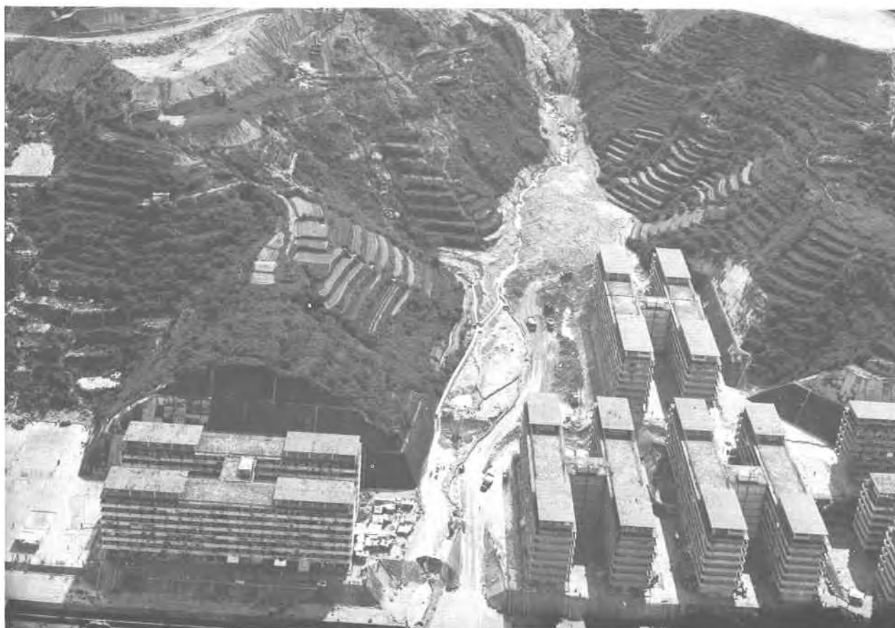
Plate 52. Oblique Aerial Photograph Looking Northeast towards the Landslip at Tsui Ping Road Estate in 1964. Hong Kong was badly hit by Typhoon Ida in August 1964. Two landslips occurred on a fill slope under construction on terrain upslope of Tsui Ping Road in the Kwun Tong area of Kowloon. The first landslip was early in the morning of 10.8.1964, after intense rainfall the previous day. Reports indicate that a mud avalanche flowed down the valley and deposited up to 3m of debris in an area approximately 90m by 70m in a resettlement estate. Surprisingly, only three people were listed missing, and no other injuries were reported. Six days later, at the same location during heavy rain on 16.8.1964, a second smaller landslip occurred shortly after 3.30 p.m. The Royal Observatory recorded a 24 hr rainfall of 2.86 inches (72.6 mm) for 16.8.1964. Five injuries were recorded, and hundreds were evacuated from their homes in the Kwun Tong Estate. In this Plate, taken approximately 2 weeks after the second landslip, trucks are evident removing debris from around the housing blocks. (ISD/30.8.1964/3276/1).
