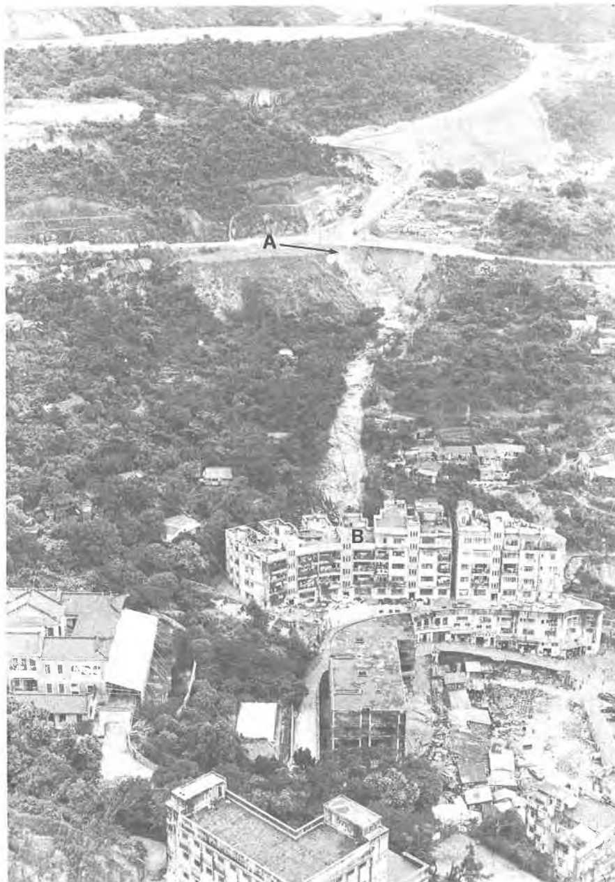
Plate 61. Oblique Aerial Photograph of Washouts on Braemar Reservoir Road and Tin Hau Temple Road in 1966. A large washout is evident at the intersection of Tin Hau Temple Road and Braemar Reservoir Road (A). The multi-storey development at B is near Kai Yuen Street. (Reproduced from Chen (1969), ISD/3982/318).
