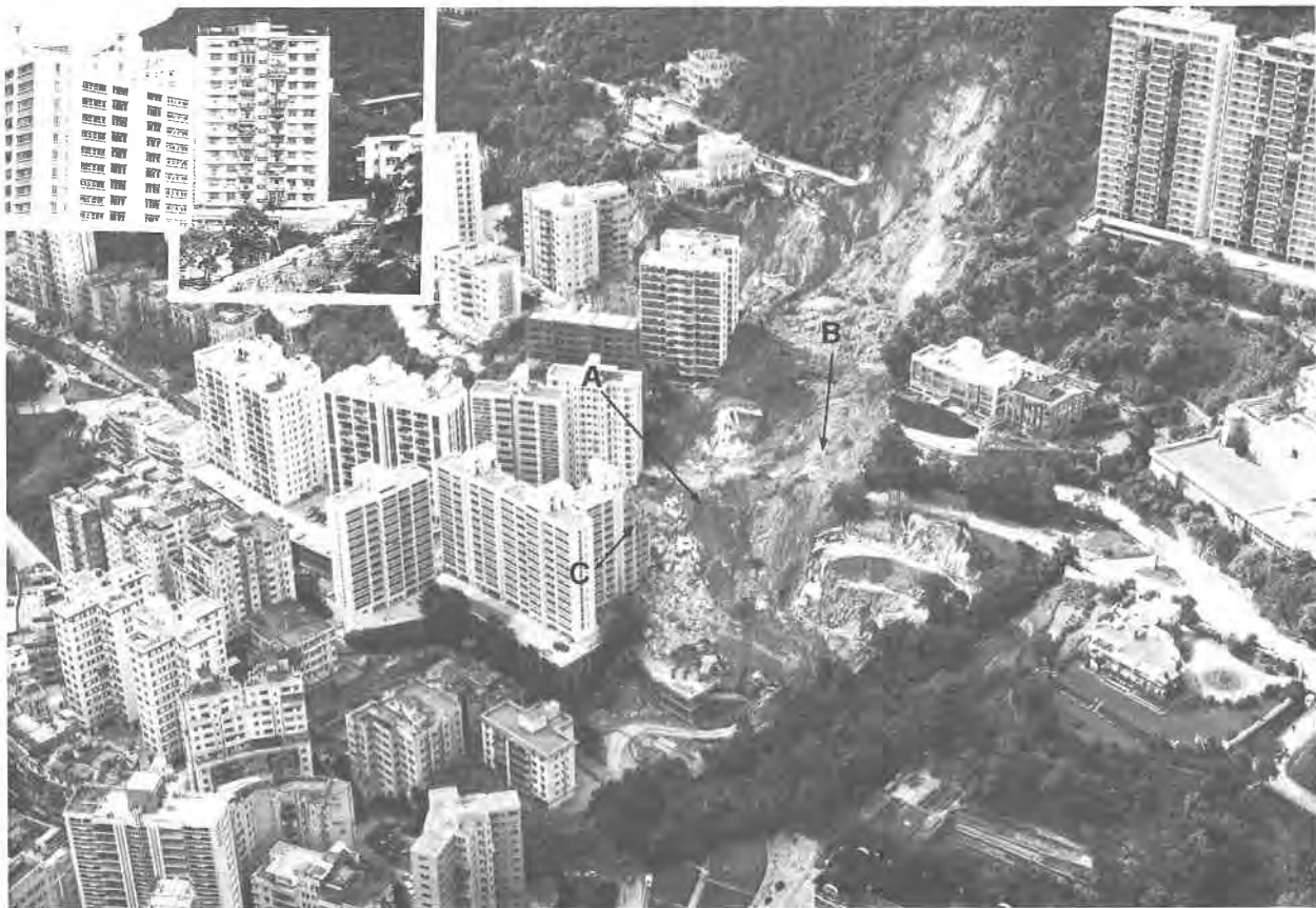
Plate 94. Oblique Aerial Photograph of the Po Shan Road Landslip in the Mid-levels Area in 1972. On 18.6.1972, a large landslide occurred in the Mid-levels of Hong Kong Island. A multistorey residential building (Kotewall Court) collapsed during the failure. There were 67 fatalities and twenty injuries in this incident. The landslide occurred between 8.50 and 8.55 p.m., after three days of abnormally heavy rainfall. Part of the hillside above a cut slope failed and the debris descended across Conduit Road, and then to Kotewall Road. A witness indicated that the major landslide took only seven to ten seconds (Government of Hong Kong, 1972b). This landslide also destroyed a four-storey house which was evacuated following slope movement some 4 hours before the major landslide. The location of Kotewall Court and the House are shown at A and B respectively, and on Plate 93. Damage to the upper stories of Greenview Gardens is evident at C. Kotewall Court collapsed onto Greenview Gardens, which was unoccupied at the time. The top of the landslide was at an elevation of approximately 230m and the toe of the debris reached 110 m, a vertical fall of some 120 m (Lo, 1978). The horizontal distance was approximately 255 m. (21.6.1972/ISD/8264/5). The inset in the top left hand corner shows Kotewall Court and the House at 11 Kotewall Road before the disaster. The actual date of the photograph is unknown, but it is likely that this photograph was taken only a matter of weeks before the failure. Scaffolding is evident on Greenview Gardens. (6729/72).
