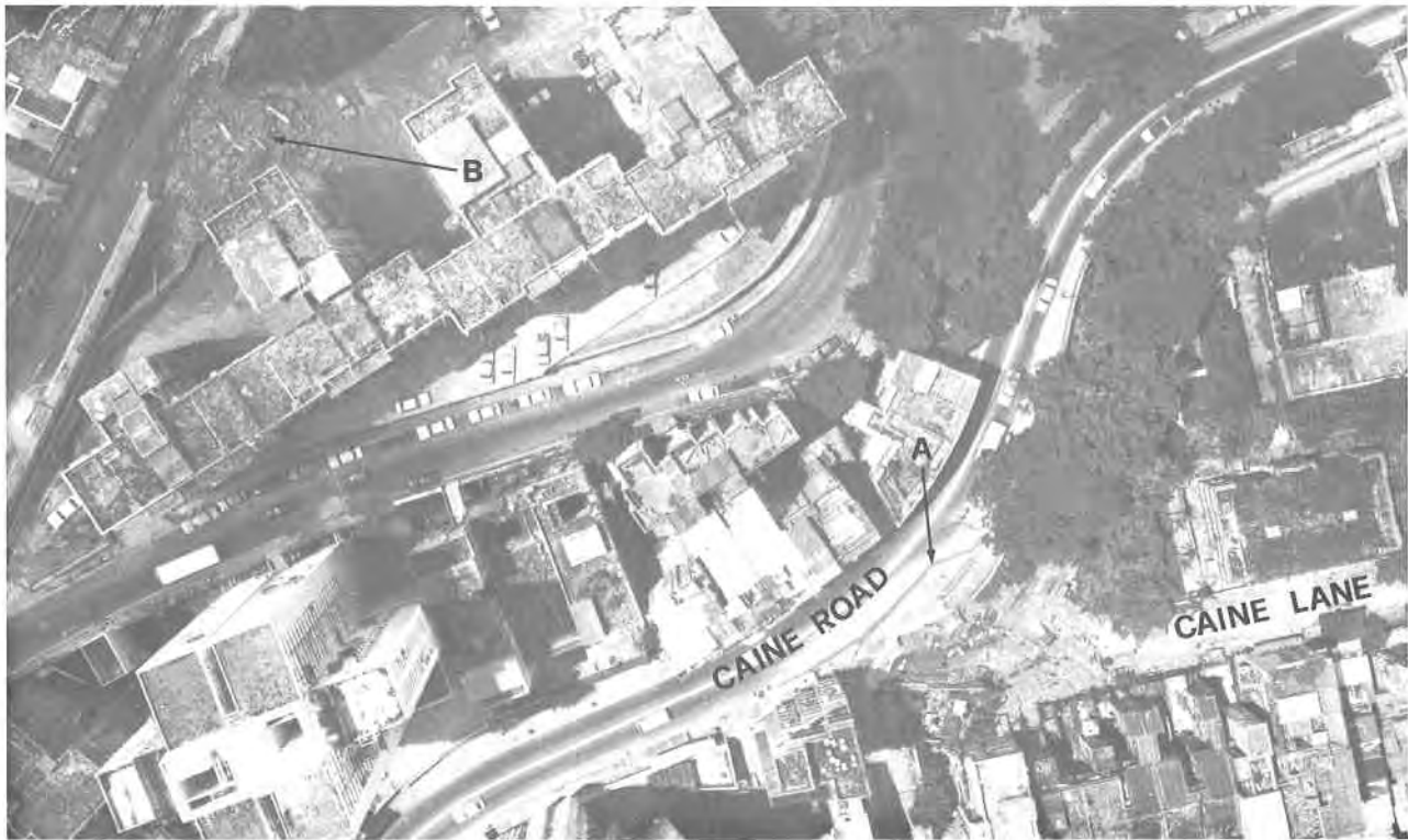
Plate 116. Aerial Photograph of the Caine Lane Retaining Wall Failure in 1976. The retaining wall between Caine Lane and Caine Road, in the Mid-levels District, collapsed on 25.8.1976. The failure (A) occurred at an elevation of approximately 70mPD. Three old masonry retaining walls supported Caine Road and Caine Lane, the lowest of which failed. Some 400 people were evacuated following this failure. Another retaining wall failure (B) occurred on the same day in Castle Road, collapsing onto the grounds of Merry Terrace. The wall was some 10m high and the failed portion was some 18m in length, at about 95mPD. (26.8.1976/15085).
