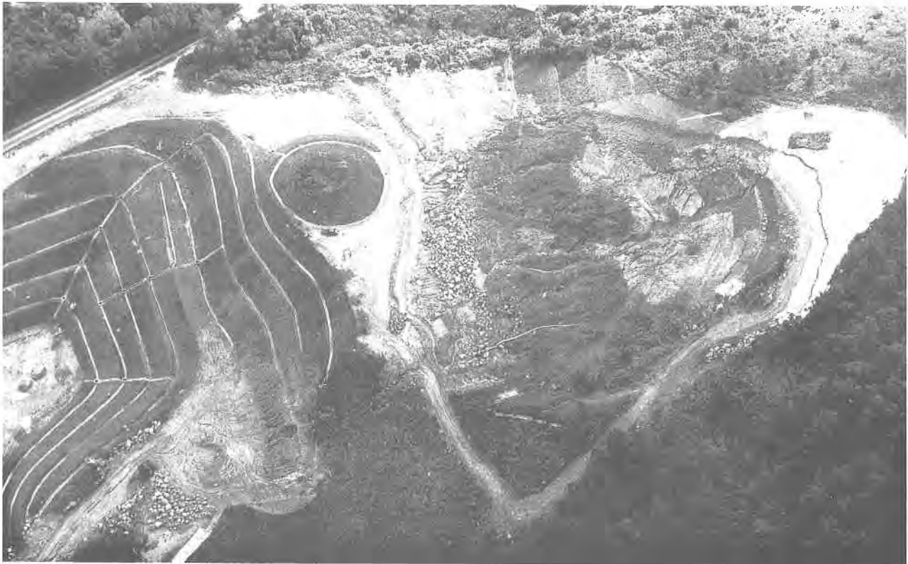
Plate 131. Oblique Aerial Photograph of a Landslip near Kwun Yam Shan in July 1979. A landslide occurred during site formation for a large development near Kadoorie Farm. This photograph was taken during July 1979. Compare this with Plate 132, which was taken some 3 months later in October 1979. (GCO/OAP/1979/PS51-20A).
