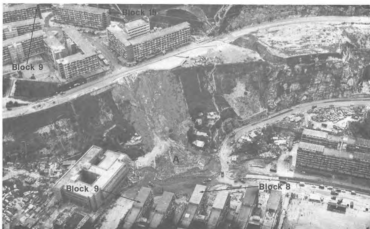
Plate 107. Oblique Aerial Photograph of Sau Mau Ping Landslip Site in 1972. On the afternoon of 18.6.1972, between 1.10 and 1.24 p.m., a massive landslide occurred on a fill slope between Hiu Kwong Street and Tsui Ping Road in Sau Mau Ping, Kowloon. This landslide followed some 6 weeks of continuous rainfall, culminating in 3 days of intense rain. The Royal Observatory recorded a total rainfall of 652.3 mm during the period 16–18.6.1972. This shallow failure took the form of a high velocity flowslide, and was probably due to 'liquefaction' caused by the super-saturation of uncompacted fill material. A large number of huts (A) were buried by mud, with 71 killed and 60 injured. The locations of Blocks 9 and 15 affected by landslips in 1976 are also shown. Compare this with Plate 111. Plates 108 and 109 provide further coverage of the 1972 failure. (ISD/21.6.1972/8264/11).
