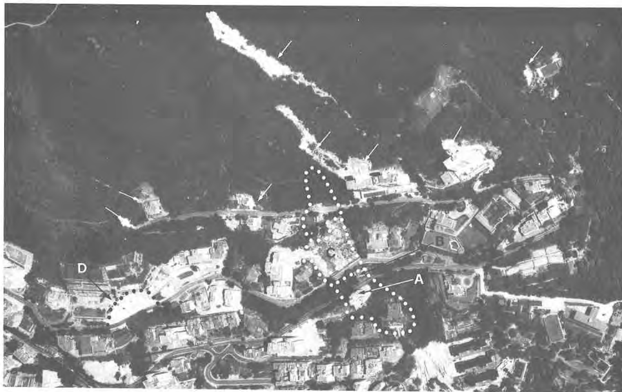
Plate 93. Enlargement of Aerial Photograph of Landslips in the Mid-levels Area in 1967. The major landslips are arrowed. The general extent of the Po Shan Road landslip in 1972 (Plates 94 to 100) is shown, and the location of Kotewall Court is indicated at A, and the house at 11 Kotewall Road at B. Both these structures were destroyed during the major Po Shan Landslip at about 9.00 p.m. on 18.6.1972. A large cut platform is evident at C, and seepage is also apparent across the platform. Remedial measures appear to be underway on the site of the retaining wall failure in 1966 (D), which is shown in Plate 73. This Plate accompanies Plate 92. (1967/5606).
