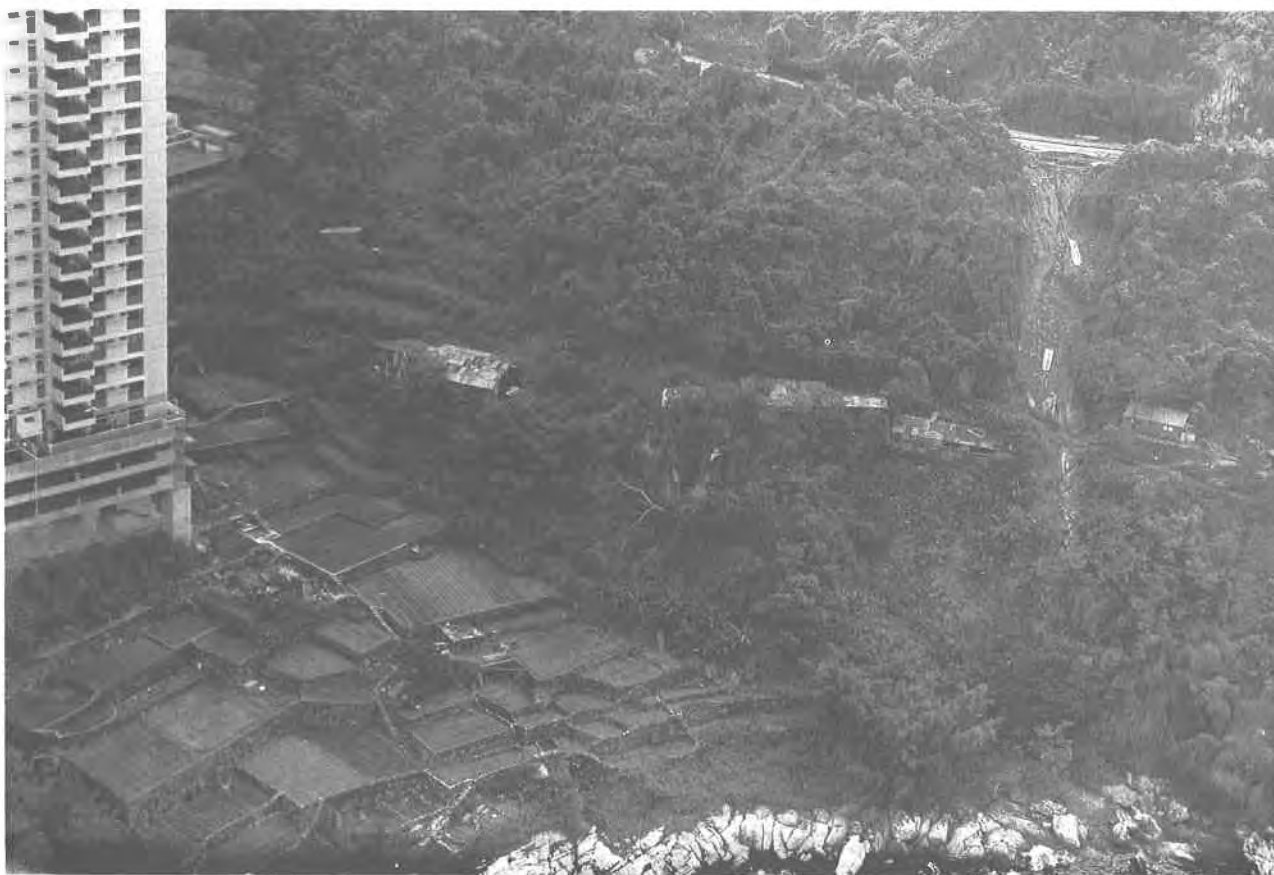
Plate 133. Oblique Aerial Photograph of a Landslip below Victoria Road in 1979. This landslide occurred during Typhoon Hope in September 1979 and affected huts in a mid-slope position near Baguio Villa. (GCO/OAP/1979/PS75-6A).
