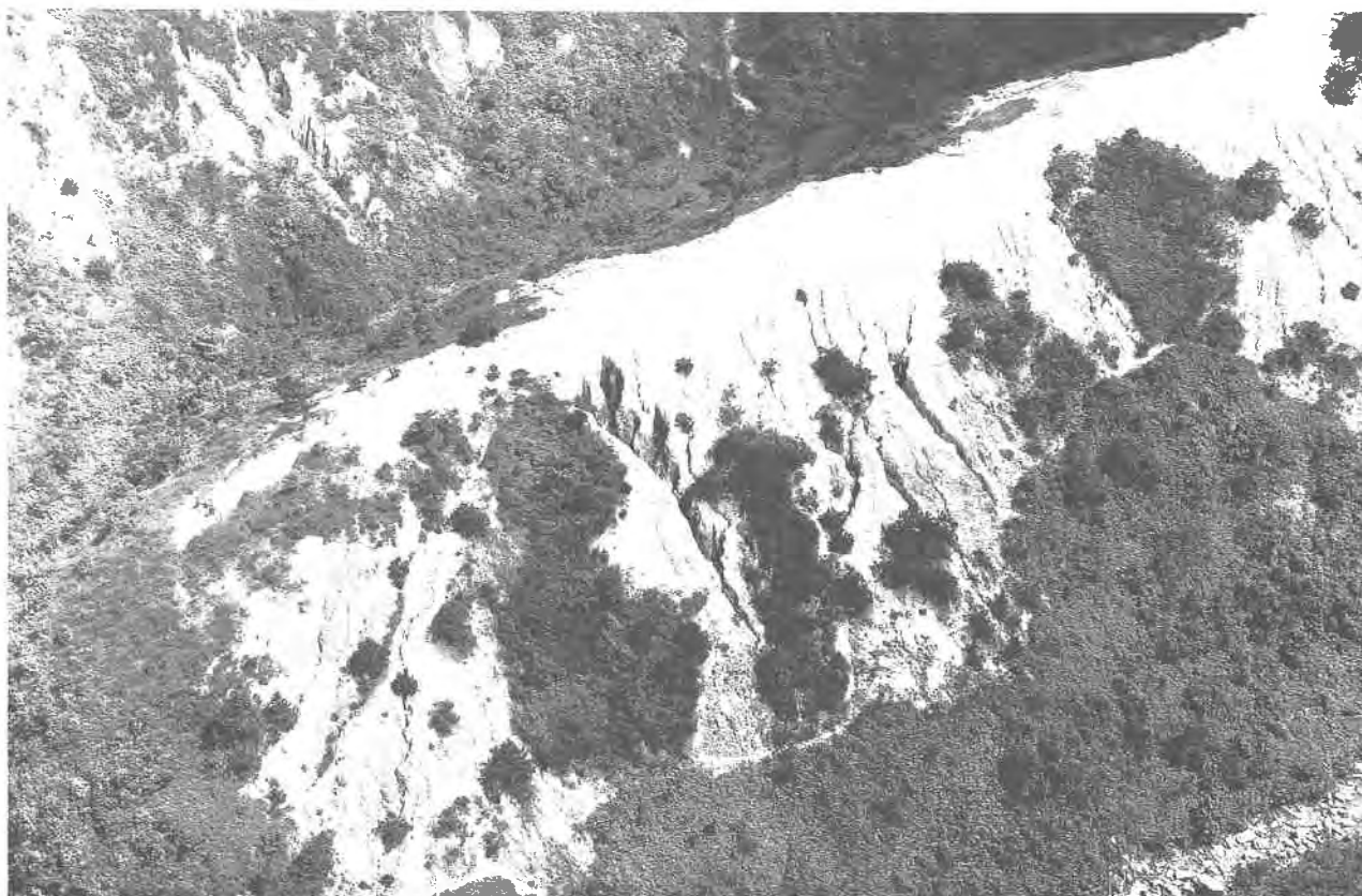
Plate 198. Oblique Aerial Photograph of Severely Eroded Granitic Terrain near Ha Pak Nai in 1978. This photograph highlights the nature and occurrence of gully erosion on granitic terrain in the western New Territories. Deep gully incision is evident near the crest of the slopes and becomes more shallow in a downslope direction. (GCO/OAP/1983/PS372-10).
