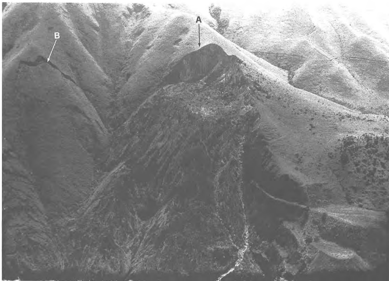
Plate 128. Oblique Aerial Photograph of Landslip at Ma On Shan Mine Site in 1979. The landslide associated with old mine workings at Ma On Shan is easily the largest area of instability within the Territory. Taken in 1979, this photograph shows the unstable mine workings, and the extensive system of tension cracks on the south-facing natural hillside. Instability was first apparent in 1954 in the area indicated at A. Evidence of the first incidence of the large tension cracks on the south-facing slope (B) was apparent in aerial photographs taken in 1969, and by 1973 they were clearly defined. The tension cracks have enlarged since 1973. Extensive underground operations associated with mining occurred between 1953 and 1976, and tunnels and shafts were constructed beneath the site. The Ma On Shan Mine has a long history of development commencing in 1906, when the first licence was issued to the Hong Kong Iron Mining Company. In 1934, the New Territories Iron Mining Company was granted a Crown Lease for 50 years. In 1940, South China Iron Smelters Limited took over with the intention of building a blast furnace on the sea-front. From 1942 to 1944, the mine was operated sporadically by the Japanese and employed about 1 500 workers. As there was no mechanical transport, the ore was carried by coolies to the seashore (Davis, 1961). In 1949, the Mutual Trust Company assumed the mining rights and in 1953 the Nittetsu Mining Company of Japan joined the Mutual Trust Company to operate the mine. In that year, the change-over from open cast to underground mining began and by 1959, all mining was underground. The mine ceased operations in 1976 (Addison, 1986). (GCO/OAP/1979/PS55-8).
