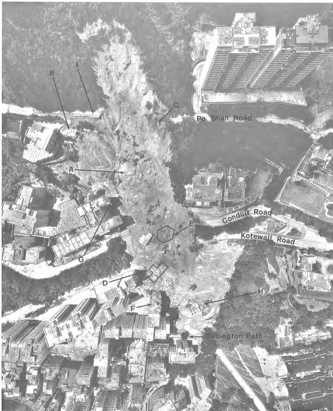
Plate 96. Large Scale Aerial Photograph of the Po Shan Road Landslip in 1972. Note the large block of rock, probably of volcanic origin at (A), the failure of the lawn and garage at 21 Po Shan Road (B), the vehicle below Po Shan Road (C), the location of Kotewall Court (D), the location of the four storey private dwelling at 11 Kotewall Road (E), the damaged portion of Greenview Gardens (F), debris around Skyline Mansions (G), and the debris around a structure under construction (H). The residents of 11 Kotewall Road (E) were evacuated following a landslip at about 5.00 p.m. on 18.6.1972, some 4 hours before the major failure. The building was apparently buried up to the 2nd Floor by landslip debris after the 5.00 p.m. failure, and the occupants escaped without injury. (Government of Hong Kong, 1972b). The boulder on Po Shan Road referred to in Plate 99 is at I. (20.6.1972/1650).
