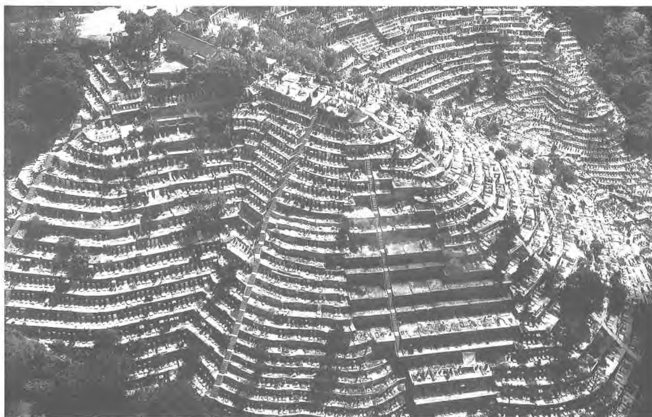
Plate 136. Oblique Aerial Photograph of Remedial Works to a Landslip in the Cemetery at Pok Fu Lam in 1981. A landslide resulted in the exhumation of more than 500 grave sites and illustrates in a dramatic manner, that it is not always possible to 'rest-in-peace' from the dangers of slope failure. (GCO/OAP/ 1981/PS230-2A)
