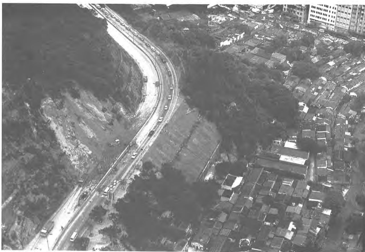
Plate 119. Oblique Aerial Photograph of Landslip on Ching Cheung Road in 1982. This photograph shows the disruption of the east bound carriageway above Wai Man Tsuen in Butterfly Valley. The landslide resulted from the failure of a large cut slope. (GCO/OAP/PS336-12A).
