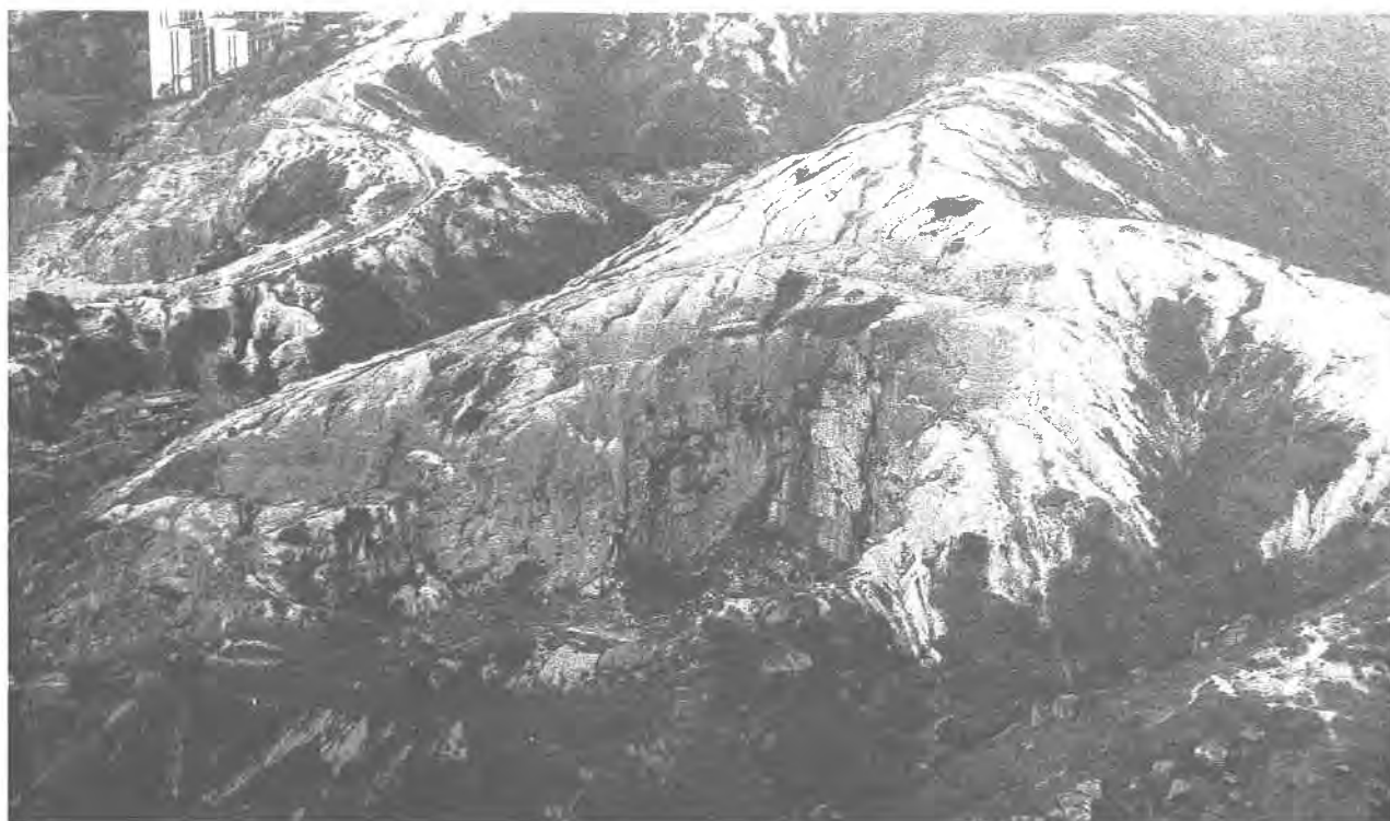
Plate 197. Oblique Aerial Photograph of Severely Eroded Granitic Terrain near Ngau Tau Kok in 1984. This photograph shows the severely eroded nature of the hillcrests which is characteristic of much of the granitic terrain in the Territory. Gully erosion originates almost at the crest of the ridges and spurlines on this type of terrain. (GCO/OAP/1985/PS525-5A).
