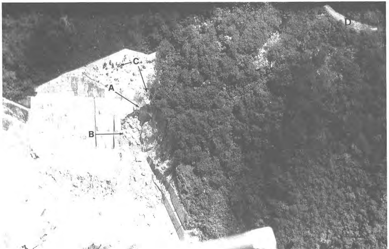
Plate 130. Oblique Aerial Photograph of Landslip at Ngau Chi Wan in 1979. Failure at A, of a cut slope, during site formation, in decomposed granite (B) and colluvium (C) is evident on a natural drainage line. A portion of Jats Incline is evident at D. (GCO/OAP 1979/PS55-23).
