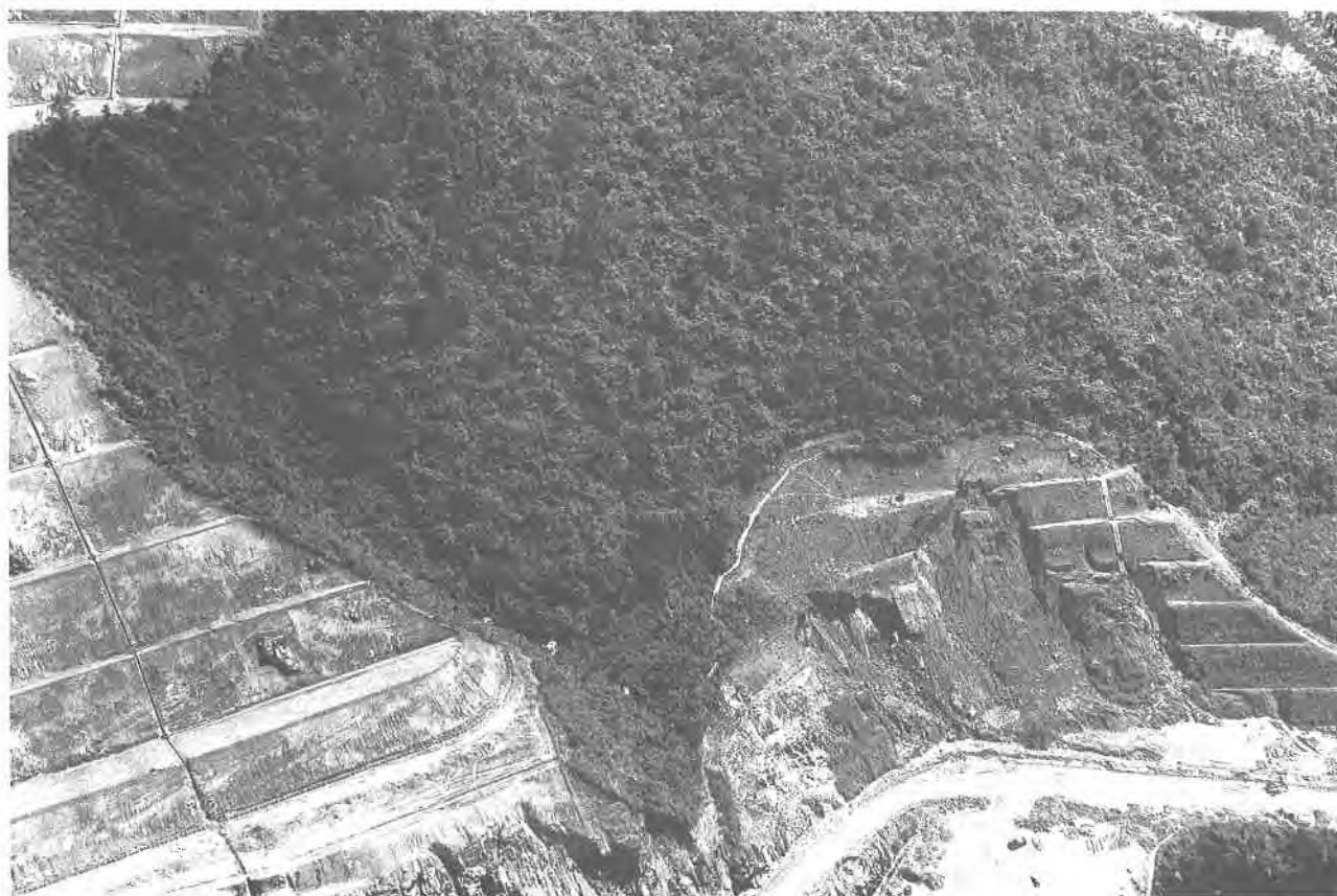
Plate 127. Oblique Aerial Photograph of Landslip at Kau Tau in 1979. Failure of a cut slope occurred in a borrow area near the Chinese University of Hong Kong. (GCO/OAP/1979/PS52–17).
