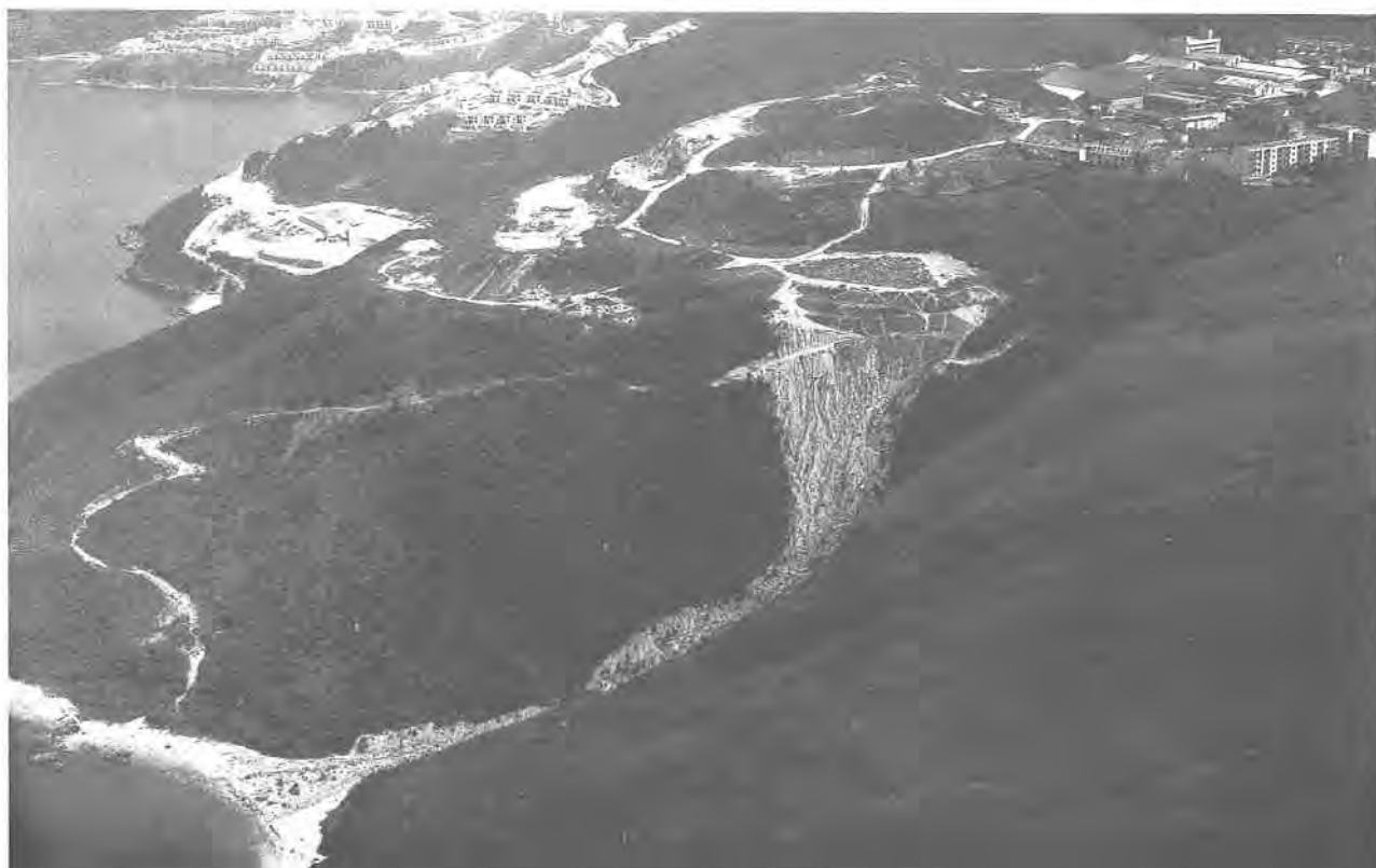
Plate 135. Oblique Aerial Photograph of a Severely Eroded Fill Slope in the Silverstrand Area in 1980. Severe gully and sheet erosion is evident on this large fill slope on the Clear Water Bay Peninsula. (GCO/OAP/1980/PS134-1).
