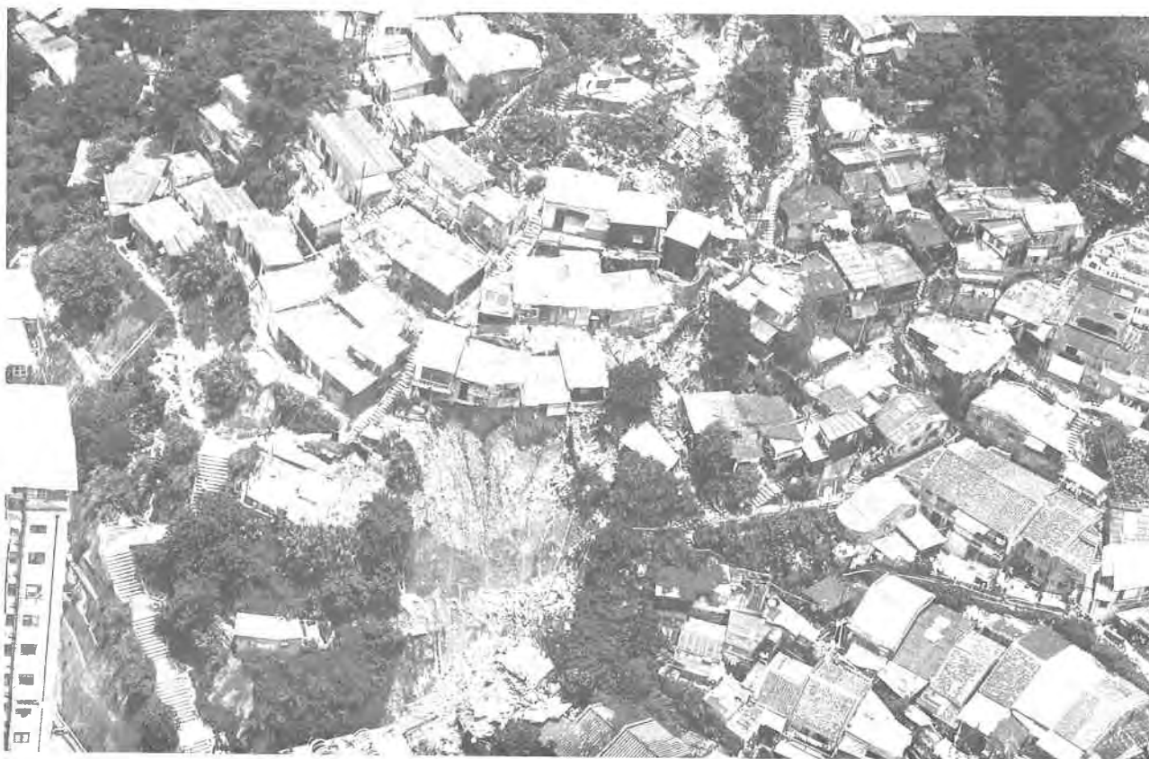
Plate 140. Oblique Aerial Photograph of Landslip at Tsin Shui Ma Tau in 1982. Slope failure occurred on a cut slope and affected squatter huts at the crest of the slope and a portion of a children's playground. Plate 139 provides detail of the failure viewed from the playground at the base of the slope. (GCO/OAP/1982/PS297-9).
