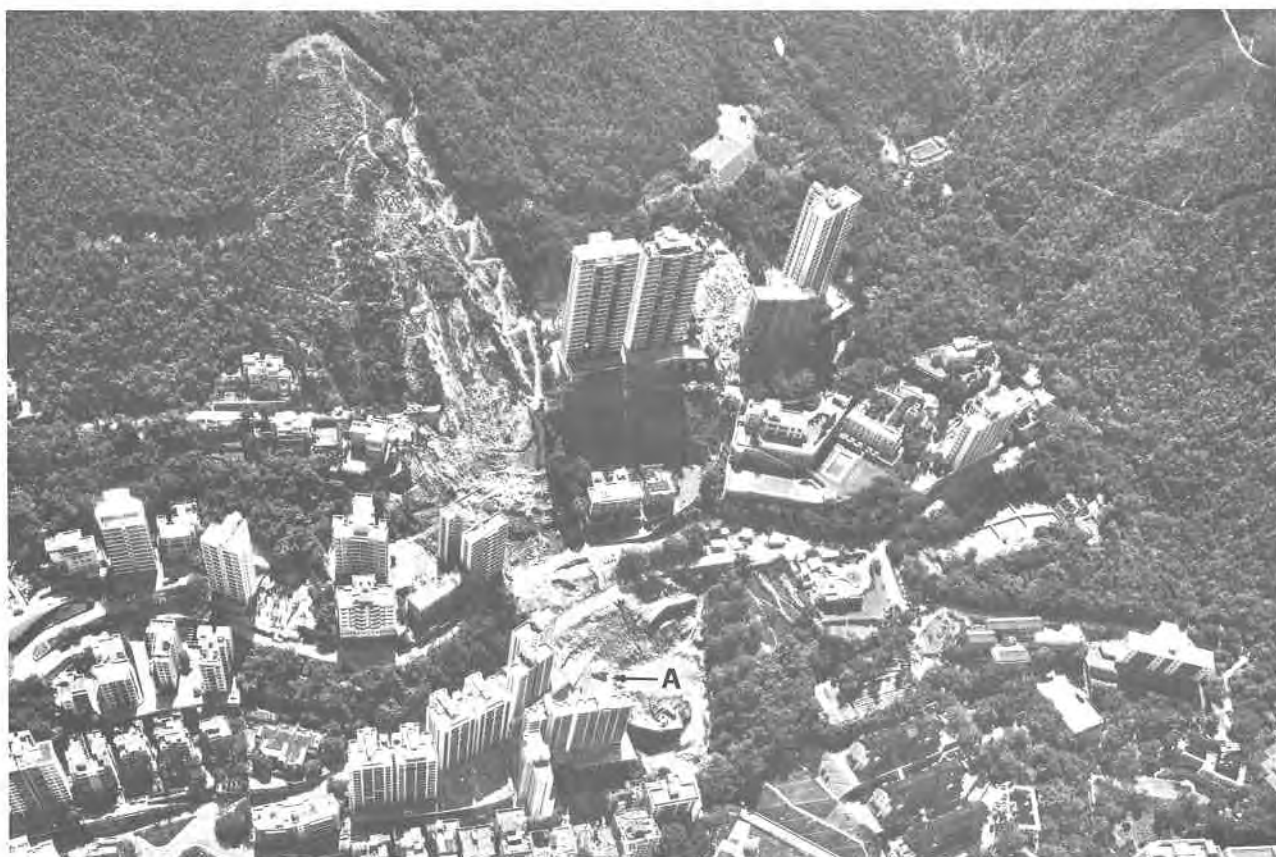
Plate 104. Oblique Aerial Photograph of the Po Shan Road Landslip Site in November 1972. This photograph was taken some 9.5 months after the failure; compare this with Plates 102 and 103. An access track to the upper portions of the landslide scar is apparent, and clearance work has progressed on the lower slopes. The damage to the upper storeys of Greenview Gardens (Plates 94 and 96) appears to have been repaired (A). (3.11.1972/2363).
