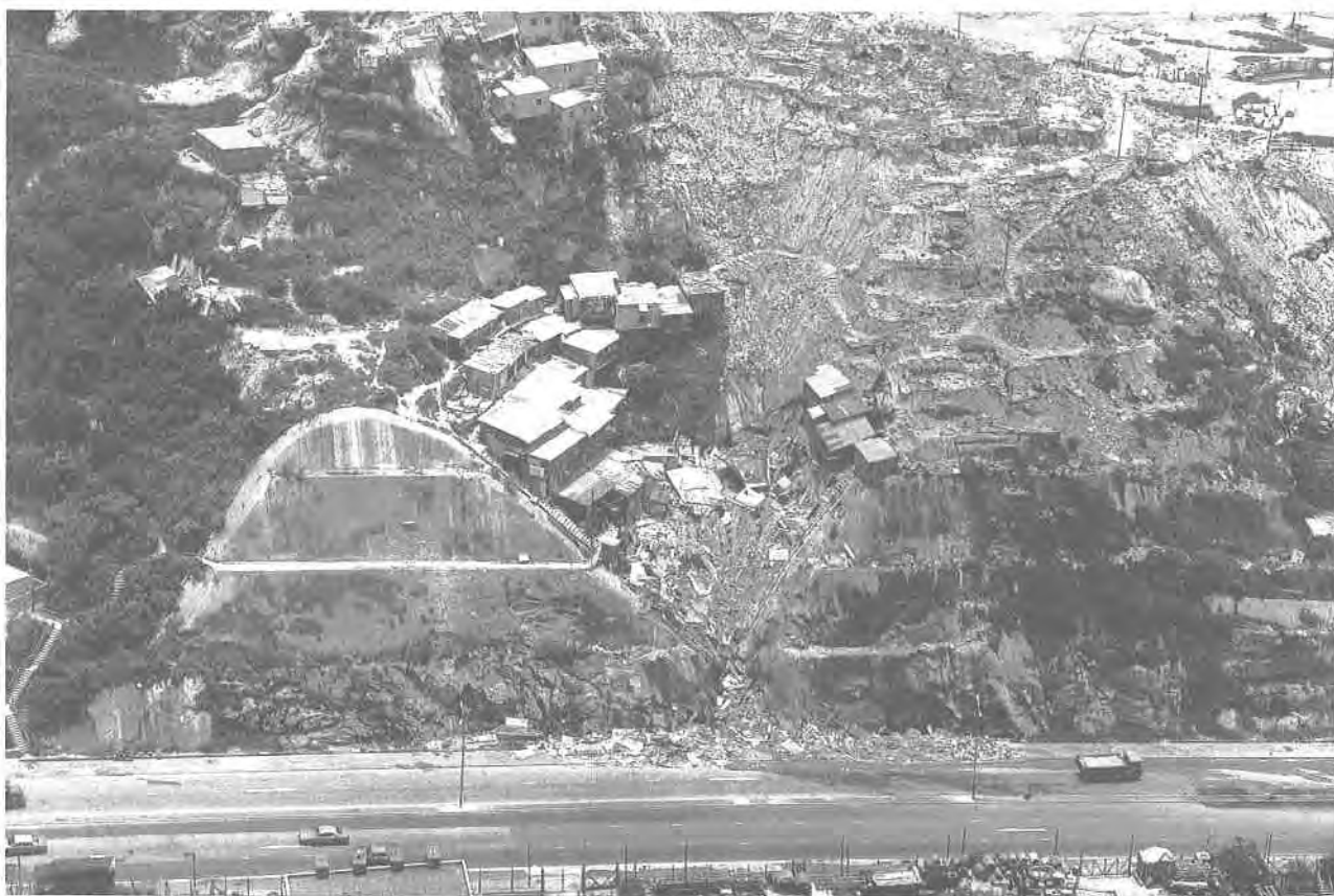
Plate 147. Oblique Aerial Photograph of Landslip in a Squatter Area at Lam Tin in 1982. A number of huts were destroyed by this failure above Junk Bay Road. (GCO/OAP/1982/PS297-5).
