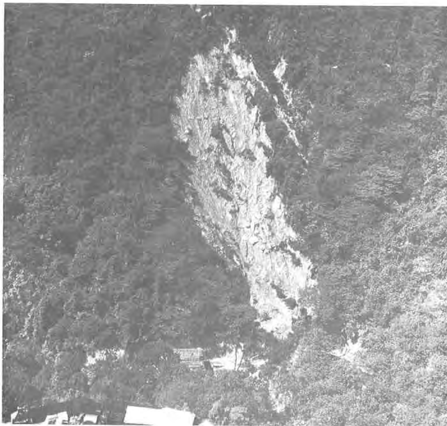
Plate 138. Oblique Aerial Photograph of Landslip near the Crow's Nest in 1981. This landslide occurred on natural granitic terrain in the vicinity of Beacon Hill, and is also shown in Plate 137. (GCO/OAP/1981/PS232-12).
