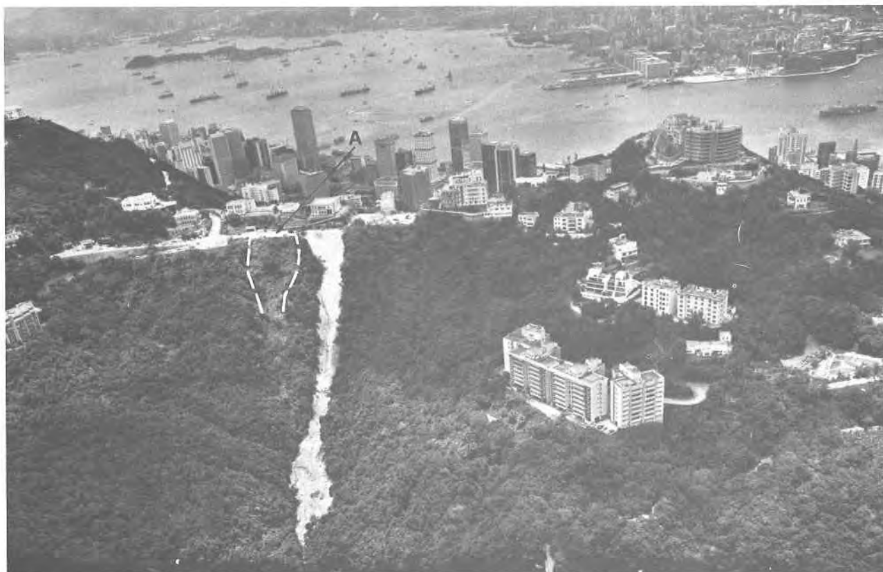
Plate 57. Oblique Aerial Photograph of Landslip on Peak Road in 1983. The area at A failed in 1966 and the incident is highlighted in Plate 58. Plate 153 provides a view of the 1983 failure from the carriageway. (21.6.1983/49230).
