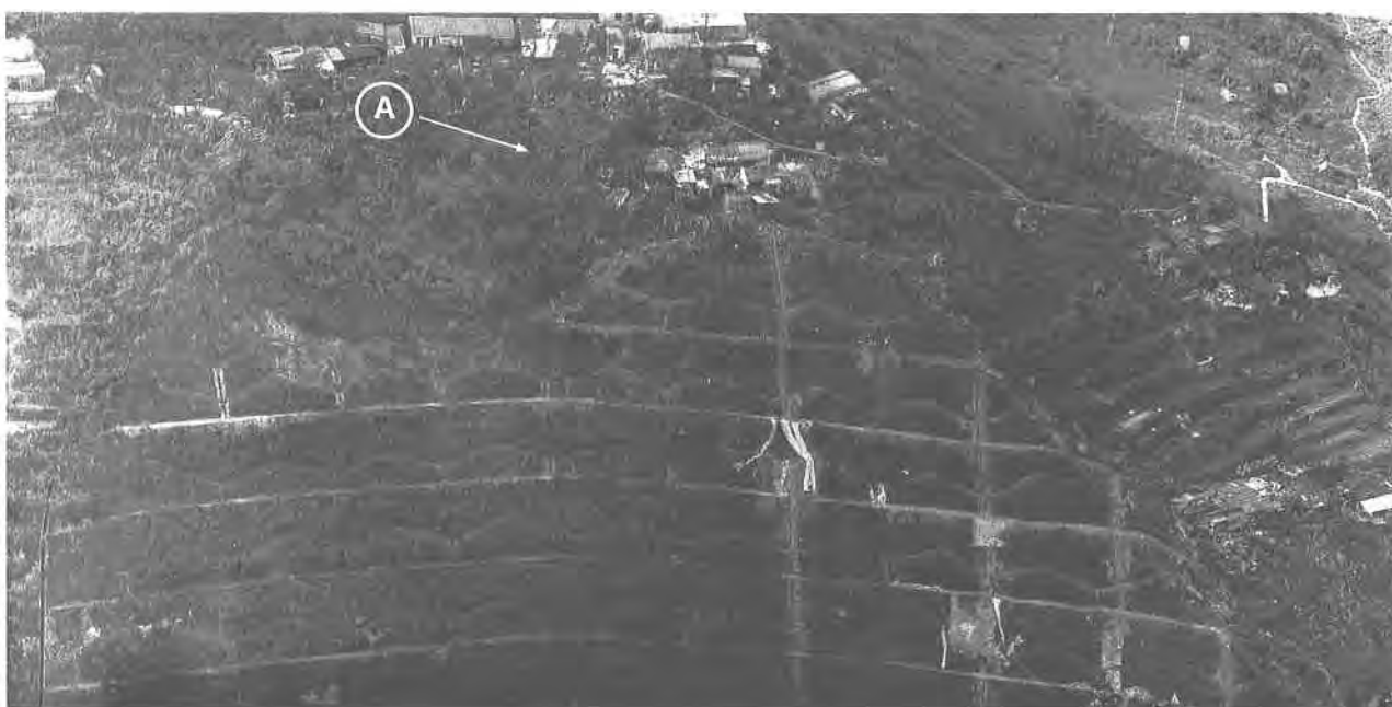
Plate 171. Oblique Aerial Photograph of Slope Failure on a Cut Slope at Pun Shan Tsuen in October 1983. Site investigation is in progress on the mid to lower portions of the cut slope following the slope failure shown in Plate 172. The general location of Plate 172 is shown at A. (GCO/OAP/1983/PS399-9).
