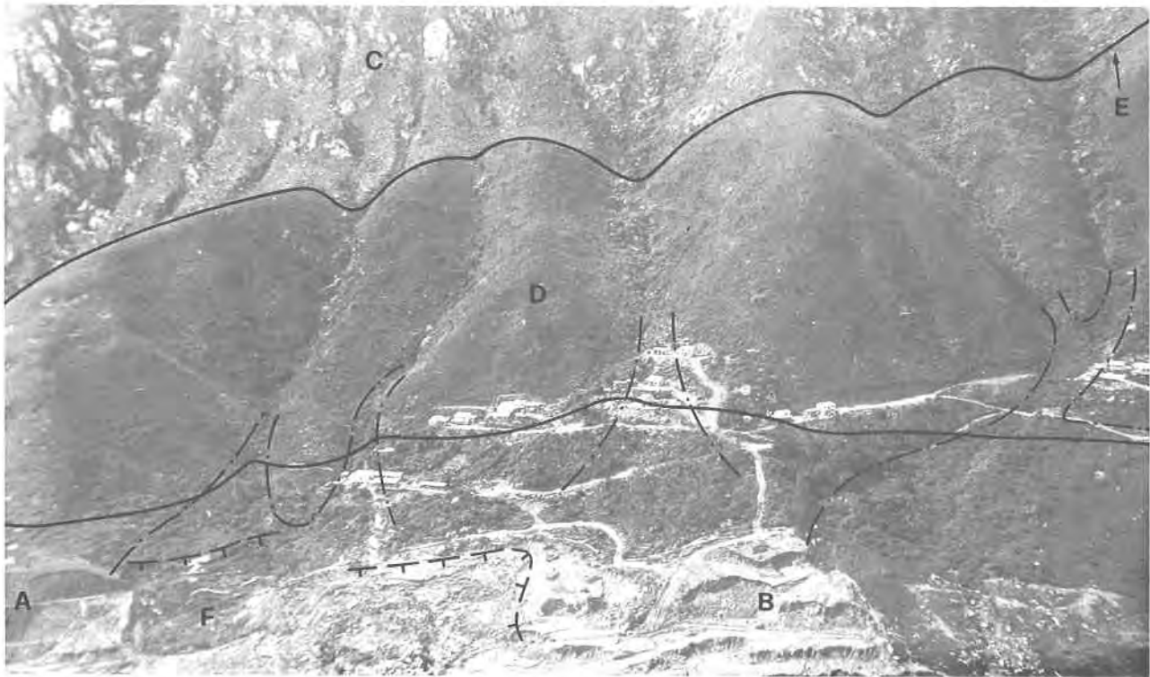
Plate 120. Oblique Aerial Photograph of Tuen Mun Borrow Area 19 in 1978. On the eastern slopes below Tsing Shan (Castle Peak), several areas of instability are associated with decomposed volcanic (A) and colluvial terrain (B). The upper slopes are formed of well-jointed granite (C) and decomposed metasediments (D), separated by a near-vertical fault (E). This Plate demonstrates the significance of the natural drainage pattern on instability. The zone of instability marked at F (shown in Plate 121) is within an area that receives discharge from the upper slopes. Numerous tension cracks are visible within the area. This view is to the west across the borrow area on 28.9.1978. The stereotriplet at Plate 122 shows the general nature of the terrain prior to development. (GCO/OAP/1978/PS9-1).
