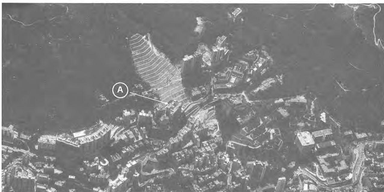
Plate 106. Oblique Aerial Photograph of Remedial Works to the Po Shan Road Landslip Site in February 1974. Reinstatement appears to be complete, with a large retaining wall behind Skyline Mansions (A). The new alignment of Conduit Road has been completed. Plate 117 shows the area in 1980. (28.2.1974/8264).
