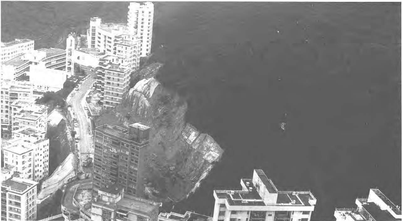
Plate 145. Oblique Aerial Photograph of Landslip in South Bay Close in 1982. The failure occurred in the upper 12 m of a slope under construction on 29.5.82, during heavy rain. More than 3 000 m 3 of debris was involved and affected much of the site for a multistorey residential block. The failure occurred along a pre-existing, persistent discontinuity some 700 mm thick in places. The infill material consisted of a 'gouge' of gravel sized fragments of volcanic rock in a silty matrix, with occasional bands and pockets of pink clay. After the failure, water flowed from the discontinuity at several points. Piezometers, read on a daily basis prior to the failure, did not confirm the existence of a perched water table. However, piezometer buckets were installed in existing standpipes after the failure, and readings taken during the August rainstorms in 1982 showed much higher water levels. The landslide occurred as a simple wedge failure along a pre-existing major discontinuity. (GCO/OAP/1982/PS286-8).
