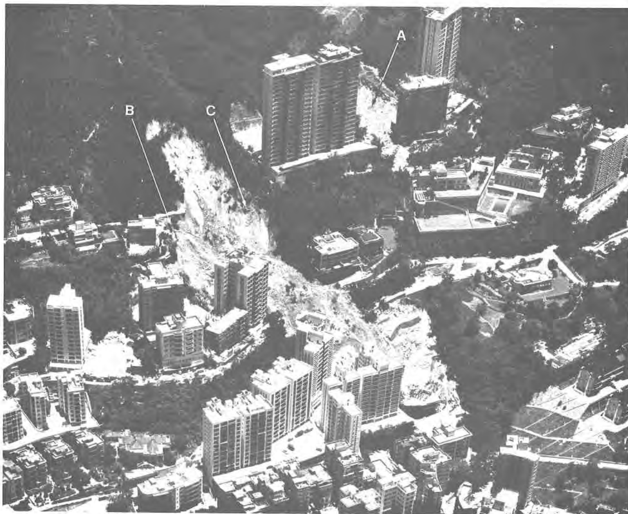
Plate 97. Oblique Aerial Photograph of the Po Shan Road Landslip Site in 1972. The plate provides a perspective of the disaster site from the northeast, some 6 days after the landslide. Note the large landslide behind the partially constructed Hamilton Court (A); the lawn and garage area at 21 Po Shan Road have collapsed (B); compare this with the photographs in Plate 94. The vehicle is still evident (C). The landslide on the slope behind Hamilton Court occurred on the morning of 16.6.1972, some 2 days before the major incident and blocked Po Shan Road (Government of Hong Kong, 1972b). (24.6.1972/1805).
