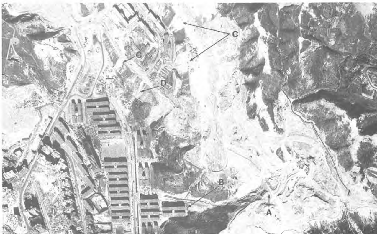
Plate 55. Enlargement to Accompany Stereopair of the Tsui Ping Road Area in 1964. This Plate accompanies Plate 56. Remedial works to the failure site are evident at A and debris is being removed from around the housing blocks at B. Landslips are evident to the north on newly formed slopes in the Sau Mau Ping Area (C), and a large gully is apparent on the fill slope at the site of the 1972 landslide (D). Compare this with Plates 107, 109 and 115. (13.12.1964/2539).
