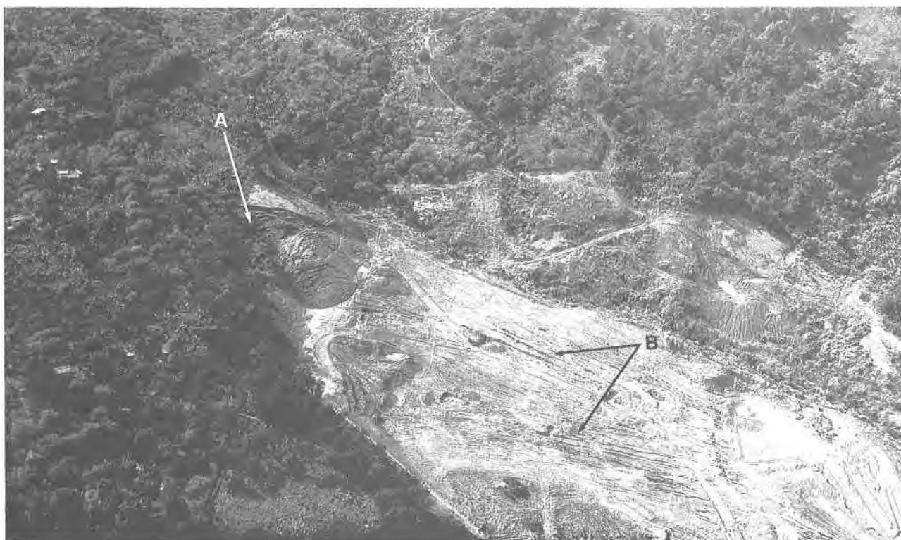
Plate 126. Oblique Aerial Photograph of Landslip in Tuen Mun Borrow Area 8 in 1978. A small landslide (A) occurred during site formation on deeply weathered volcanoclastic rocks. Severe erosion and soil tunnelling are also generally evident on the cut slope at B. Unlike Borrow Area 19 (Plates 120–124), colluvial deposits did not blanket the site prior to construction (GCO/OAP/1978/PS3–9).
