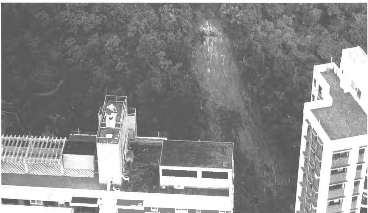
Plate 146. Oblique Aerial Photograph of Landslip above Kennedy Road in 1982. Failure occurred on the hilly terrain south of Wan Chai. (GCO/OAP/1982/PS260-23).
