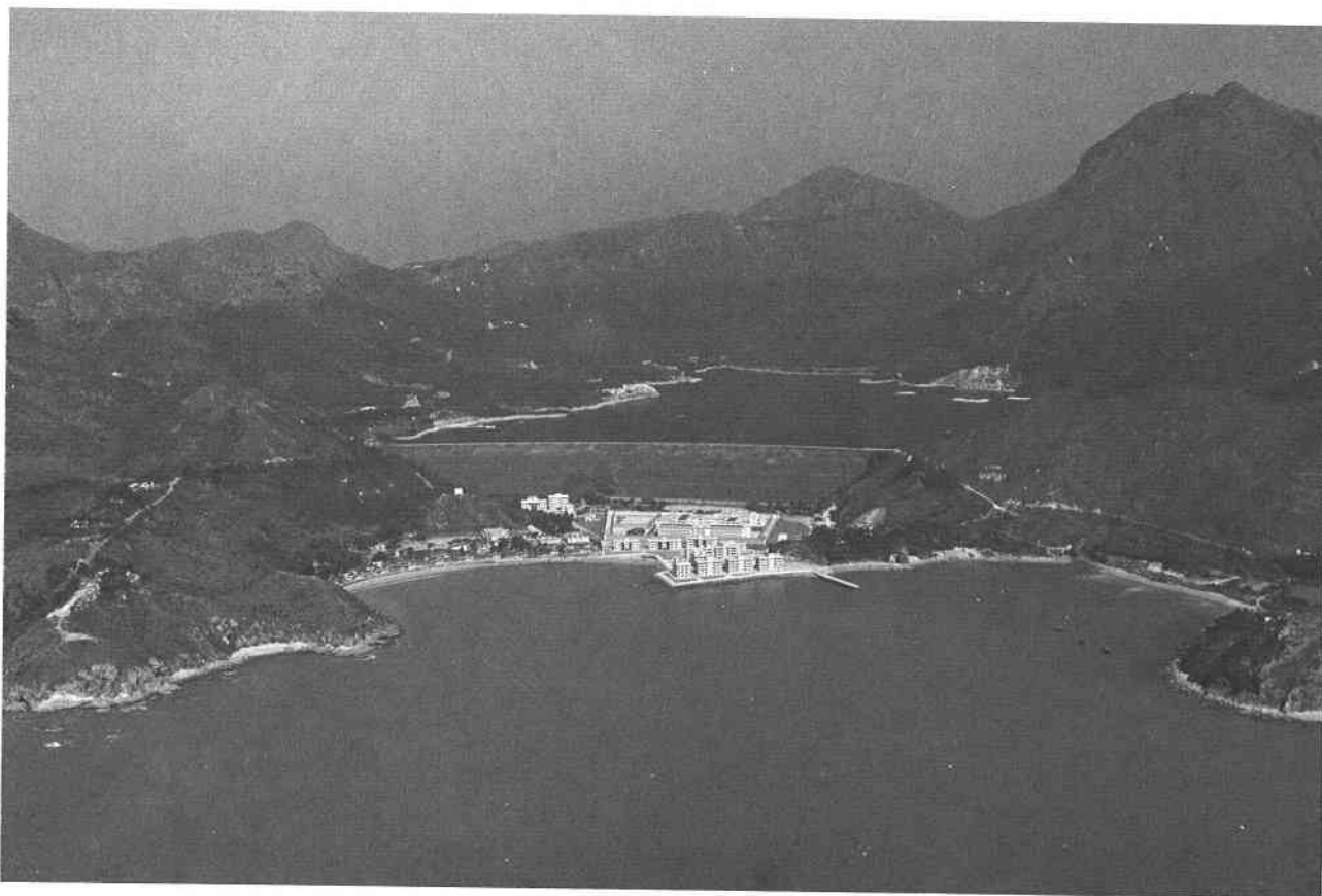
Plate 16. Oblique Aerial Photograph of Shek Pik Reservoir and the Surrounding Terrain. Disused quarry slopes form areas of bare soil and rock around the margins of the reservoir. Many of the steep sideslopes are prone to landslips. (GCO/OAP 1984/11034).
