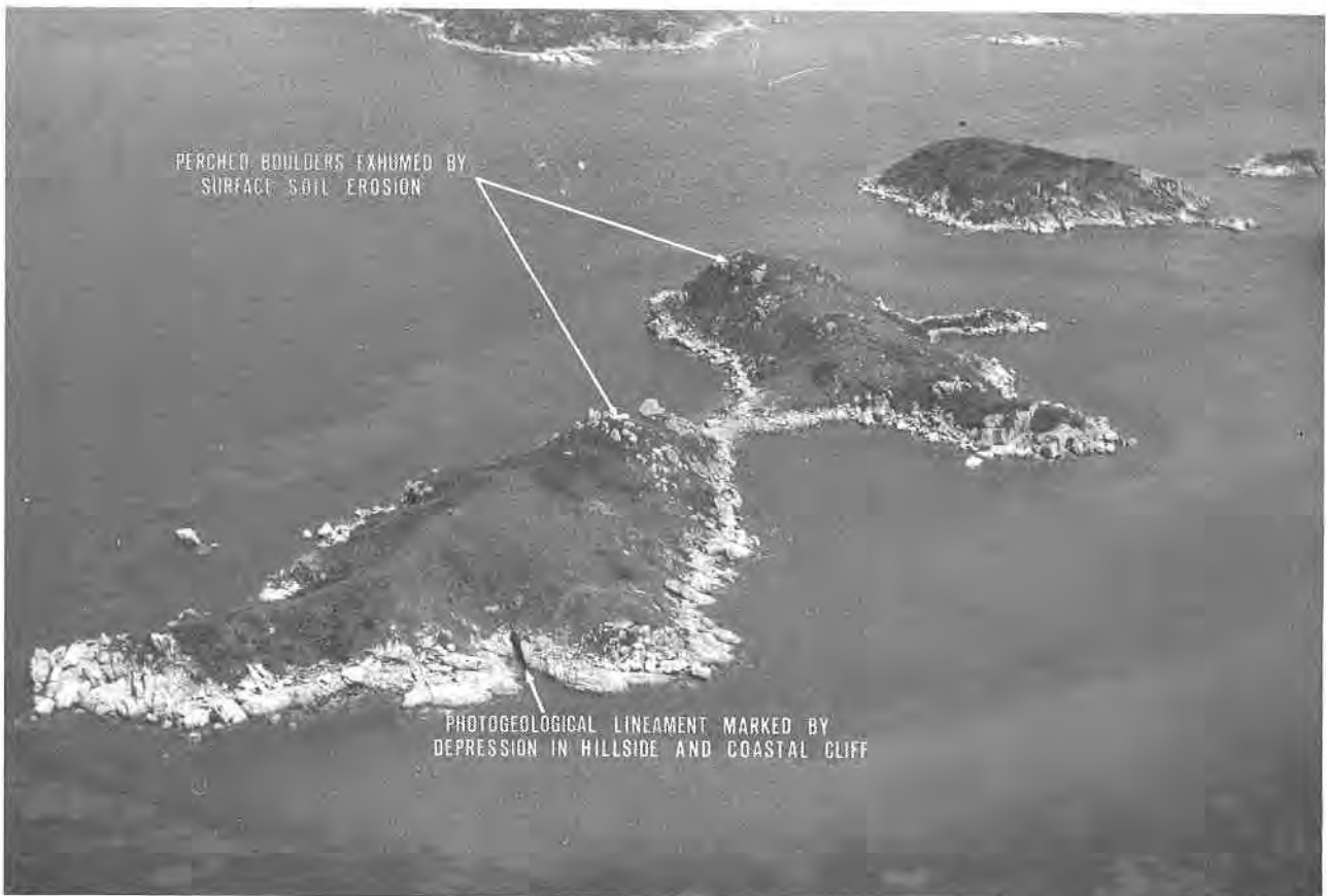
Plate 7. Oblique Aerial Photograph of Ma Chau and Yuen Chau (Soko Islands) . These uninhabited islands are composed of the well-jointed Fan Lau Porphyritic Granite. (GCO/OAP 1984/10802).
