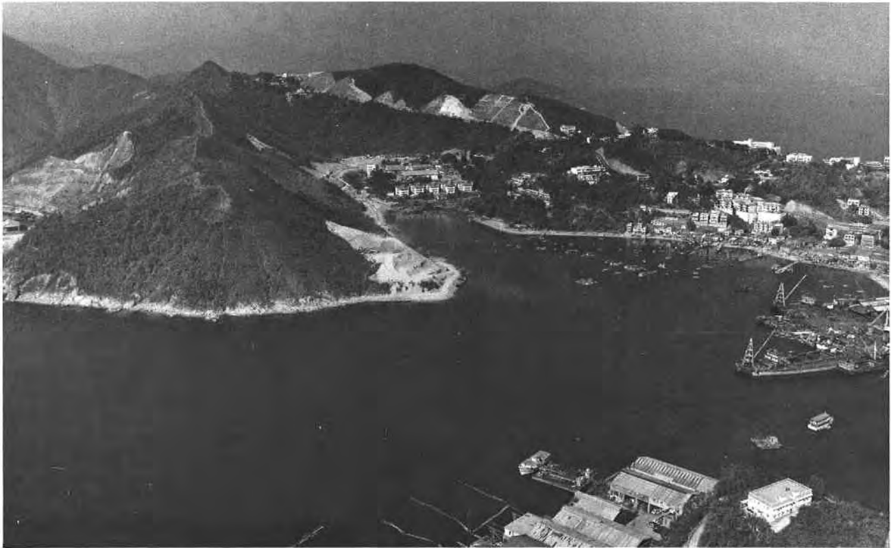
Plate 9. Aerial View of Junk Bay Around Hang Hau Village. This photograph was taken in January, 1984 and shows the coastline with only small areas of reclamation, much larger areas will be reclaimed as part of the Junk Bay New Town. The high cut slopes along the Clear Water Bay Road are evident in the background. (GCO/OAP 1984/10042).
