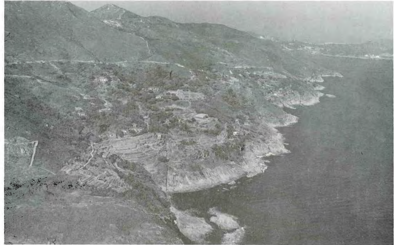
Plate 1. Aerial View of the West Coast of Junk Bay. Gently to moderately sloping midslope terrain may be suitable for development. Note the geological photolineament in the coastal cliffs passing inland along a colluvium-filled depression. The upper slopes show numerous perched boulders. (GCO/OAP 1984/10026).
