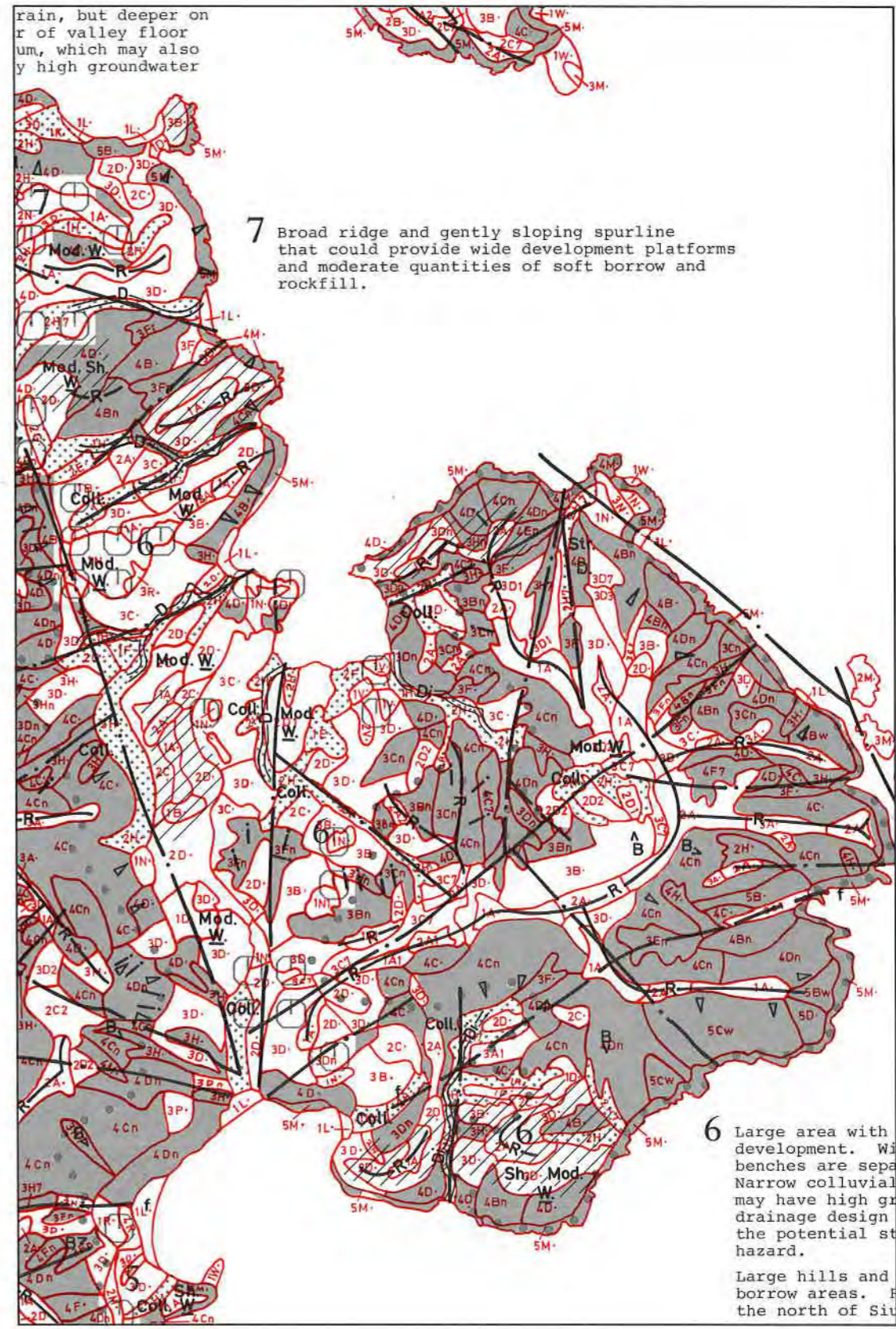
Scale 1:20 000 Example of the Terrain Classification Map Superimposed on the GLEAM Fig. 18b
