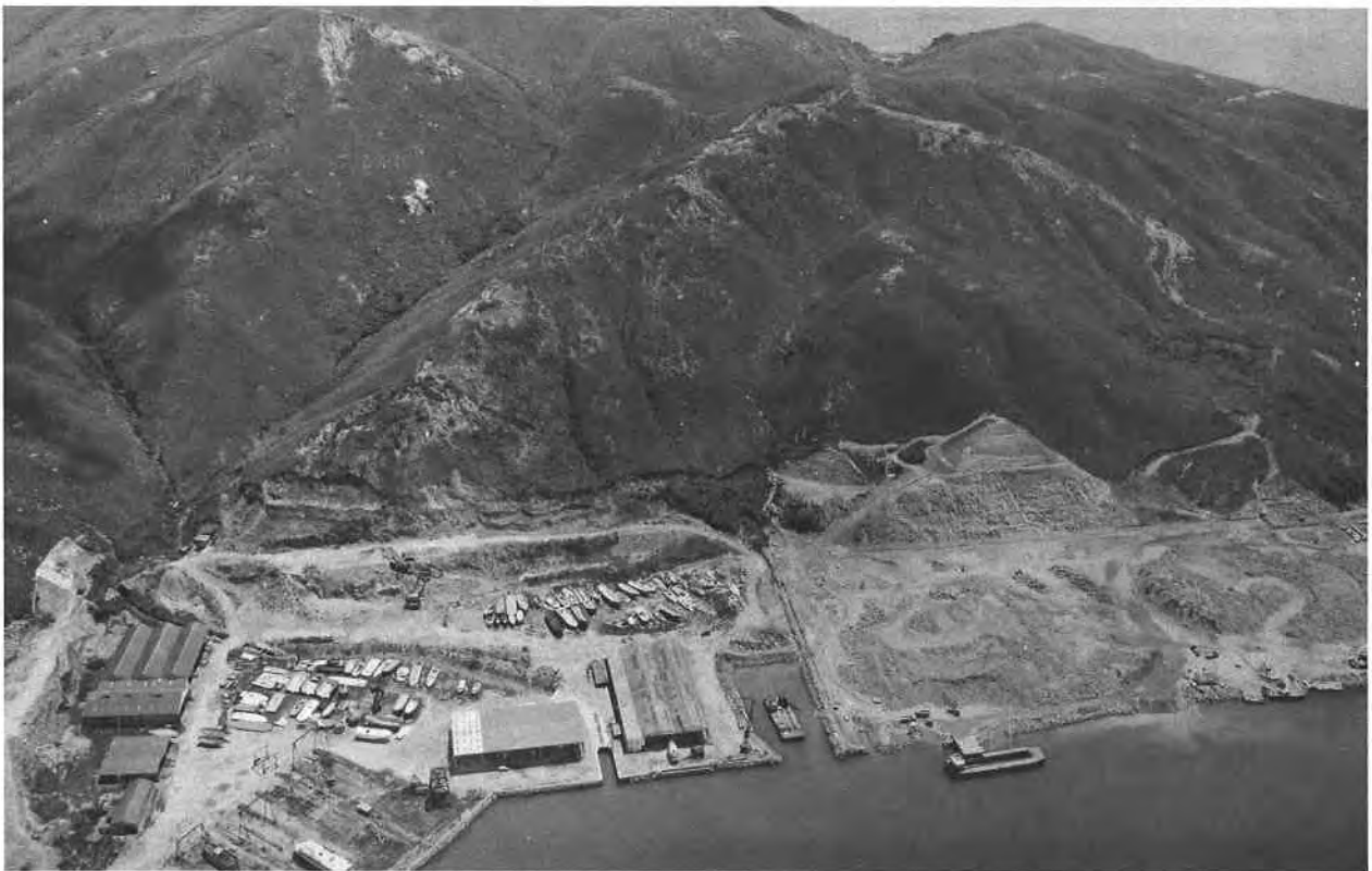
Plate 16. Oblique Aerial Photograph Looking Eastwards across Penny's Bay towards the Steep Granitic Terrain of Northeast Lantau. Note the gully erosion and instability associated with the ridgelines and steeper sideslopes (GCO/OAP 1981/5204).
