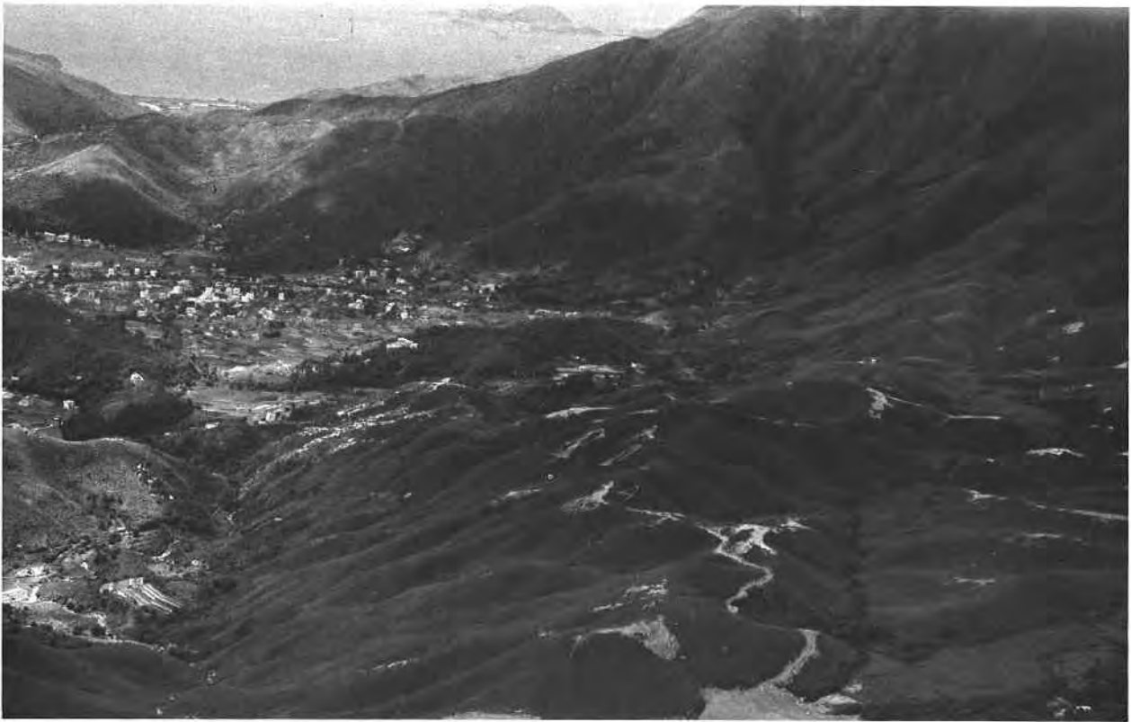
Plate 7. Oblique Aerial Photograph Looking West across Mui Wo Towards Pui O. In the foreground the low, undulating relief is typical of the decomposed granite whilst in the background the steep terrain is composed of volcanics. Colluvial deposits occur on the footslopes and within the drainage lines associated with volcanic terrain. (GCO/OAP 1981/5316).
