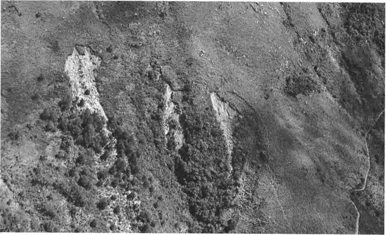
Plate 9. Well-defined Natural Landslips in Colluvial Materials on the Pat Sin Range. The colluvium is essentially volcanic derived in this locality (GCO/OAP 1981/1324).
