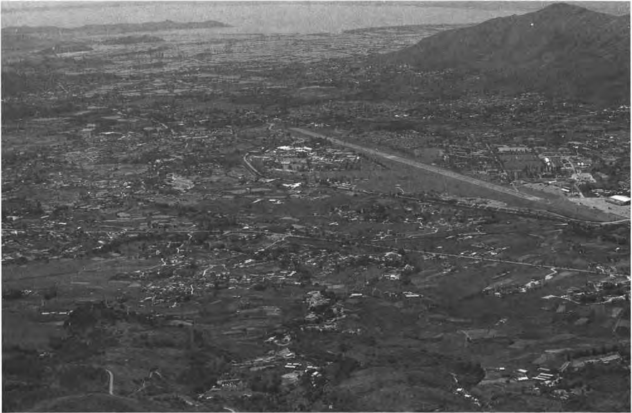
Plate 9. Oblique Aerial Photograph Looking Northwest along Shek Kong Valley towards Tsim Bei Tsui. Deposits of raised alluvium form the gentle slopes of the foreground, with low-lying floodplains bordering the streams in the centre of the Plate. (GCO/OAP 1980/3764).
