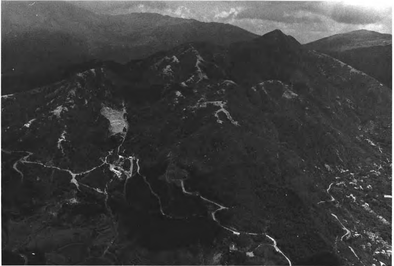
Plate 12. Ridgecrest Erosion on the Needle Hill Granite. The Needle Hill Granite is less susceptible to erosion than other coarser—grained granites in Hong Kong. The resultant topography is correspondingly less rounded with moderately steep sideslopes. Gully erosion, occasionally severe, is generally confined to ridgecrests and spurlines. (GCO/OAP 1981/4897).
