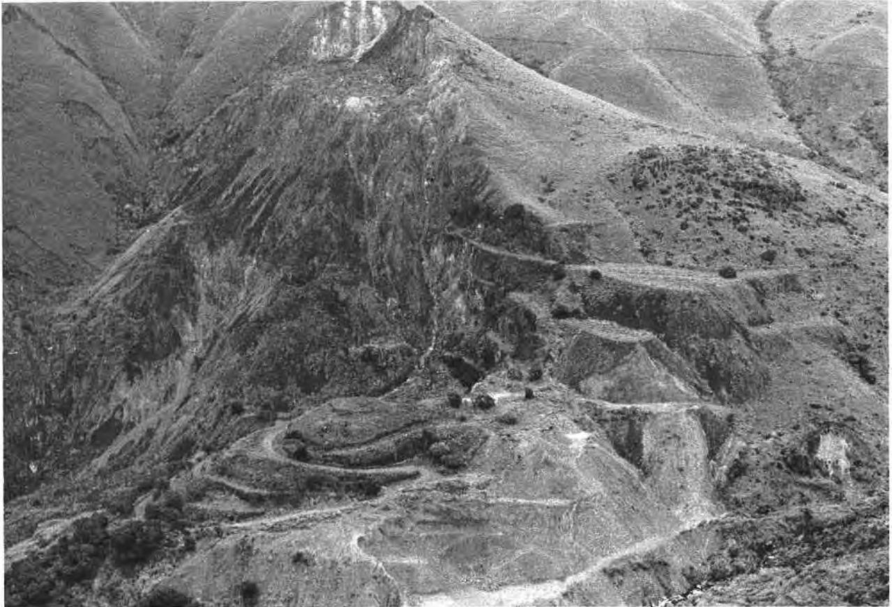
Plate 18. Unstable Terrain Associated with the Mine near Ma On Shan. A very large, well-defined landslide is evident in the middle-left of this Plate. The workings at the now abandoned mine probably caused the slope failure. Extensive mine tailings are evident at bottom of the Plate. These superficial deposits (man-made) are probably poorly compacted. Both the above features constitute significant geotechnical constraints for future development. (GCO/OAP 1982/7452).
