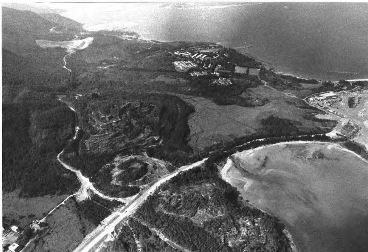
Plate 17. Alluvial Fan and Deltaic Deposits at Wu Kai Sha. The area is part of the Ma On Shan New Town Development. Recent alluvial sands and gravels overlying older clays silts and sands predominate in these flat-lying superficial deposits. Some interdigitation of these materials with colluvial fan deposits is expected on footslope and drainage plain terrain in the middle-left of the Plate. (GCO/OAP 1983/9000).
