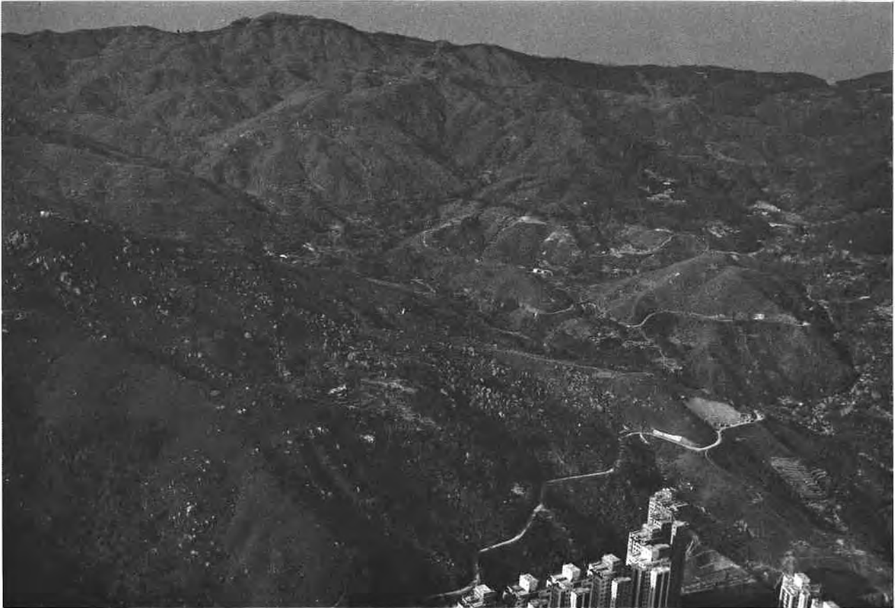
Plate 11. Dissected Upland Terrain and Boulder Strewn Sideslopes Northwest of Tsuen Wan. Predominantly coarse-grained pyroclastic rocks and coarse tufts of the Repulse Bay Formation are shown in this Plate. Numerous large residual corestones and tors at bottom-left indicate the presence of the Repulse Bay Formation Agglomerate. These boulders may influence future developments down slope. The extensive valley floors and footslopes are liable to flood during storm periods. Stream entrainment, infilling and platforming may render these lowerlying areas suitable for development. (GCO/OAP 1980/2866).
