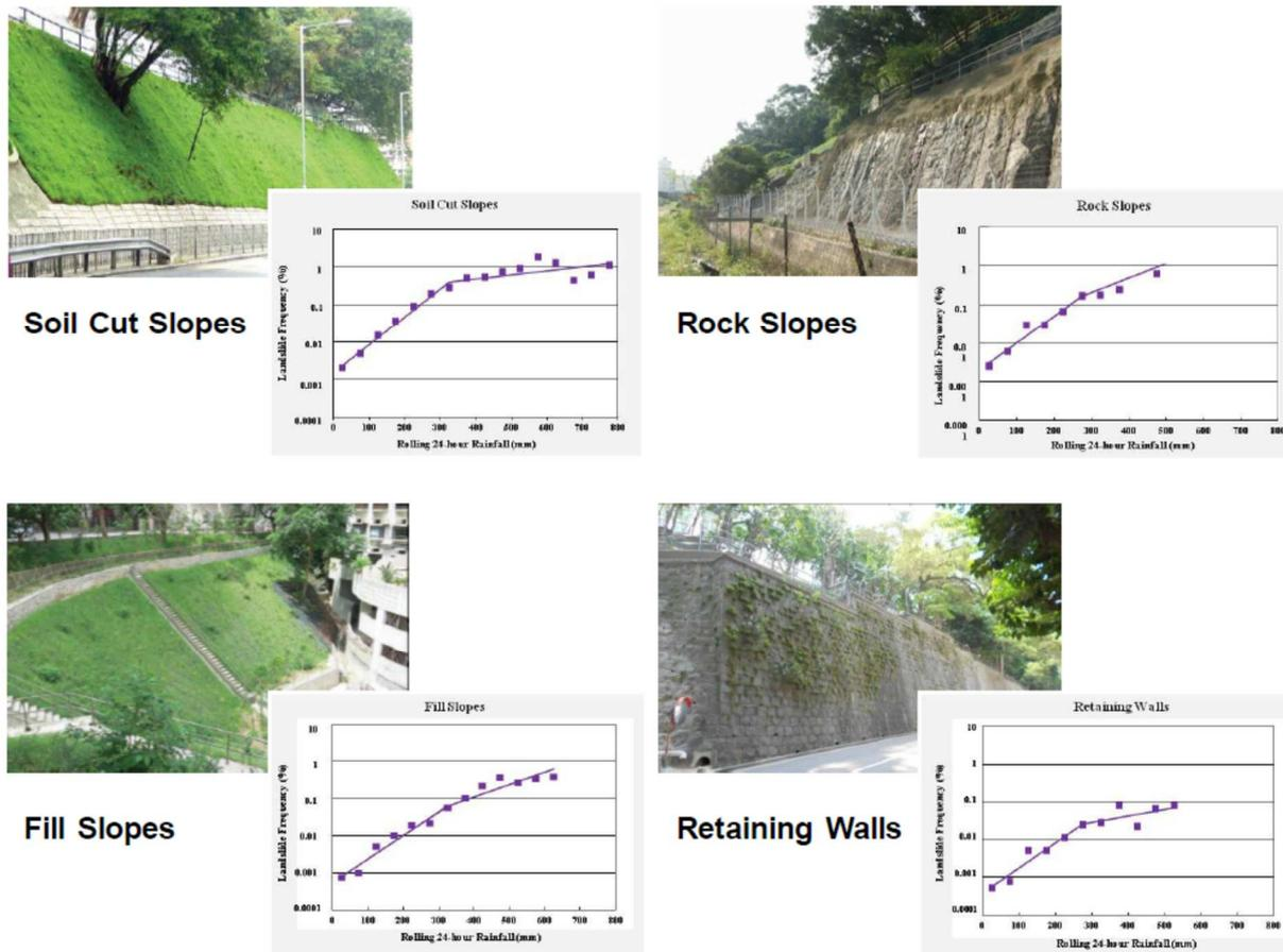
Figure 1. GEO's landslide-rainfall correlations for slopes and retaining walls.
