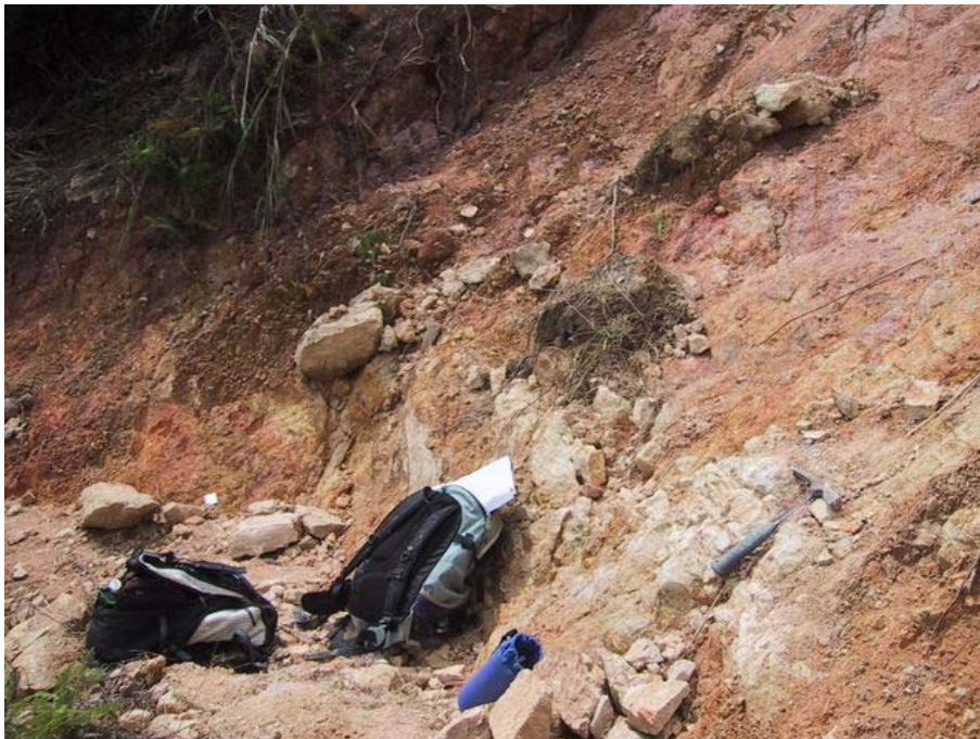
Plate 10 - View of Break in Slope Within the Source Area (Roughly parallel to the band of lighter rock (MT6) found high in the source area. Photograph taken on 16 May 2003)
