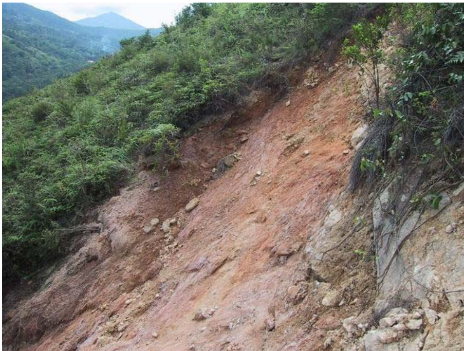
Plate 8 - View of the Western Flank of the Source Area (Relatively clean surface of rupture with overlying colluvium exposed at the scarp. Photograph taken on 16 May 2003)
