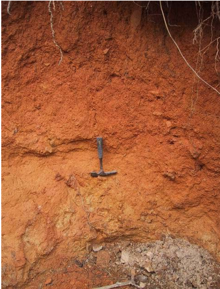
Plate 25 - View of the Failure Eastern Flank of the Drainage Line at Chainage CH 88 (Hammer denotes the contact between colluvium and completely decomposed coarse ash tuff. Photograph taken on 16 May 2003)
