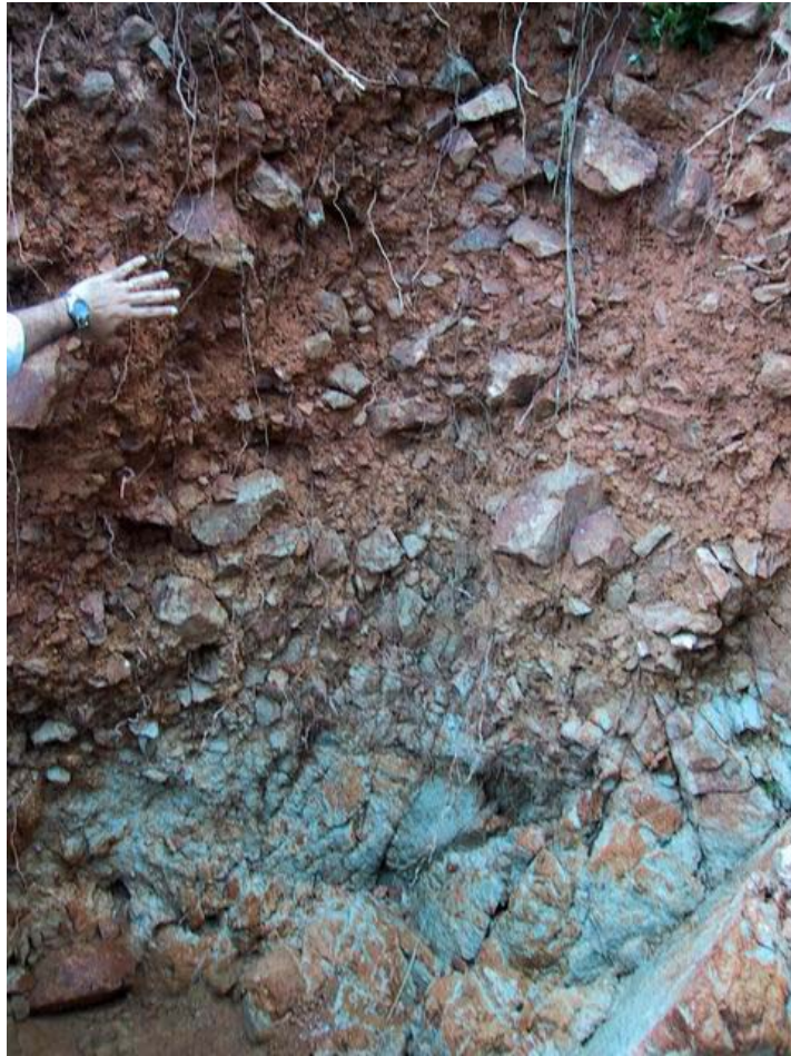
Plate 27 - View of Colluvium Overlying Insitu Metamorphosed Siltstone at Chainage CH 120 (Photograph taken on 9 May 2003)
