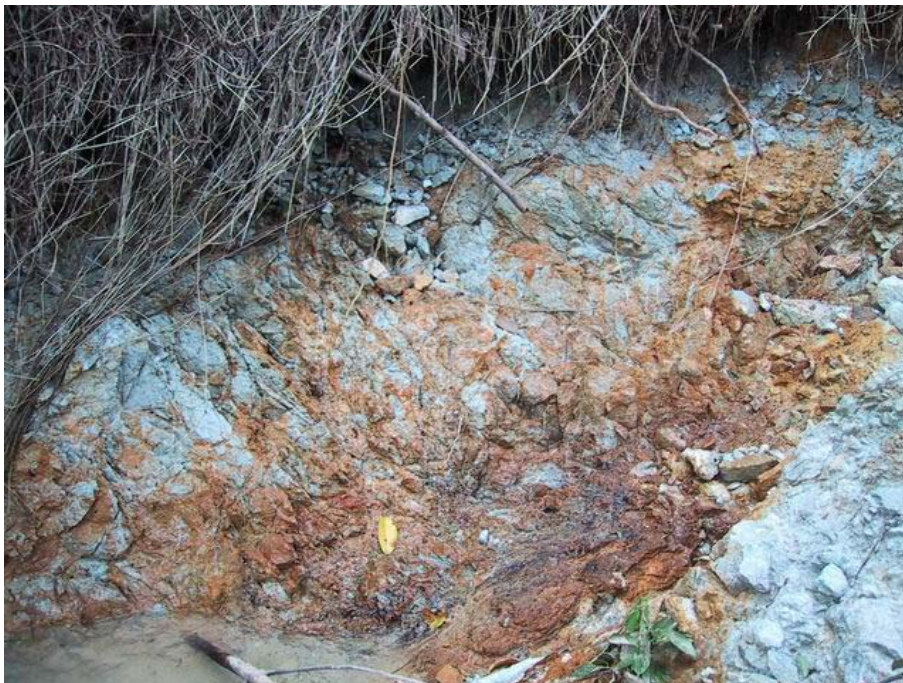
Plate 36 - Insitu Decomposed Coarse Ash Tuff Found within the Drainage Line/Debris Trail Near the Toe of the Landslide at Chainage CH 135 (Photograph taken on 9 May 2003)
