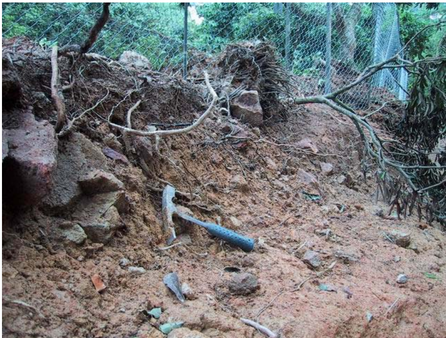
Plate 30 - Close-up View of Colluvium Exposed at the Flanks of the Drainage Line at Chainage CH 125 (Photograph taken on 9 May 2003)
