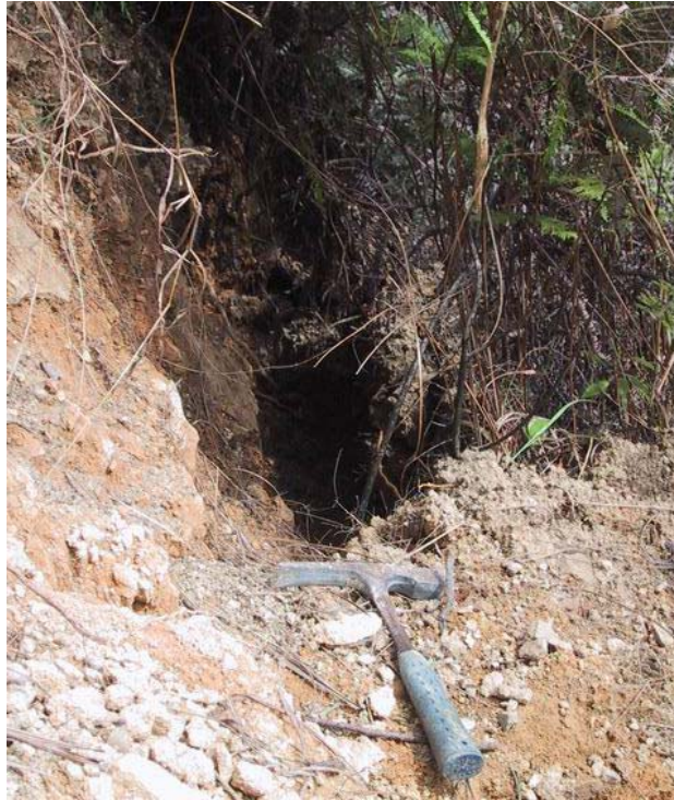
Plate 13 - View of Tension Crack on the Eastern Flank of the Source Area (Photograph taken on 16 May 2003)
