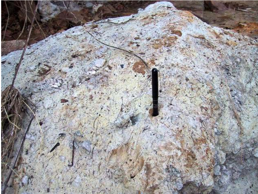
Plate 35 - Decomposed Coarse Ash Tuff With Kaolin Rich Matrix Found Near the toe of the Debris Trail (Photograph taken on 9 May 2003)
