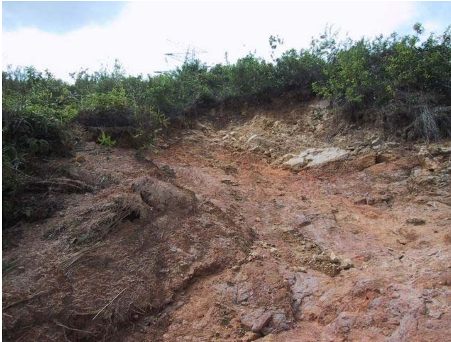
Plate 5 - View of the Western Portion of the Main Scarp (Note the lithology change - HDV/MDV with overlying metamorphosed siltstone. Photograph taken on 9 May 2003)
