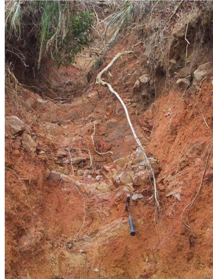
Plate 22 - View of the Incised Gully Near the Access Road (Insitu MDT and CDT exposed within the gully with colluvium exposed at the flanks. Photograph taken on 16 May 2003)
