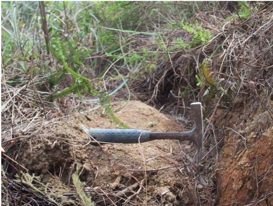
Plate 14 - View of Tension Crack on the Western Flank of the Source Area (Photograph taken on 16 May 2003)
