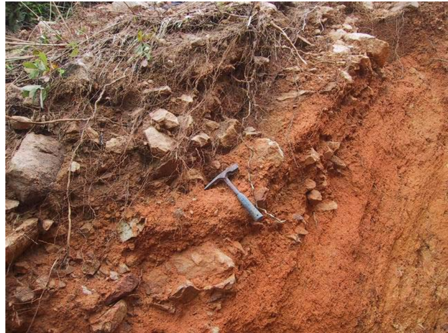
Plate 26 - View of Varying Ages of Colluvium at the Western Flank of the Failure within the Drainage Line at Chainage CH 88 (Photograph taken on 16 May 2003)
