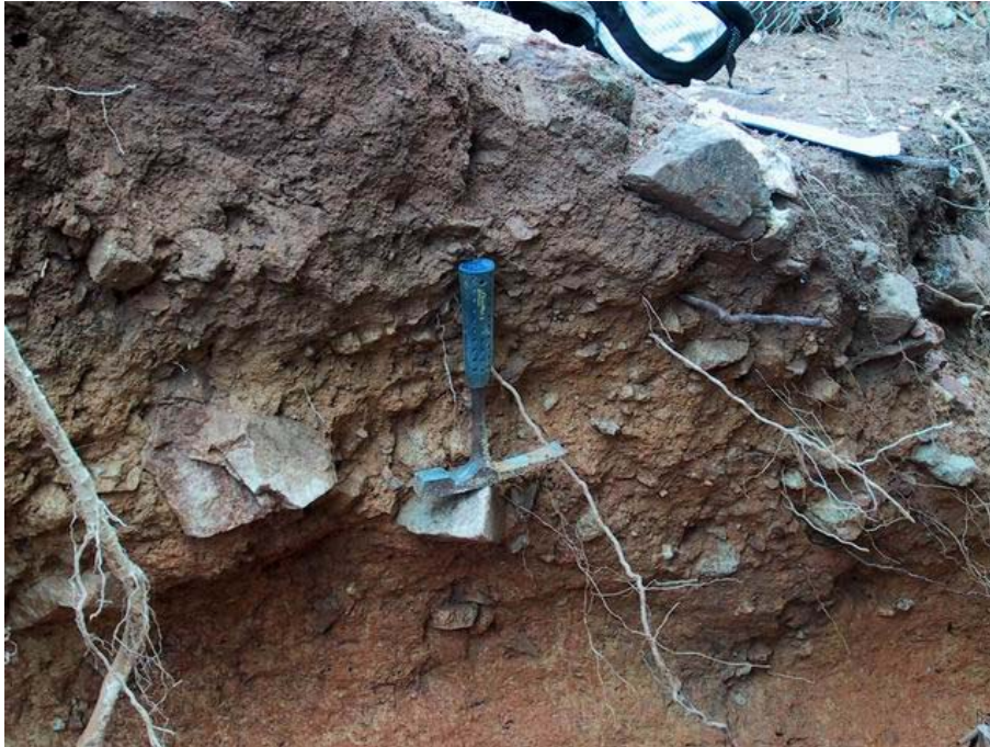
Plate 29 - Close-up View of Colluvium Within the Incised Gully at Chainage CH 123 (Photograph taken on 9 May 2003)
