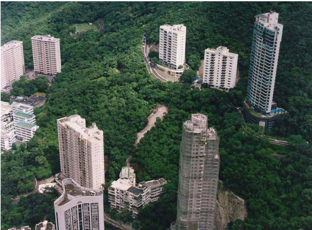
Figure 5.14 - A 20 m 3 Landslide in 1998 Resulted in Damage to Property
