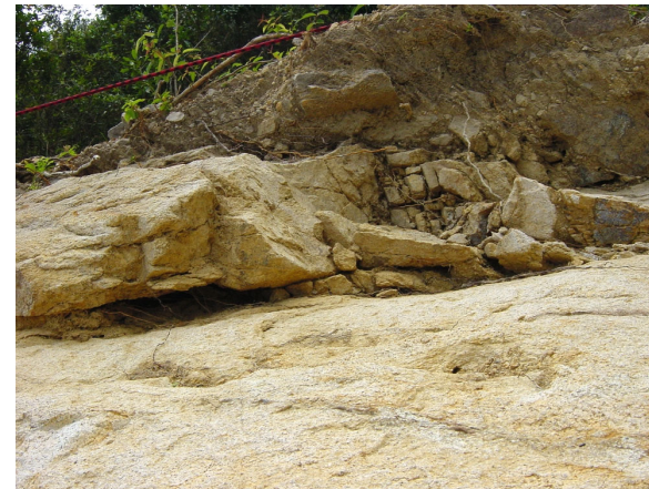
(d) Landslide along joint planes in weathered rock
