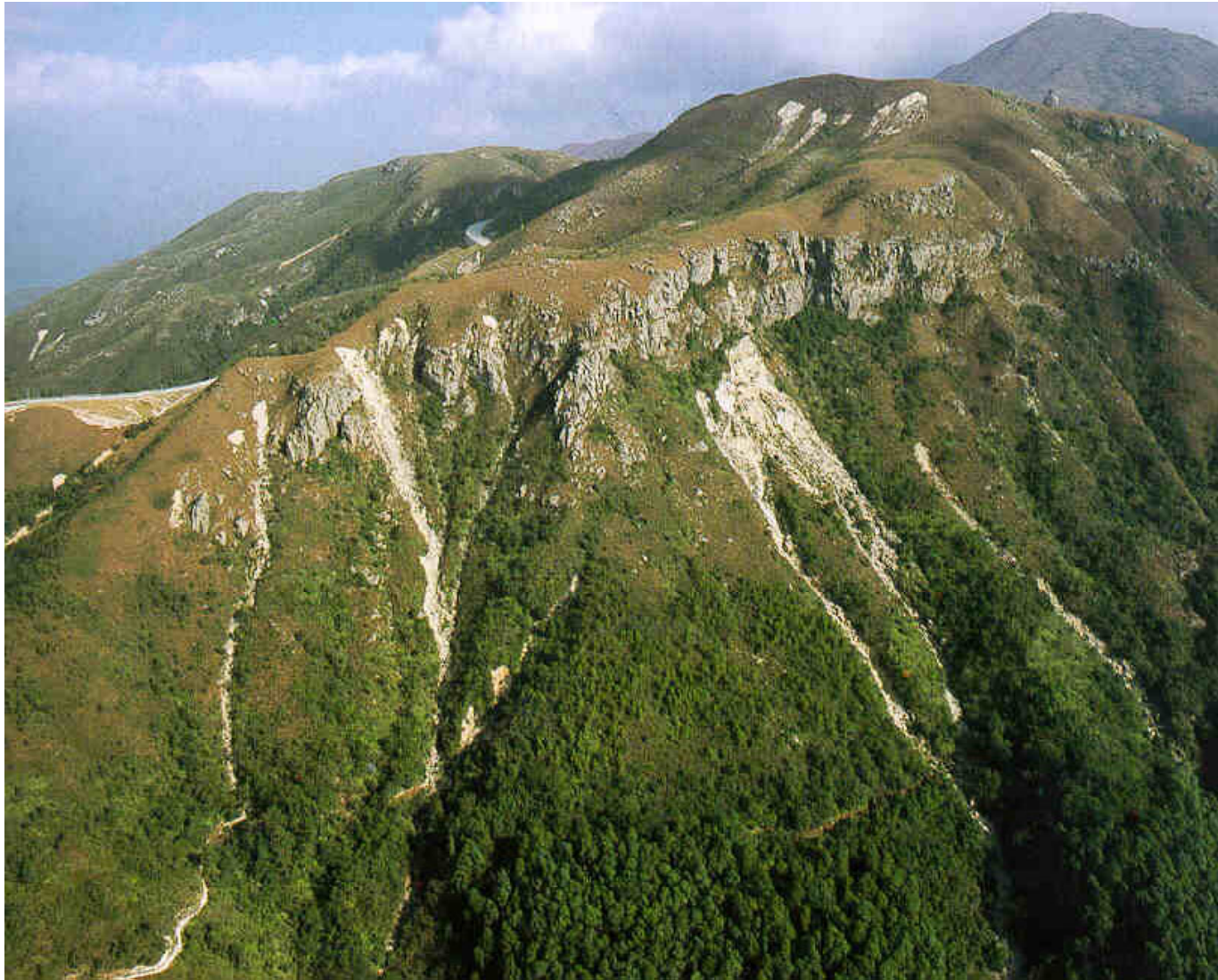
Figure 3 - Rain-induced Shallow Natural Terrain Landslides
