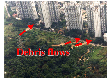
Plate (c) - Debris flows reached the access road to the housing estate
