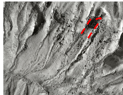
Plate (c) - 1963 aerial photograph showing a large relict landslide near the existing Tung Chung Road
