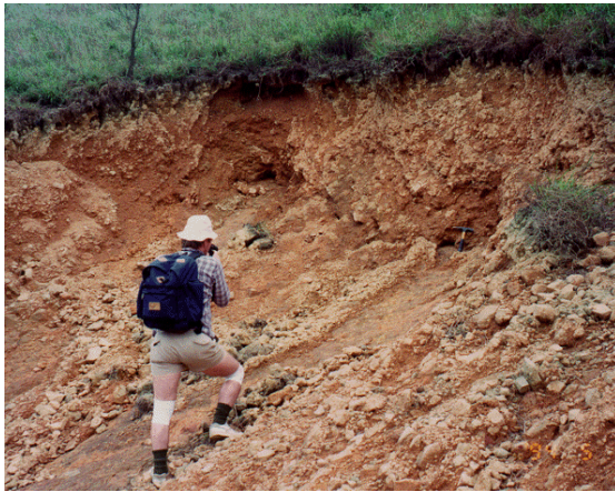
(a) Landslide in colluvium, above the interface with weathered rock
