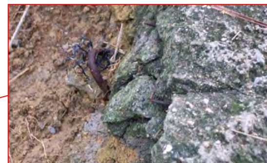
Plate 6 - View of Remnants of Erosion Control Mat around the Crest of the 5 May 2003 Landslide Site (Photograph taken on 14 June 2003)
