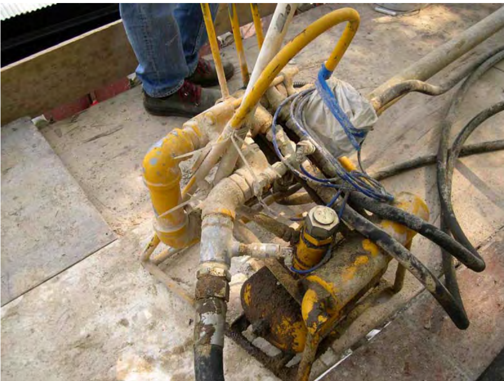
Plate 6 - Sensors Installed onto the Manual Control Panel
