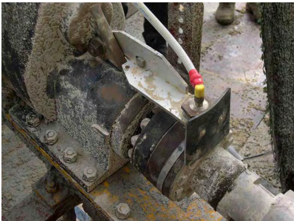
Plate 4 - Sensor for the Measurement of Rotation Speed
