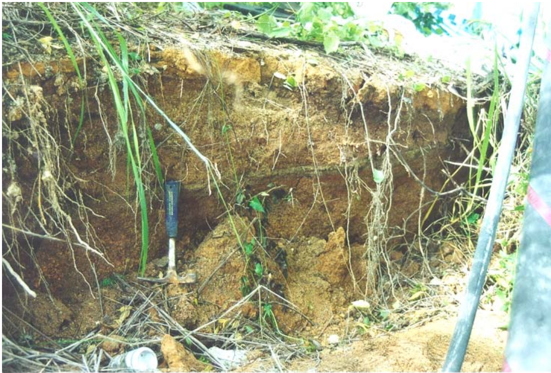
Plate 7 - Main Scarp at the Northern Distressed Zone (Photograph Taken by Hong Kong Geological Survey on 31 August 1999). Hong Kong Geology Survey Archive No. GS99/080C/21. See Figure 34 for location.
