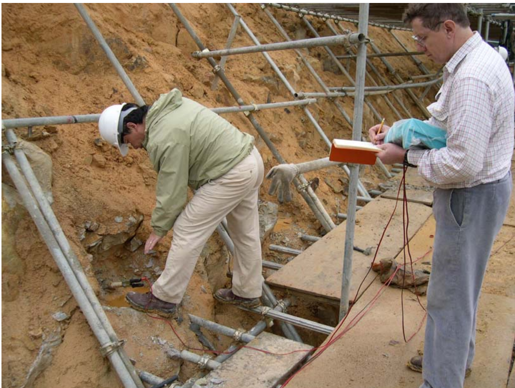
Plate 5 - Measurement of Electrical Resistance at a Working Nail
