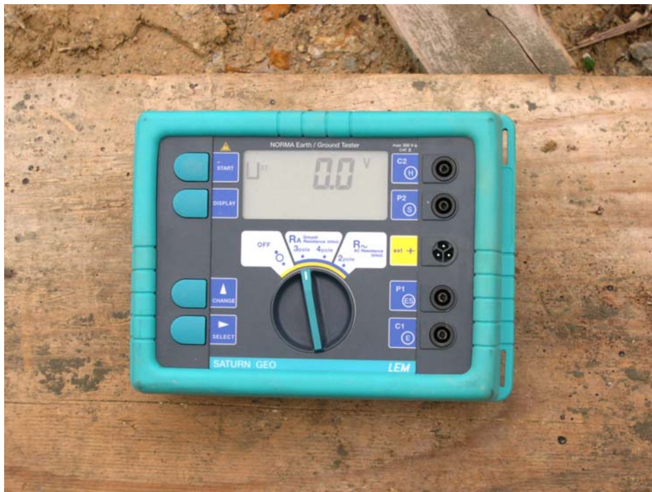
Plate 4 - Instrument Used in the 3-pole AC Electrical Resistance Method
