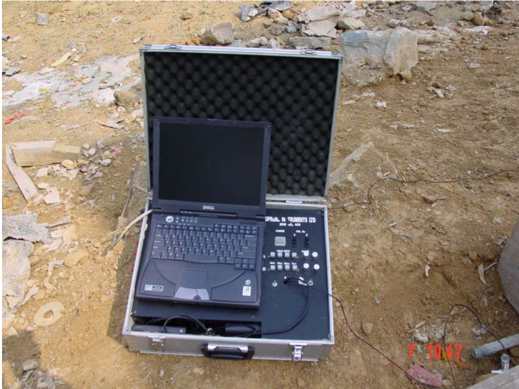
Plate 3 - Instrument Used in Surface Wave Time Domain Reflectometry
