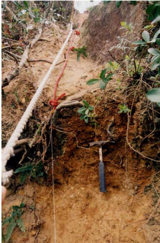
Plate 7 - View of a Minor Scarp (0.5 m in Height) Immediately above the Main Scarp Along Surface Strip SS1 (Photograph taken on 11 March 2003)
