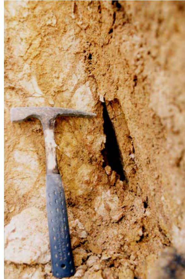
Plate 14 - Close-up View of Deformed Rock Mass with Voids and Kaolin Coated Joint Surfaces (Photograph taken on 18 March 2003)
