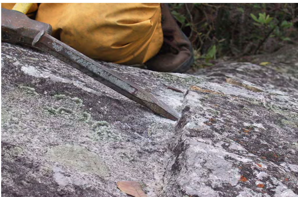
Plate 4 - Sampling a 50 mm Thick Slab of Rock From a Boulder at the Sunset Peak West Landslide Site for Surface Exposure Dating (Taken on 28.3.02)
