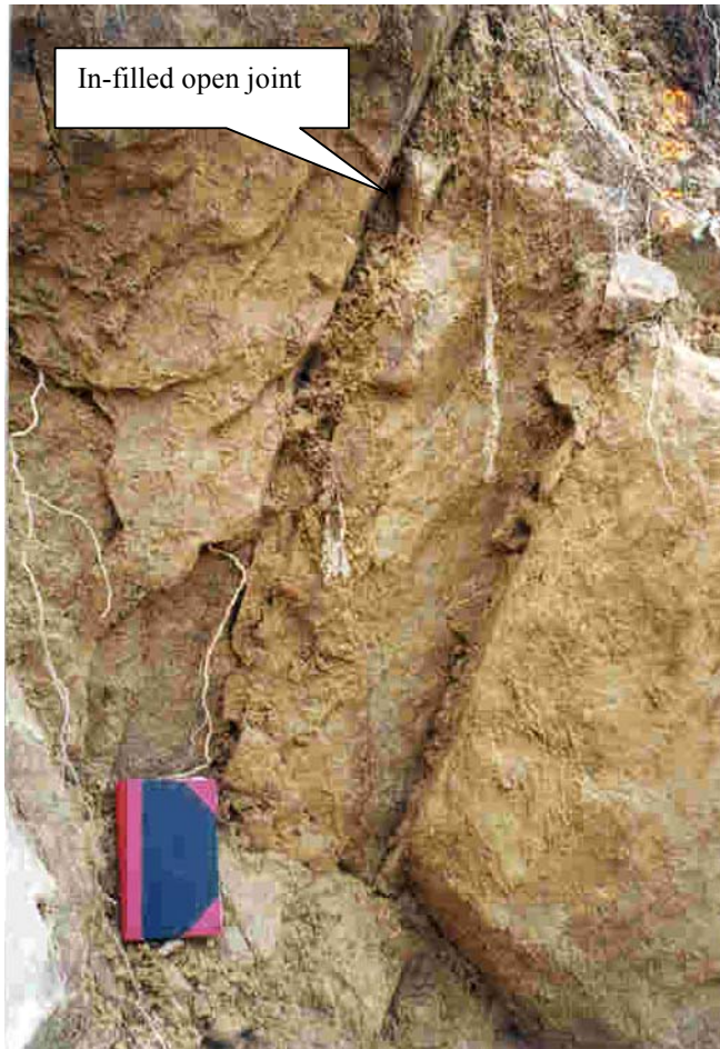
Plate 22 - Details of Open and Infilled Joints in Main Scarp of Landslide A (Photographs Taken on 31 September 1999)
