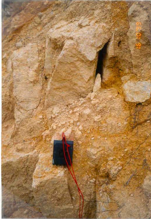
Plate 23 - Details of Open and Partially Infilled Joints in Main Scarp of Landslide A (Photographs Taken on 16 October 1999)
