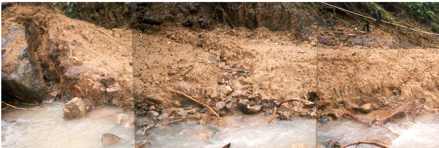
Plate 18 - Fresh, Silty Debris Overlying Old Debris (Angular Cobbles) near Site of the Kitchen Structure to House No. 38 (Photograph Taken on 25 August 1999)
