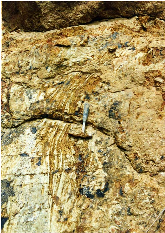
Plate 6 - Flow Banded Quartzphyric Rhyolite Exposed in Landslide Scar 4 (Plate Location Shown on Drawing EG503) (Taken on 6/8/97)
