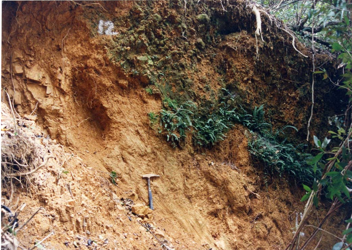
Plate 36(a) - Main Scarp Showing Vegetation Line Indicating at Least Two Phases of Movement Together with Old and Recent Slickensides on the Scarp Surface and a Rhyolite Dyke Contact (Plate Location Shown on Drawing EG503) (Taken on 26/9/97)
