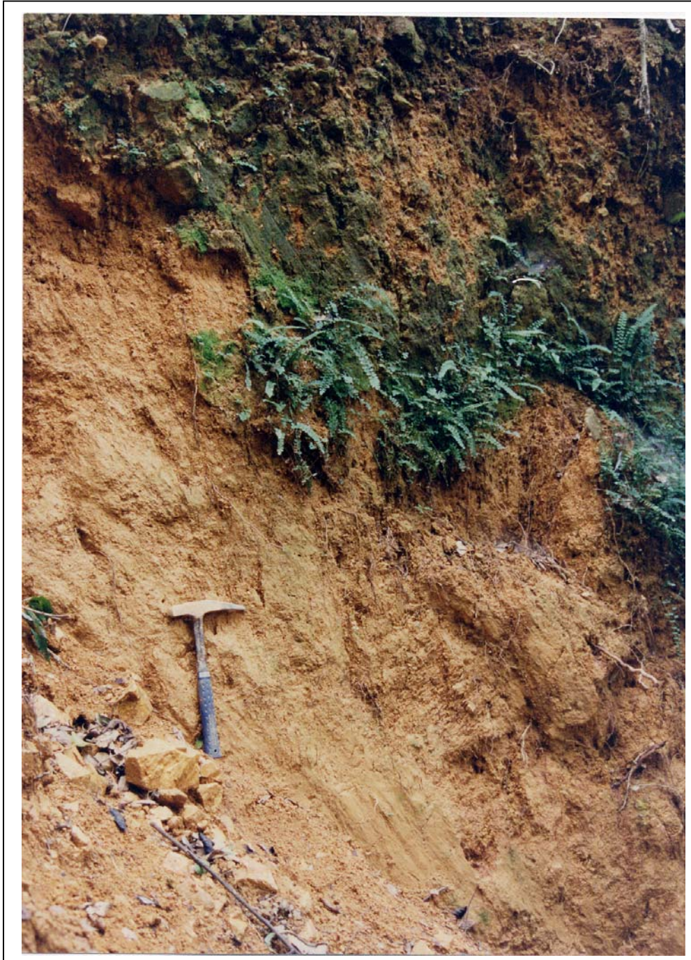
Frontispiece: The Main Scarp of the Composite Landslide with Two Generations of Slickensides and a Distinct Vegetation Line of Ferns and Moss Indicating at Least Two Phases of Landslide Development
