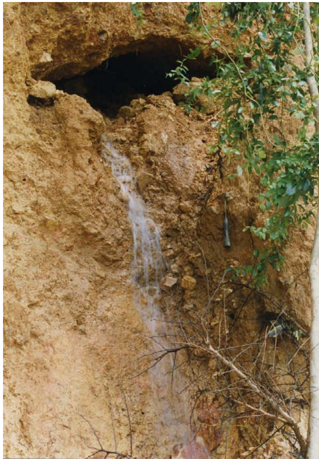
Plate 28(b) - Soil Pipe with Medium Flow (Plate Location Shown on Drawing EG503) (Taken on 8/8/97) GS 97/107C/30
