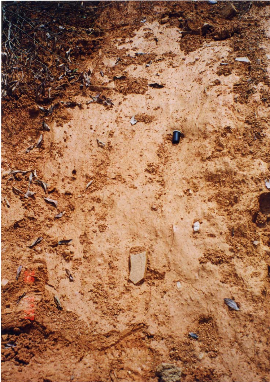
Plate 12 - Planar Slickensided Surface of Rupture Exposed below the Crown of Landslide Scar 1 (Plate Location Shown on Drawing EG503) (Taken on 30/7/97)
