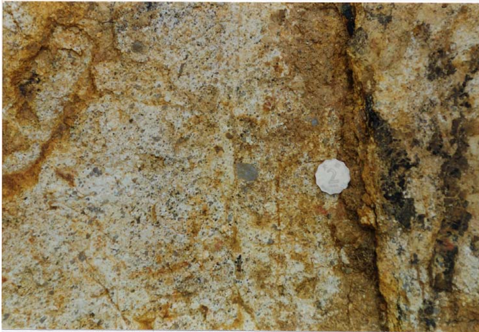
Plate 5 - Lapilli-Bearing Coarse Ash Crystal Tuff (Plate Location Shown on Drawing EG503) (Taken on 7/7/97)
