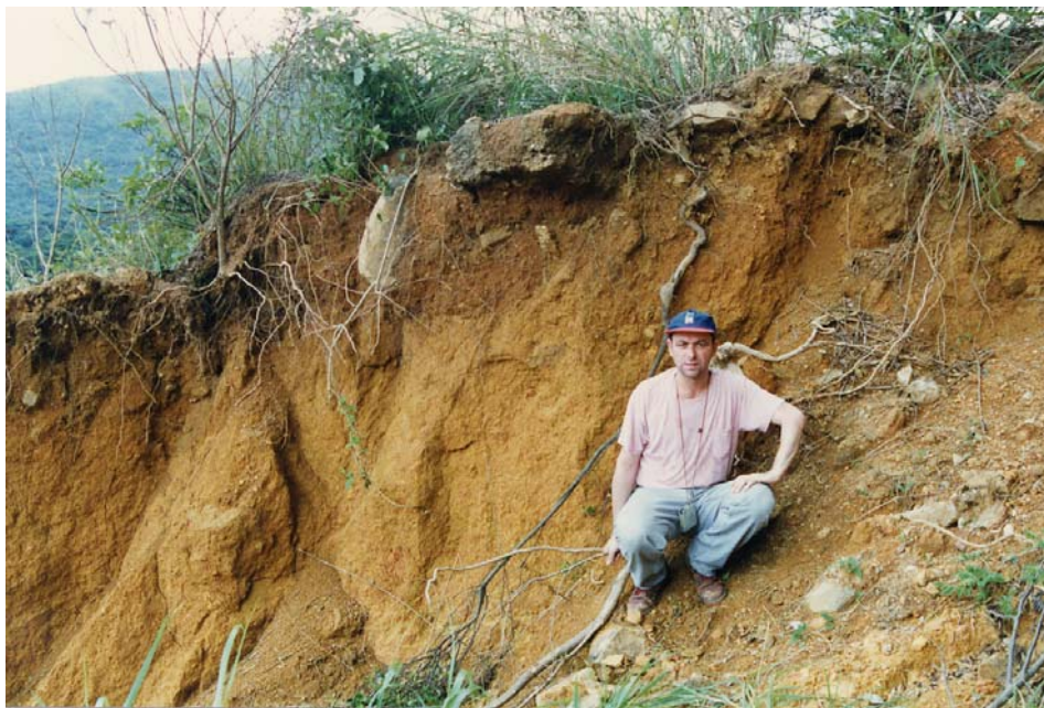
Plate 16 - Made Ground Exposed in the Main Scarp of Landslide Scar 2 (Plate Location Shown on Drawing EG503) (Taken on 7/8/97) GS 97/93C/14
