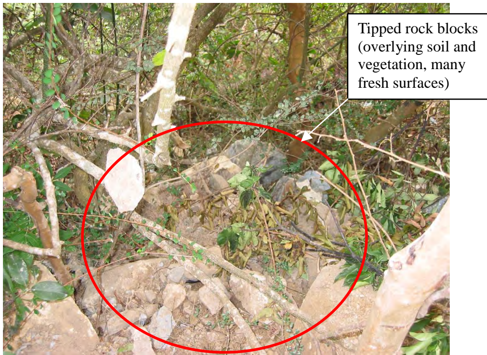
Plate 8 - Tipped Rock Blocks on the Hillside below the Catchwater (Photograph taken on 5 December 2002)
