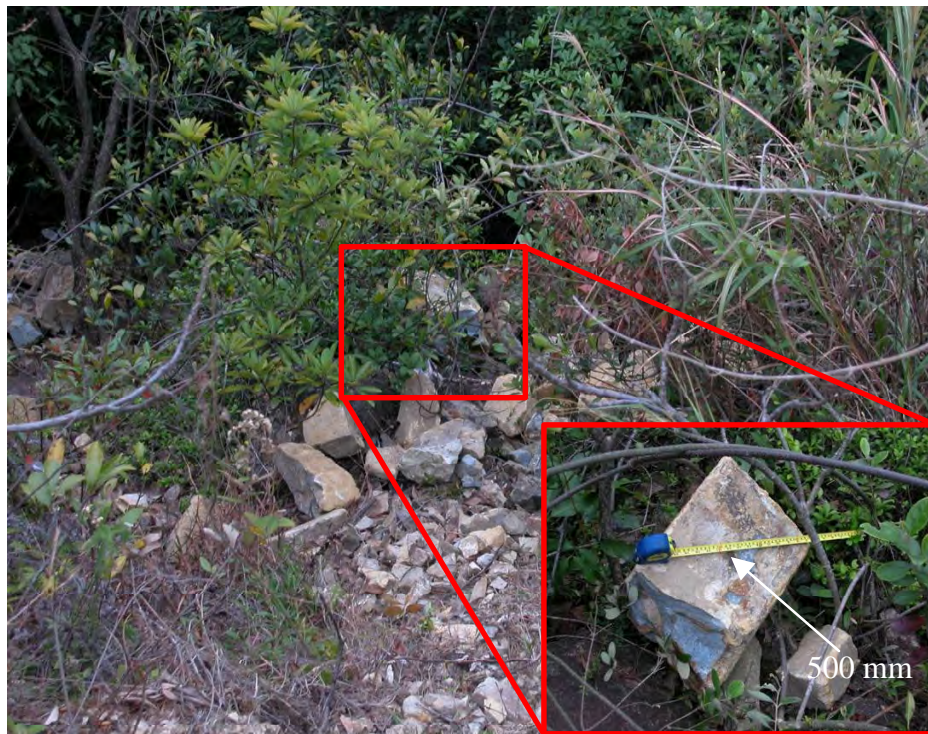
Plate 9 - Tipped Rock Blocks up to 0.5 m across below the Catchwater (Photograph taken on 14 February 2003)
