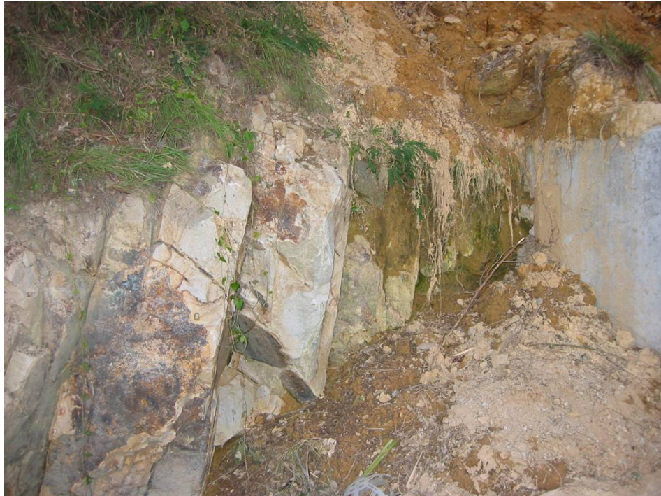
Plate 3 - Moderately Decomposed Tuff to the North of the Toe of the Landslide (Photograph taken on 16 August 2002)
