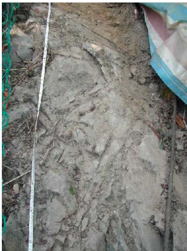
Plate 27 - Moderately Decomposed Tuff Exposed in Slope Strip No. SS2 between 1.4 m and 6.6 m (Photograph taken on 5 September 2002)
