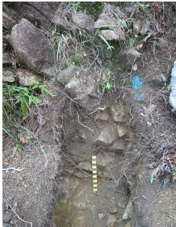
Plate 9 - Inspection Trench Across Curved Lineament Showing Exposed Rock on Side and Base of Trench (Photograph taken on 17 June 2002 by HCL)
