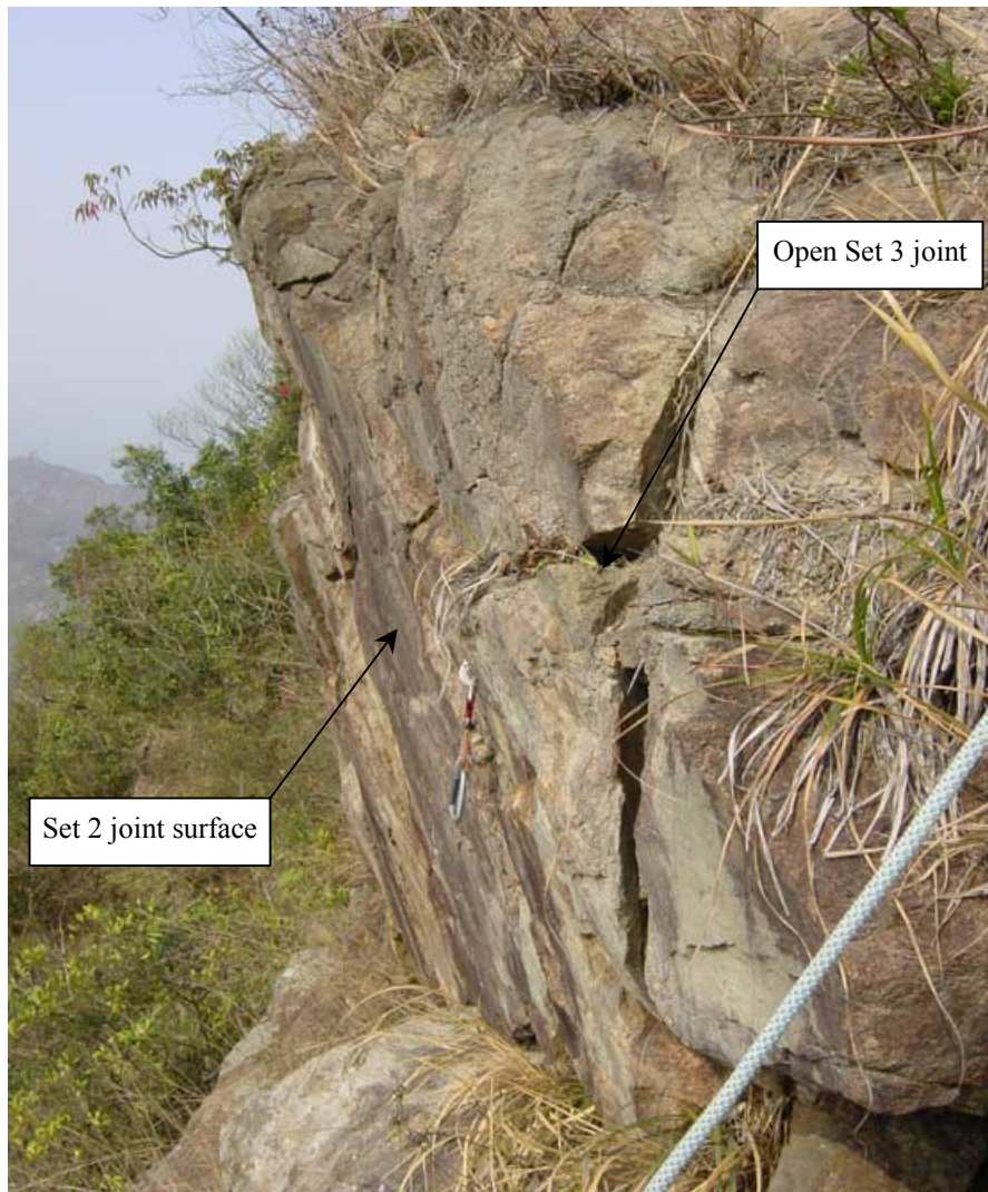
Plate 26 - Dilated Joints in Rock Face above Source Area (Photograph taken on 4 January 2002)
