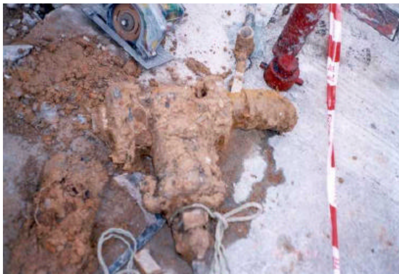
Plate 5 - Corroded Watermain and Stop-valve Removed (Photograph taken on 14 December 2001 by WSD)
