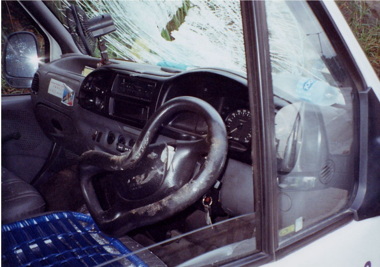
Plate 1 - View of Damage to Windscreen and Steering Wheel Caused by Falling Rock Fragment (GEO Incident No. MW2001/06/007) (Photograph taken by Police on 9 June 2001)
