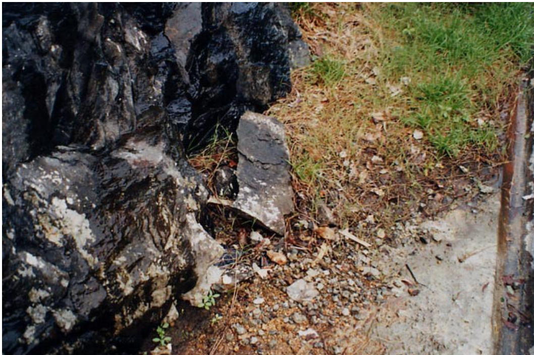
Plate 24 - View of Rock Debris and Seepage at Toe near the Middle of the Exposed Rock Portion of Slope No. 11NW-A/C58 (Photograph taken on 14 August 2001)
