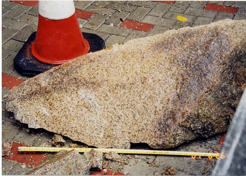
Plate 8 - Close View of Detached Rock Block Showing Clean Joint Surfaces Free of Staining and/or Infill Material. (Photograph Taken on 26 June 2001)
