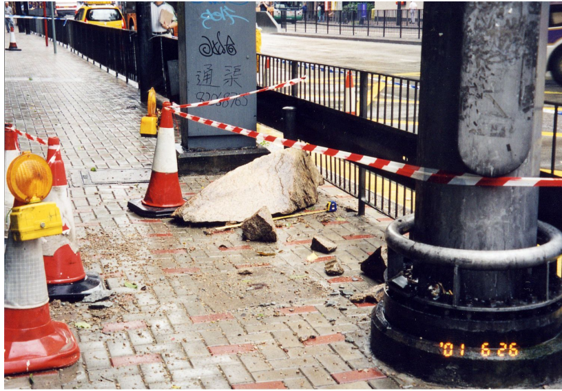
Plate 6 - View South along King's Road Footway Showing Detached Rock Block and Associated Fragments. Note Wedge-shaped Geometry of Block. (Photograph Taken on 26 June 2001)
