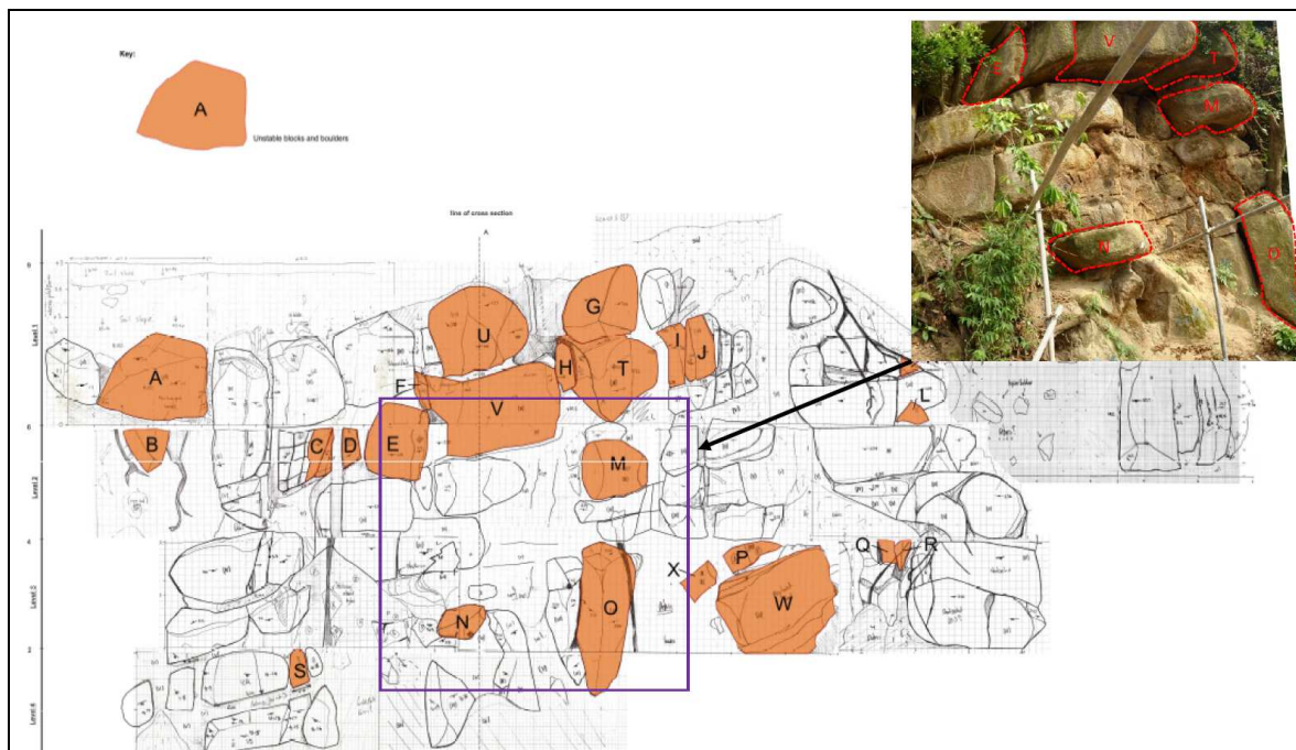
Figure D.5.4 Identification of Potentially Unstable Corestones (FSWJV, 2012a)
