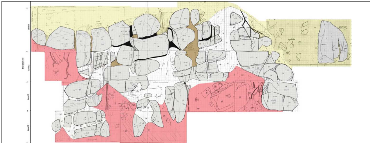
Figure D.5.3 Engineering Geological Map of Corestone Complex (FSWJV, 2012a)
