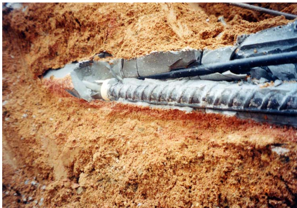
Plate 1 - Inadequate Grout Cover Revealed at a Re-development Site on Hong Kong Island
