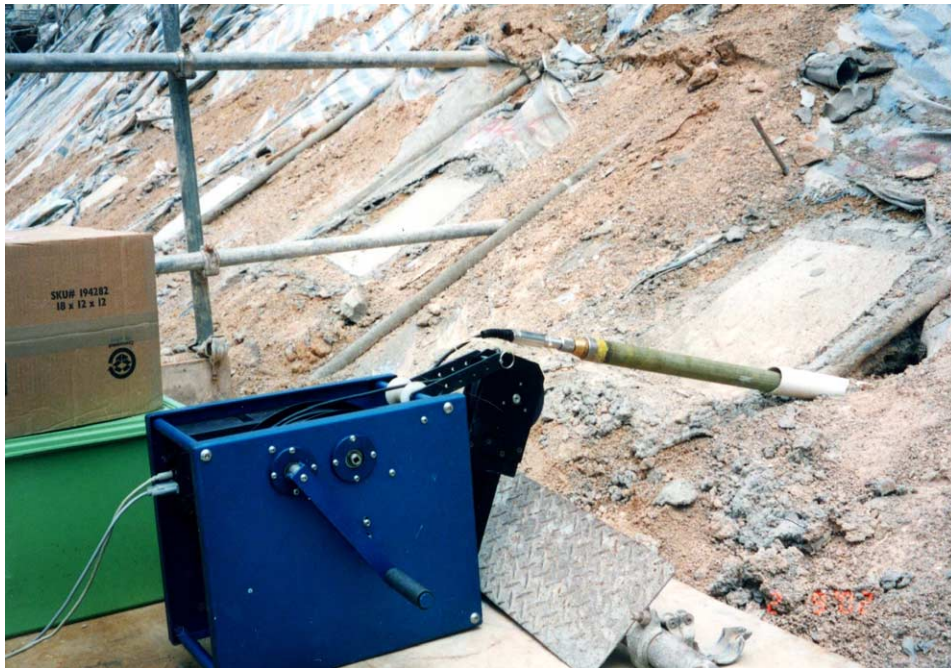
Plate 8 - Inserting the Magnetometer into a Drillhole in the Vicinity of the Test Nail
