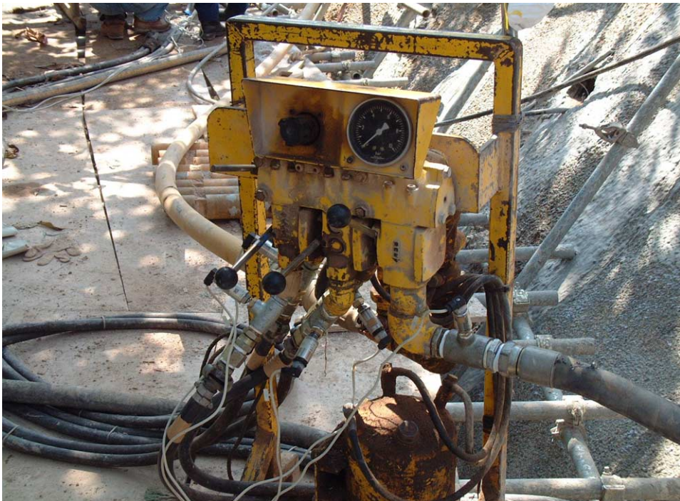
Plate 4 - Drilling Control and Operation Panel with DPM Pressure Sensors
