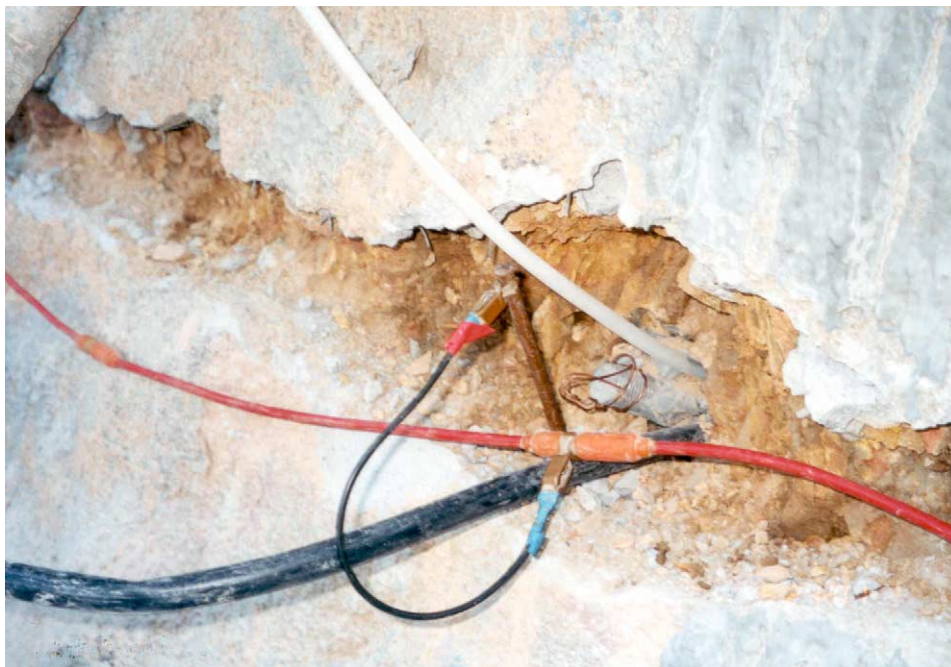
Plate 6 - One of the Electrodes Implanted in the Vicinity of the Installed Soil Nail
