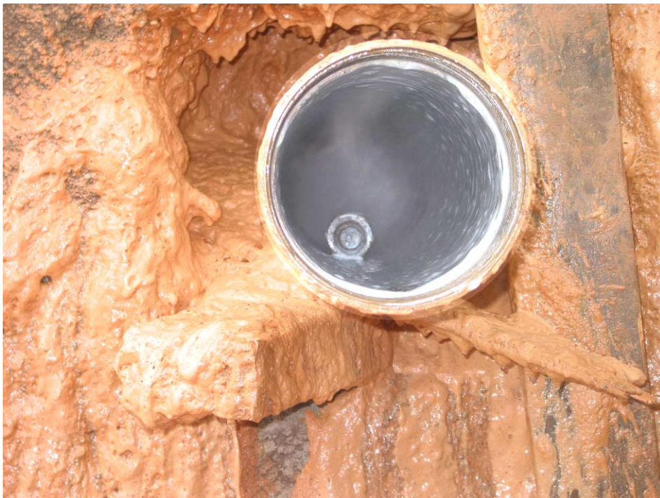
Plate 16 - A Steel Soil Nail Remained in the Casing after Over-coring
