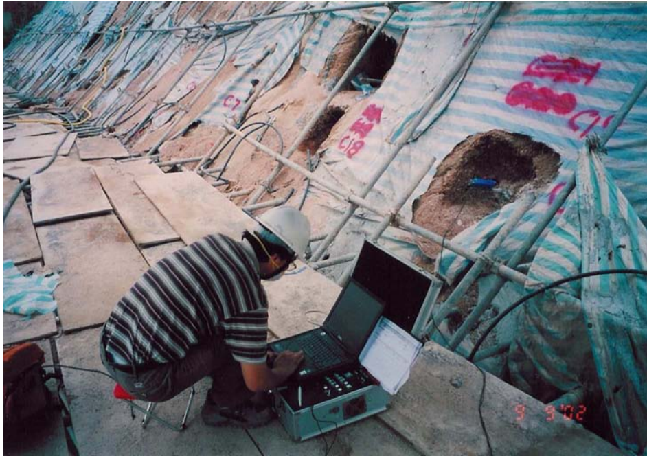
Plate 13 - Set Up of the TDR Instrument
