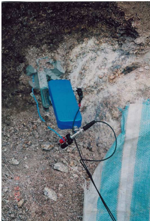
Plate 12 - Connection Details of a Pulse Emitter and Receiver at a Nail Bar Head
