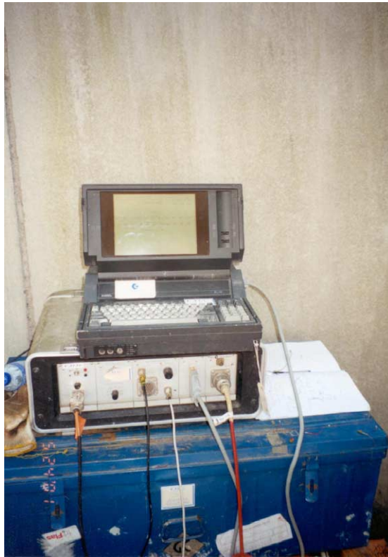
Plate 7 - Set Up of the Test Using the Mise-a-la-Masse Method
