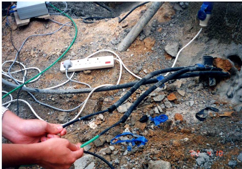
Plate 10 - Inserting the Probes into Two Pre-installed Plastic Tubes
