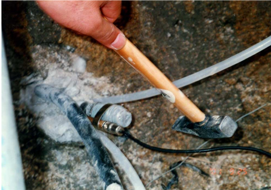
Plate 5 - Striking the Steel Soil Nail by a Light Hammer
