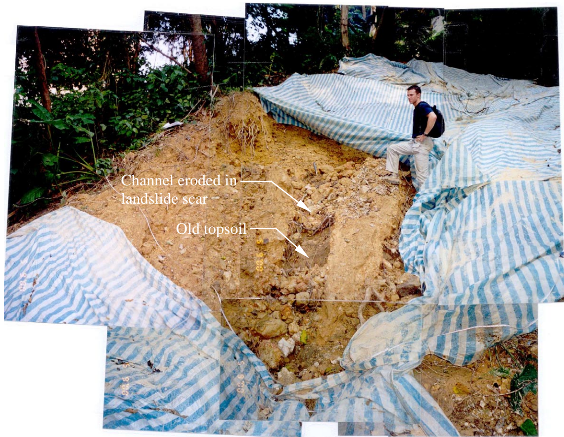
Plate 7 - View Southeast up Landslide Scar Showing Fill Material Exposed in Scar and Old Topsoil Horizon Exposed in Scoured Channel (Photograph Taken on 9 September 2000)
