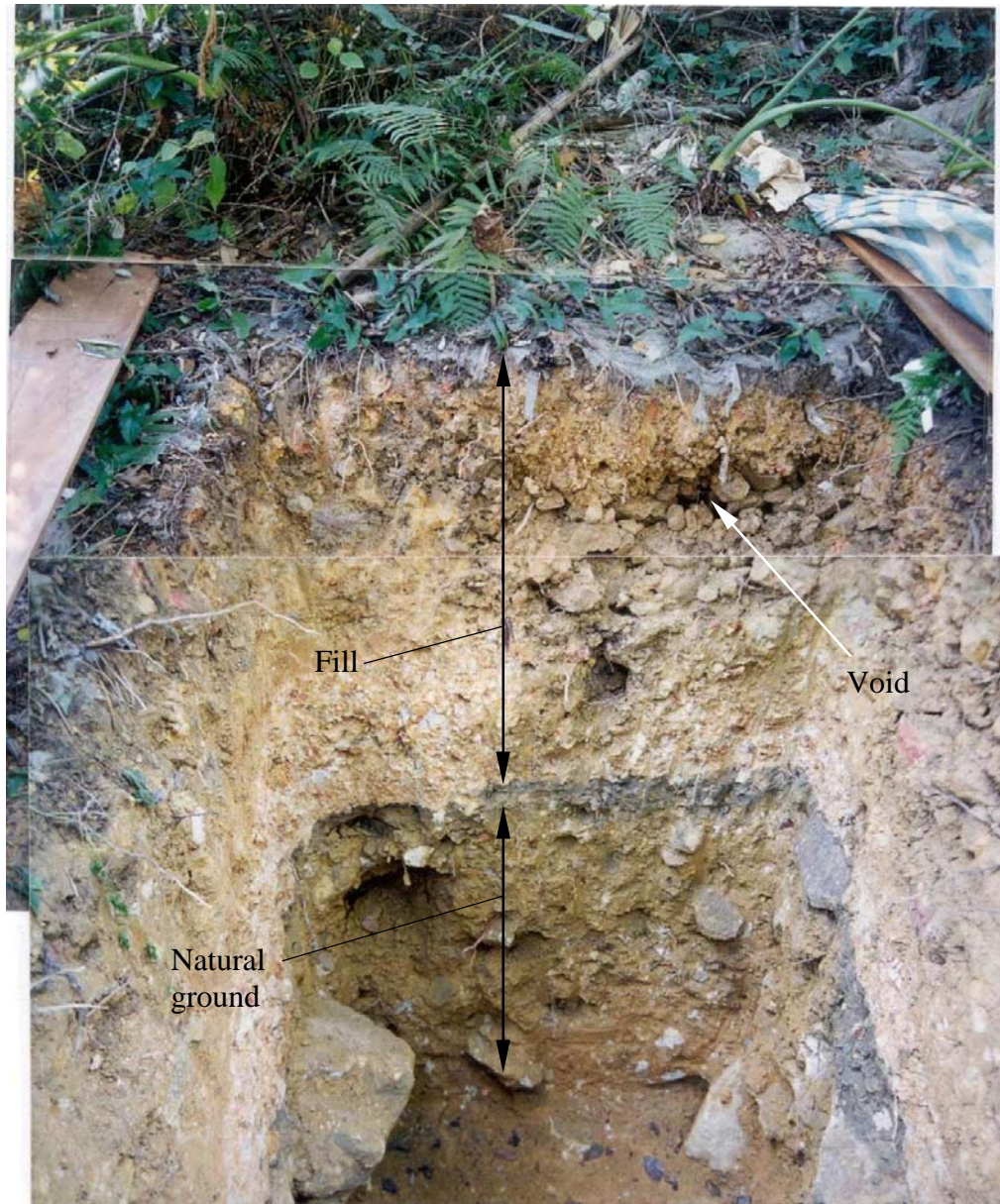
Plate 14 - Southwestern Face of Trial Pit TP5 Showing Voids in Fill (Photograph Taken on 5 March 2001)
