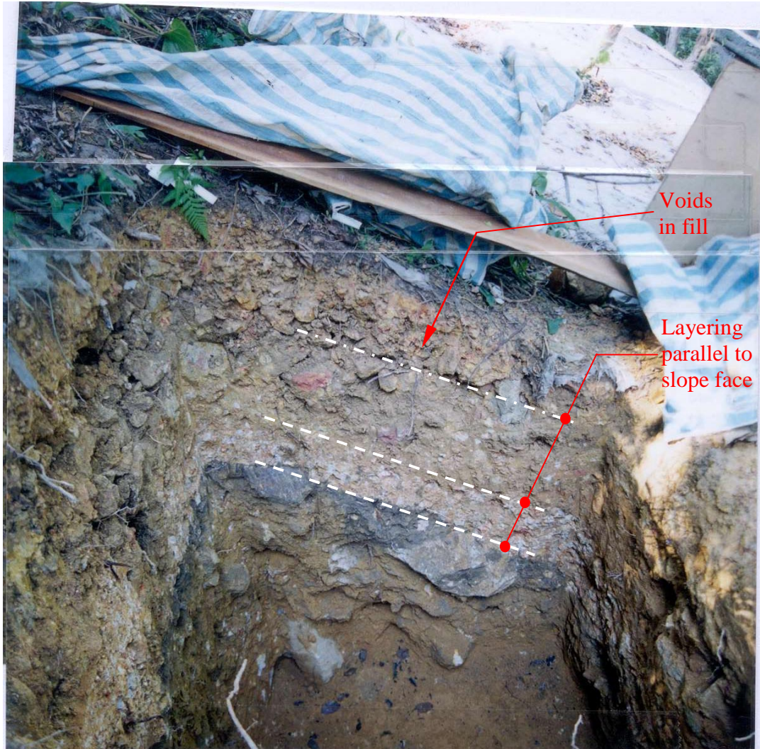
Plate 13 - Southwestern Face of Trial Pit TP5 Showing Fill Material Overlying Topsoil and Colluvium/CDT (Photograph Taken on 5 March 2001. Note Layering Parallel to Slope Face, and Voiding of Fill Indicated. Shotcreted Landslide Scar Visible at Top of Frame)
