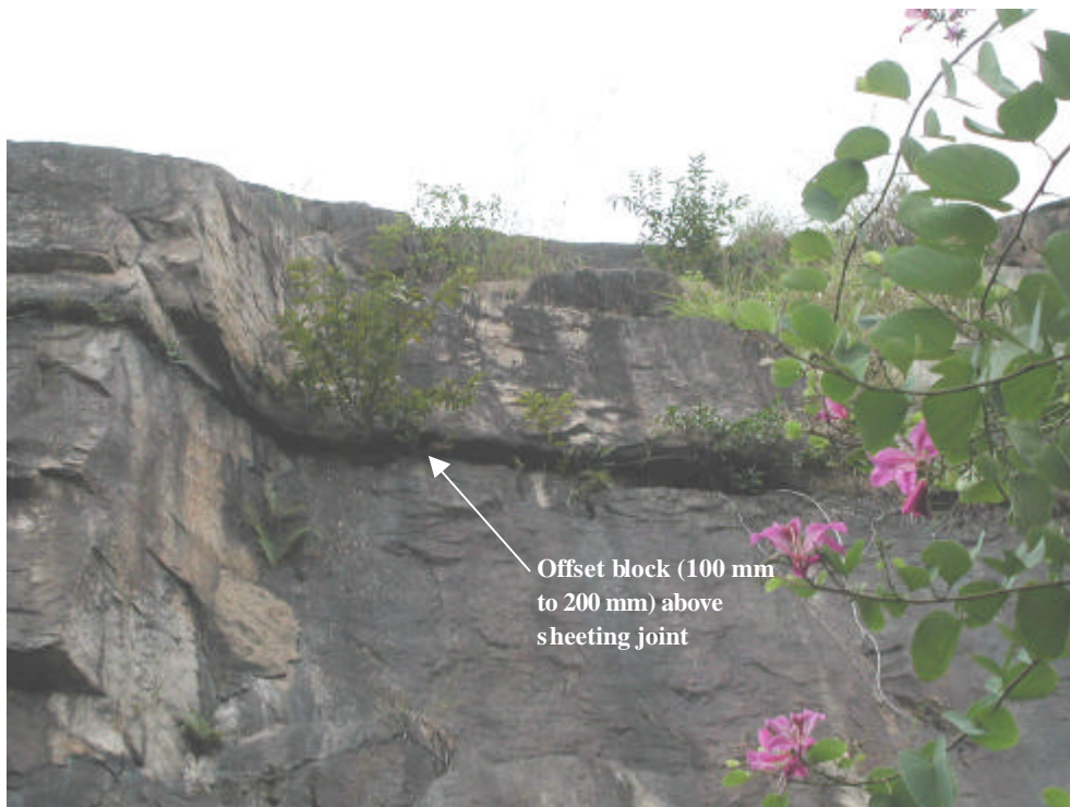
Plate 14 - Detailed View of Offset Block above a Sheeting Joint at Chainage 150 (Photograph Taken on 15 December 2000)
